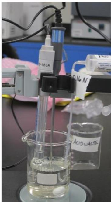
**Figure 41.** Image of titration set-up with digital titrator, stir bar, pH meter and temperature probe. Ensure nothing is touching the sides and bottom of the beaker or the stir bar
