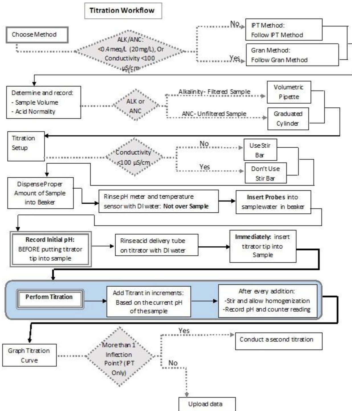
Figure 38. High Level titration workflow.
