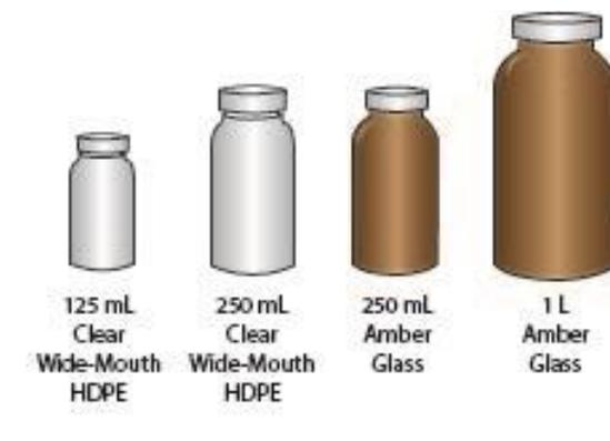
Figure 5. Water chemistry bottle types.
