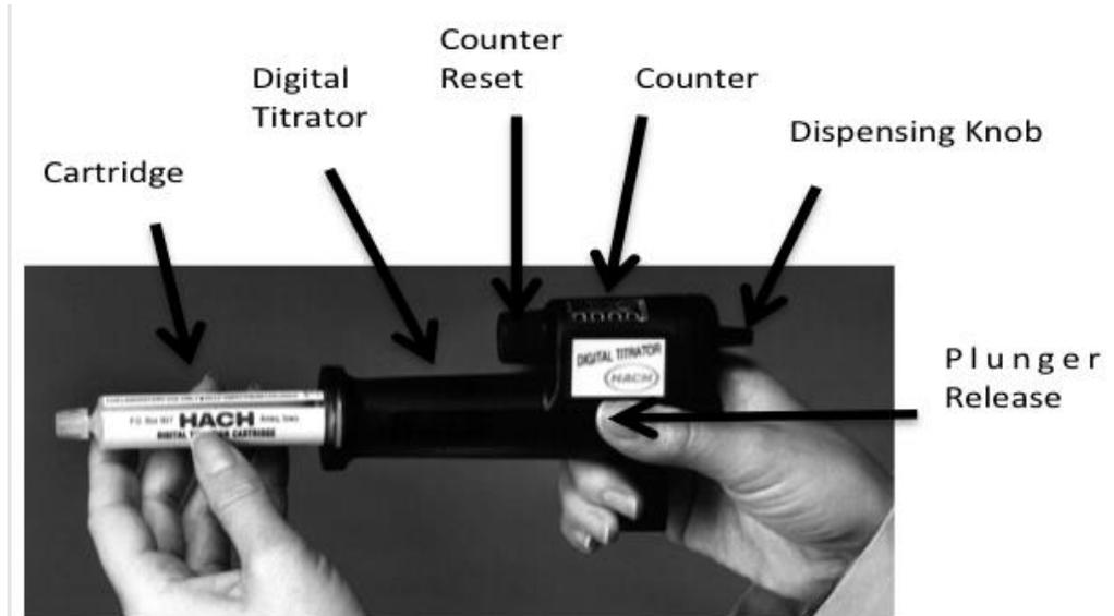
**Figure 39.** Inserting titrant cartridge into digital titrator. Photo from the Hach Digital titrator manual.
