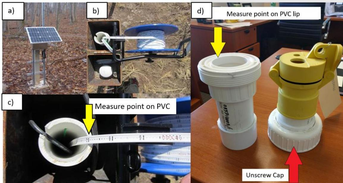
**Figure 18.** Groundwater well depth measurements (a) Standard groundwater well at a NEON site (b) Water-level tape attached to outer well casing. (c) Reading the depth to water from the water-level tape on standard well. The tapes are marked in “meters” with each foot increment marked in red. Readings are taken at the top of the inner PVC casing. (d) Cap disconnection and measurement point for wells with snorkel cap design.
