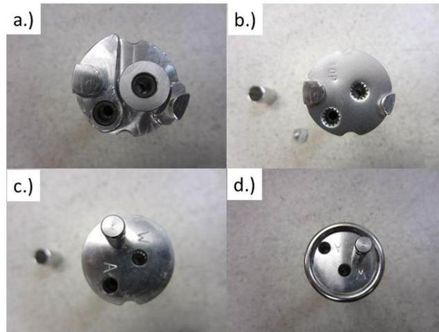
**Figure 19.** Assembly of the fitting plate at the top of the pump for holding the air and water lines. (a) Bare top of pump. (b) Fitting/grab plate added (“TOP” must face upwards). (c) Top plate added. (d) Collar added to lock parts (a-c) together.
