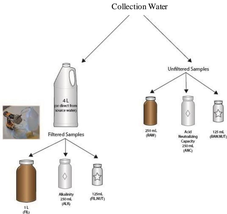
**Figure 6.** Flowchart of Water Chemistry Sample Collection and Filtration. à Indicates 250 mL, wide-mouth sample bottles that remain at the Domain Support Facility for titration analysis. ☆ Indicates 250 mL, wide-mouth sample bottles that are frozen (-20°C) immediately prior to shipping. ANC is only collected monthly. Letters in parenthesis indicate the sample type that correspond to the chemistry labels (see Figure 8).
