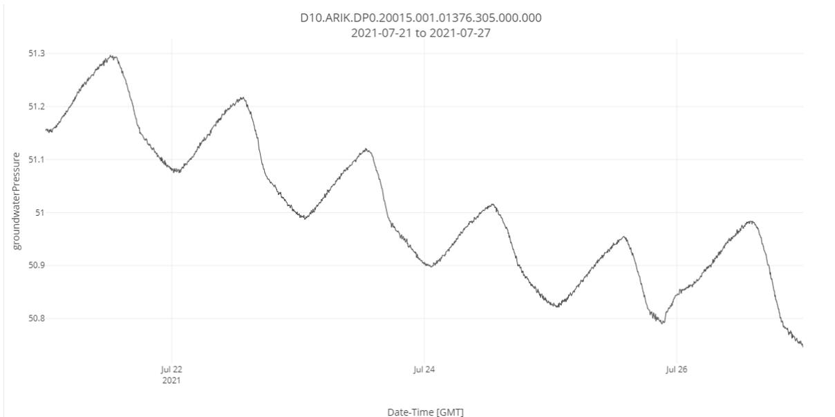
**Figure 15.** DQ Blizzard plot for groundwater pressure for an individual well over a 1-week period. Pressure is roughly 51 kPa indicating that there is about 5.1 m of water above the sensor. If the sensor is 0.5m from the well bottom, then the water column height is roughly 5.6m.
