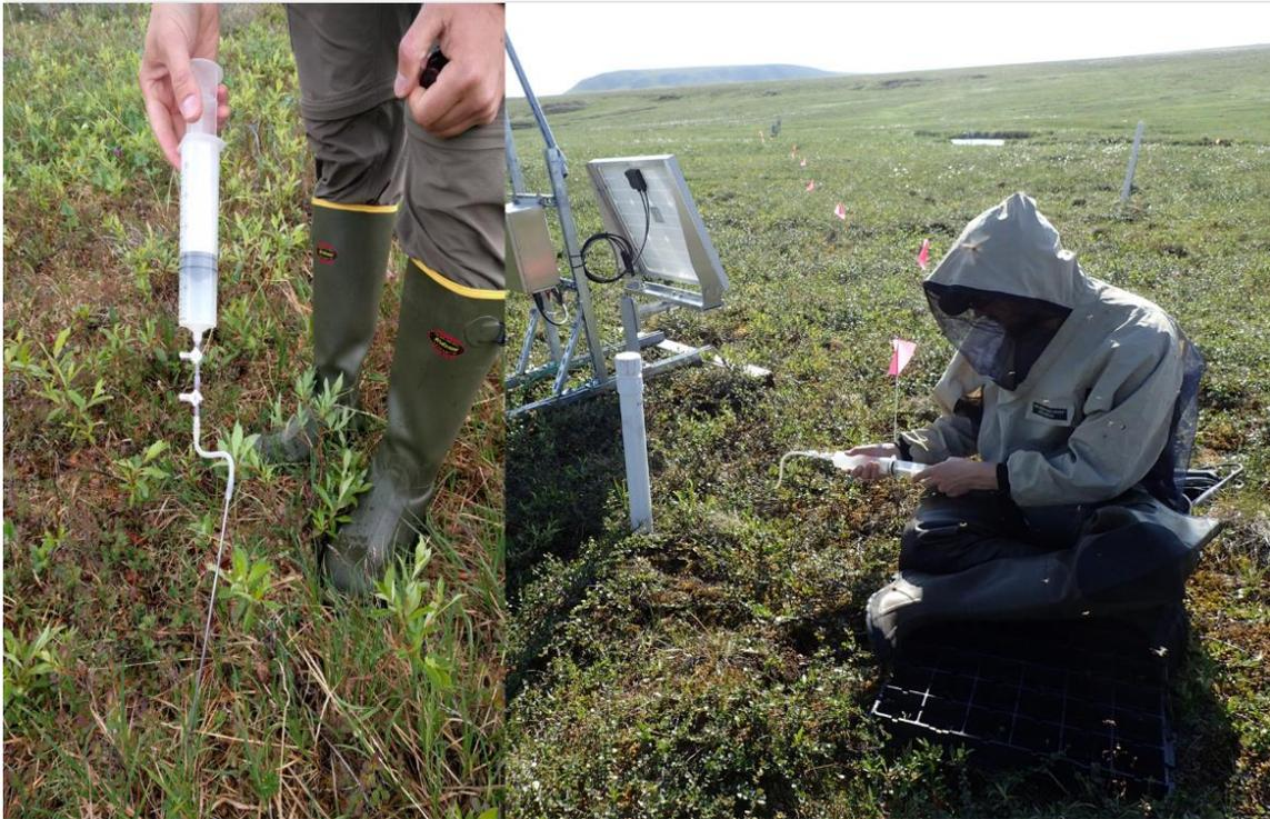
Figure 30. Sampling needle and syringe setup.
