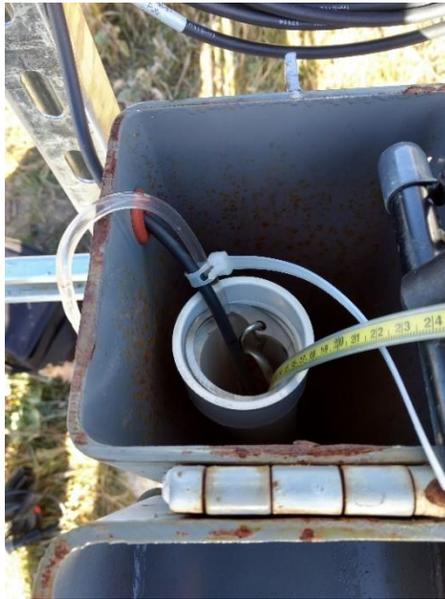
Figure 28. Pump tubing secured in place with zip tie.
