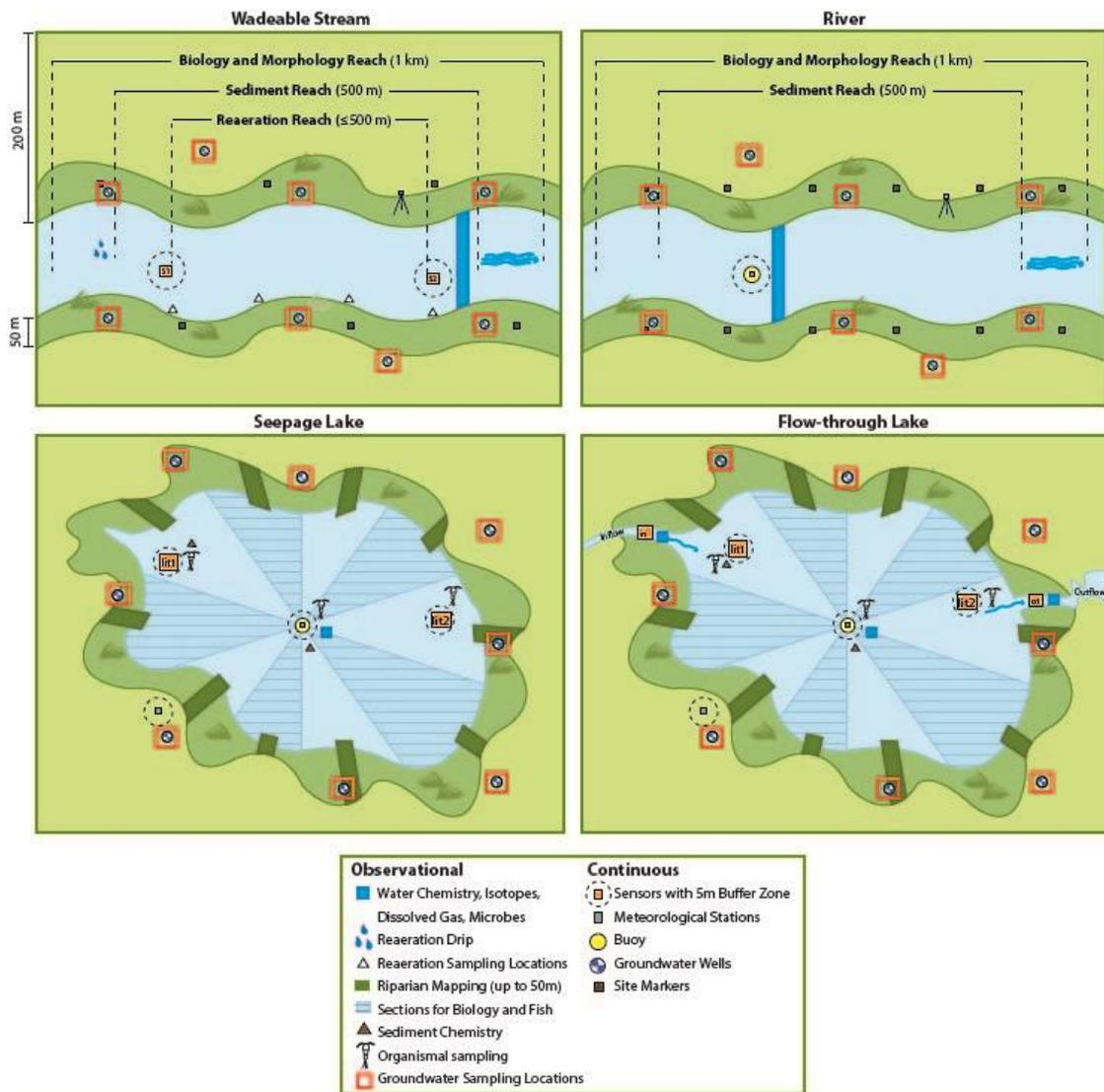
**Figure 1.** Generic site layouts for wadeable streams, rivers, and lakes surface water and groundwater sampling locations. Seepage lakes are lakes with no true inflow and outflow, while flow-through lakes have a true inflow and outflow.
