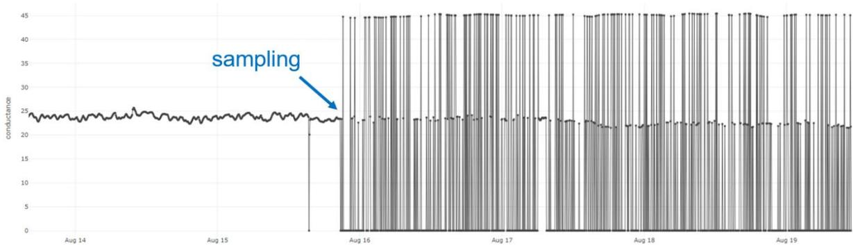
**Figure 44.** Example of noisy LO conductivity data after a sampling event.
