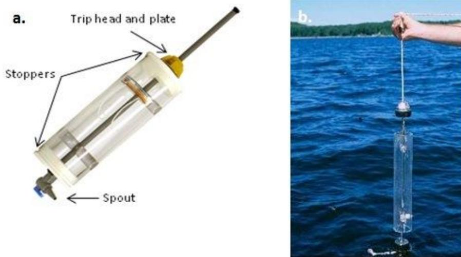
**Figure 13.** Illustration of Kemmerer sampler for water sampling (a). Illustration of how the Kemmerer is lowered into the water by holding the rope and messenger (b)
