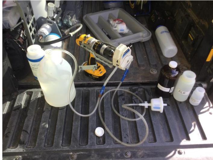
**Figure 35.** Pump and filter setup, including a peristaltic sampling pump (modified from Woessner 2007), a 4 L sample bottle, tubing connectors to connect peristaltic and C-flex tubing, and a capsule filter.
