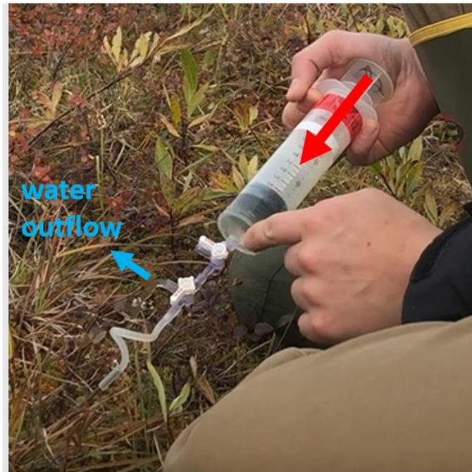
**Figure 32.** Stopcock position for expelling water during bubble-free sampling.
