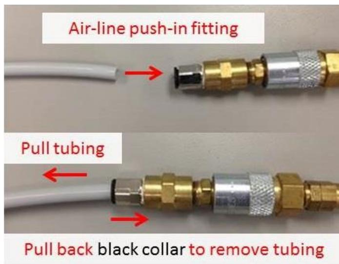
Figure 24. Attach grey air-line to blue air-line.
