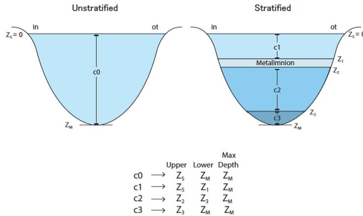
**Figure 12.** Example of an unstratified and stratified lake water column a) sampling depths with placement of the thermocline and b) identification of upper and lower section depths. In deep lakes, 2 thermal stratifications may occur, creating 3 sections. Note, hypolimnion sampling is determined by the hypolimnion section depth (i.e., thickness). If hypolimnion thickness is < 4m, collect one sample at midpoint of hypolimnion. If hypolimnion thickness is > 4 m collect an integrated sample.
