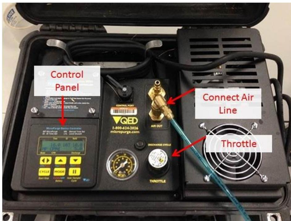
Figure 23. Attach blue air-line to controller.
