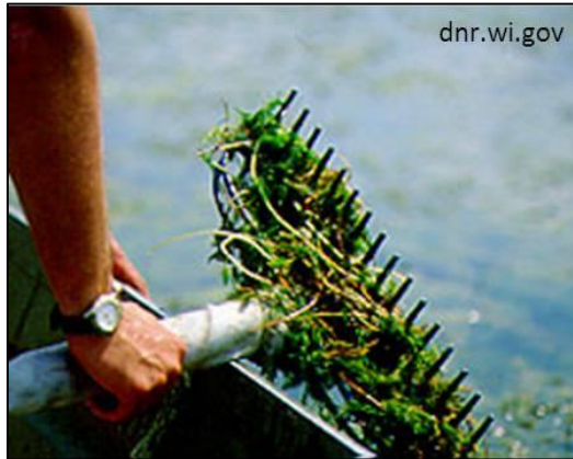
Figure 16. Double-sided rake head with plant sample being brought into the boat.
