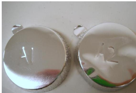
**Figure 18.** Examples of newly labeled aluminum weigh boats.
