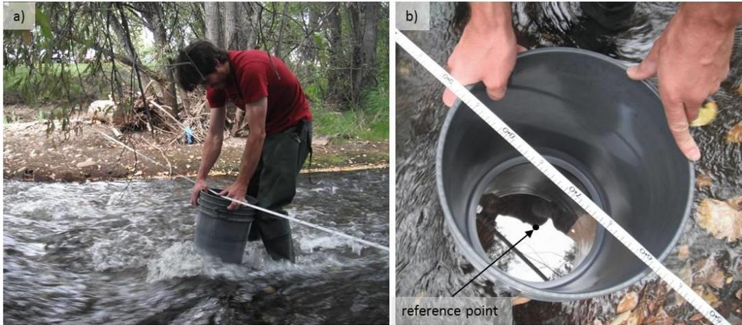
**Figure 13.** a) A field technician holds the view bucket in the water, under the meter tape transect. b) Hold the view bucket so that the reference point lines up with the point you want to sample on the meter tape.
