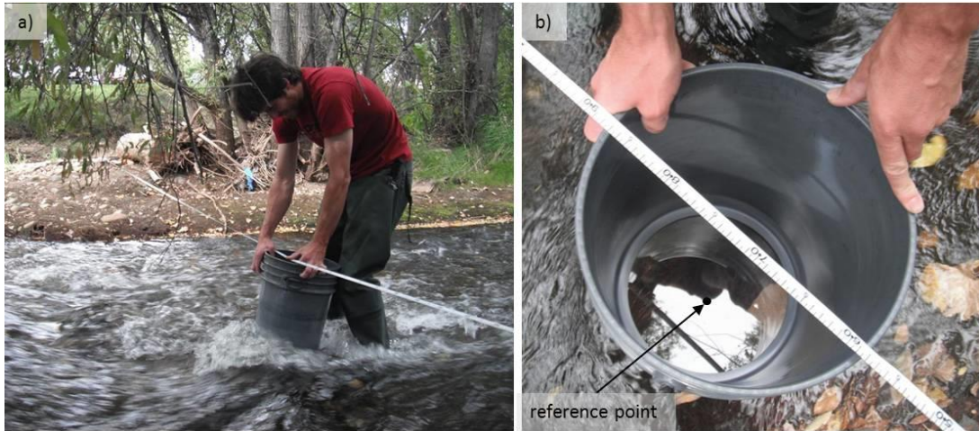
Figure 13. a) Hold the view bucket in the water, under the meter tape transect. b) Hold the view bucket so that the reference point lines up with the point you want to sample on the meter tape.
