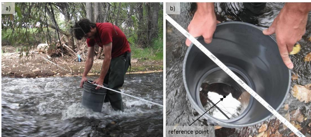
Figure 18. a) Hold the view bucket in the water, under the meter tape transect. b) Hold the view bucket so that the reference point lines up with the point you want to sample on the meter tape.
