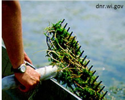
Figure 17. Double-sided rake head with plant sample being brought into the boat.
