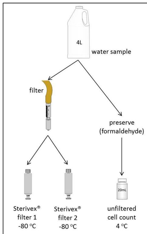
**Figure 6.** Schematic for surface water sample partitioning
