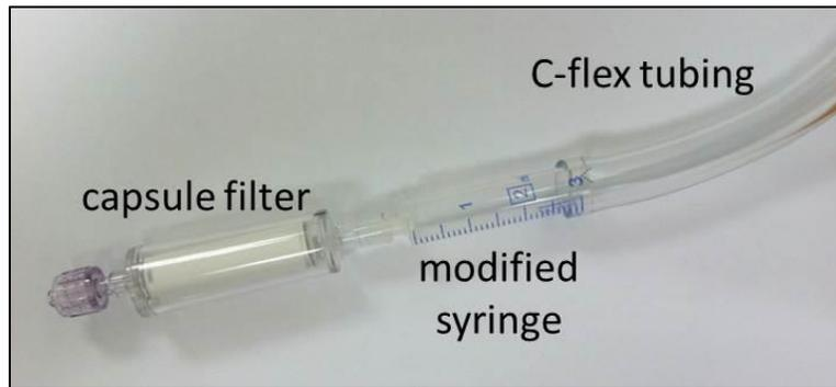
Figure 2. Filter adapter for peristaltic pump
