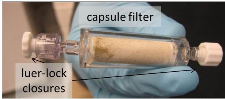
**Figure 8.** Capsule (Sterivex®) filter and luer lock closures
