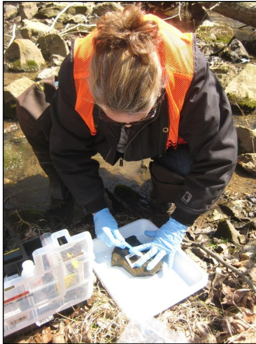
Figure 10. Template placement for epilithic microbe sampling protocol. Note sterile organizer used to hold equipment on the stream bank.
