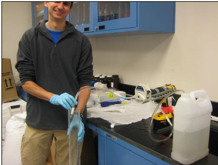
Figure 7. A field technician demonstrates pumping sample water out of the 4 gallon HDPE jug, through the peristaltic pump, the through the Sterivex® filter, and into a graduated cylinder to measure the volume filtered.
