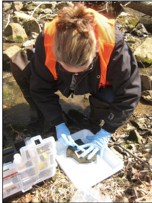
Figure 11. Template placement for epilithic microbe sampling protocol. Note sterile organizer used to hold equipment on the stream bank.
