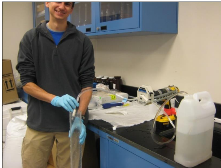
Figure 9. Pump sample water out of the 4 gallon HDPE jug, through the peristaltic pump, the through the Sterivex® filter, and into a graduated cylinder to measure the volume filtered.
