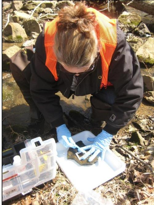
**Figure 15.** Template placement for epilithic microbe sampling protocol. Note sterile organizer used to hold equipment on the stream bank.
