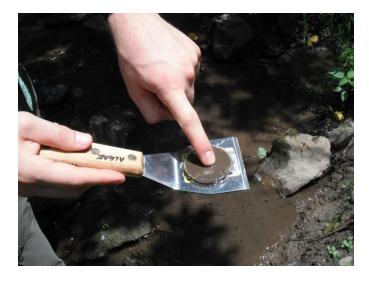
**Figure 23.** An epipelon sample collected with the Petri dish lid and metal spatula.
