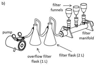
Figure 30. Filter apparatus setup: a) hand pump; b) filter manifold.
