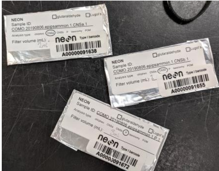
Figure 33. Example of algal chemistry packets with human readable label and barcode label.
