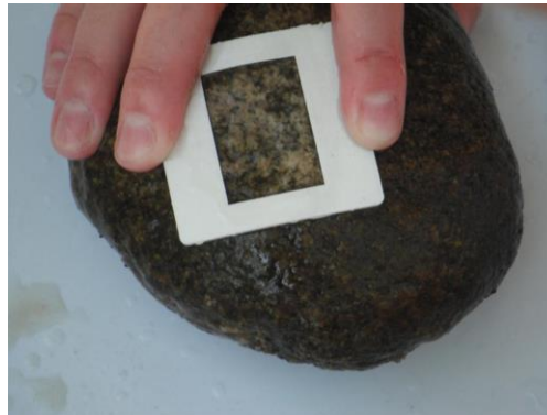
Figure 25. Template placement for epilithon protocol. (Note: Samples should not be processed in direct sunlight)
