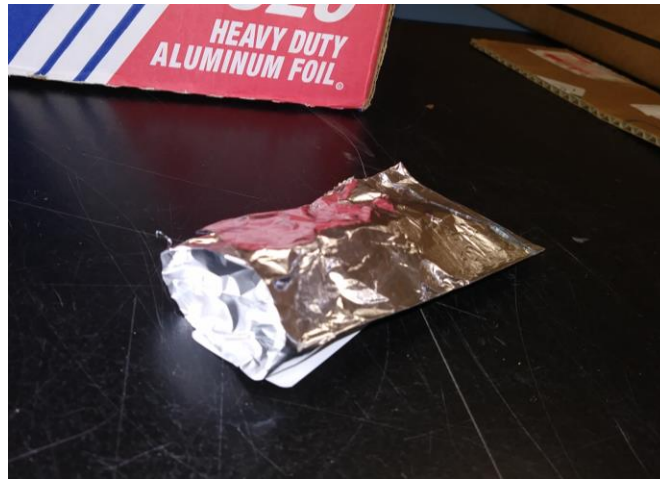
Figure 41. Example of a filter packet left slightly open for drying algal chemistry filters in the drying oven.
