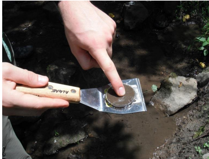
Figure 29. An epipelton sample collected with the Petri dish lid and metal spatula.
