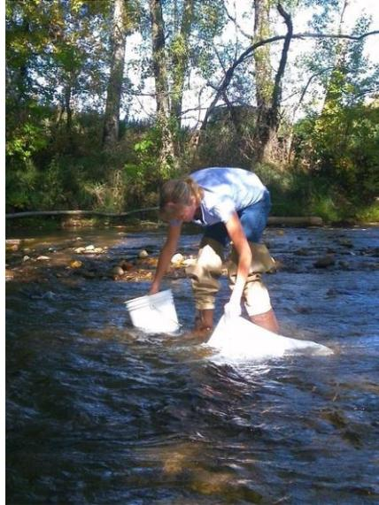
**Figure 16.** A field technician holds the Surber net on the stream bottom, and keeps the bucket nearby for depositing rocks from the base of the Surber.
