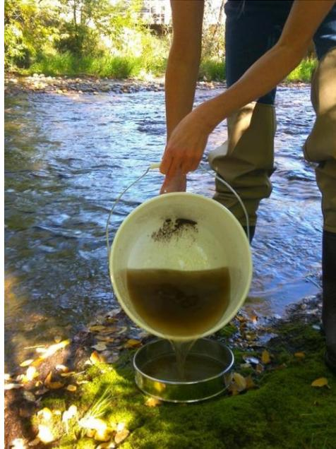
**Figure 31.** A field technician carefully pours water from the 3 gallon bucket into the sieve.
