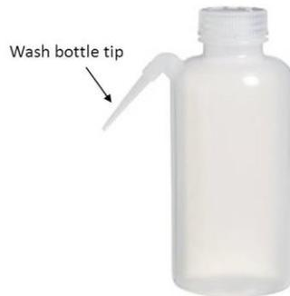
**Figure 19.** Removing the tip of the 500 mL wash bottle helps makes rinsing easier and increases water pressure. This tip pulls easily out of the main body of the wash bottle.
