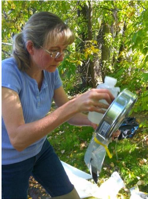
**Figure 32.** A field technician rinses the sample from the sieve into the open container with the 500 mL wash bottle.
