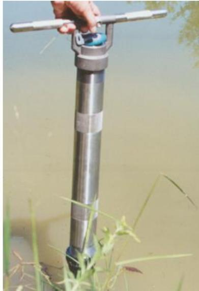
**Figure 24.** Push the hand corer through the water and into the sediments at a 90° angle
