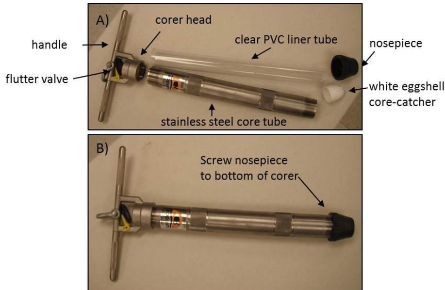
**Figure 23.** Hand-corer assembly: A) Disassembled corer. Use of the liner tube and core catcher are optional. B) Assembled corer. Note: the nosepiece may be stainless steel (not black Lexan as in photo) in some domains
