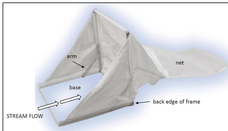
**Figure 14.** Diagram of Surber sampler set-up. The inside of the base is the sample area of the stream bottom (0.09 m<sup>2</sup>).
