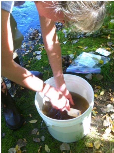
**Figure 18.** A field technician scrubs rocks from the Surber sample into the 3 gallon bucket
