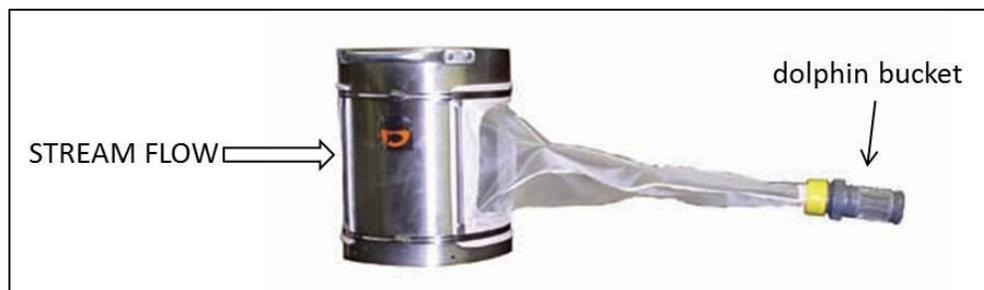
Figure 26. Hess sampler with collection net and dolphin bucket
