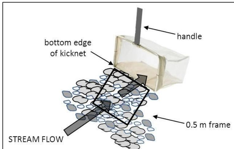
Figure 25. Example of modified kicknet setup.
