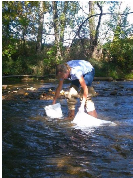
Figure 14. Hold the Surber net on the stream bottom, and keeps the bucket nearby for depositing rocks from the base of the Surber.
