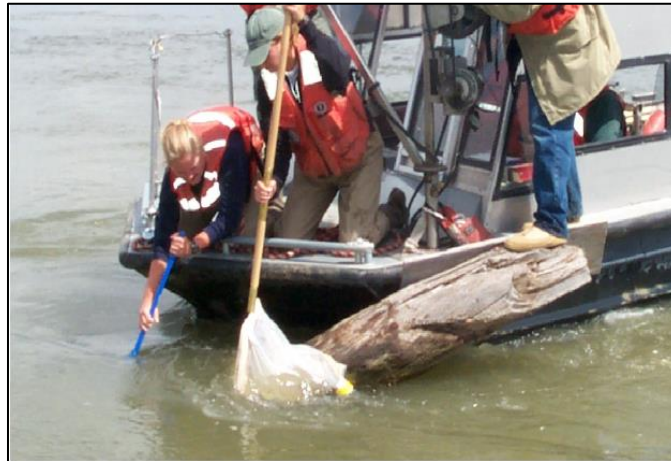
Figure 24. From Angradi et al. 2006, example of snag sampling in a large river. While the boat driver holds the boat in position, one person holds the modified kicknet against the snag, while a second scrubs the snag with a long-handled deck brush.
