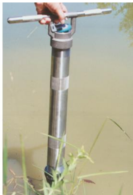
Figure 19. Push the hand corer through the water and into the sediments at a 90° angle
