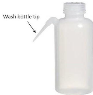
Figure 17. Removing the tip of the 500 mL wash bottle helps makes rinsing easier and increases water pressure. This tip pulls easily out of the main body of the wash bottle.
