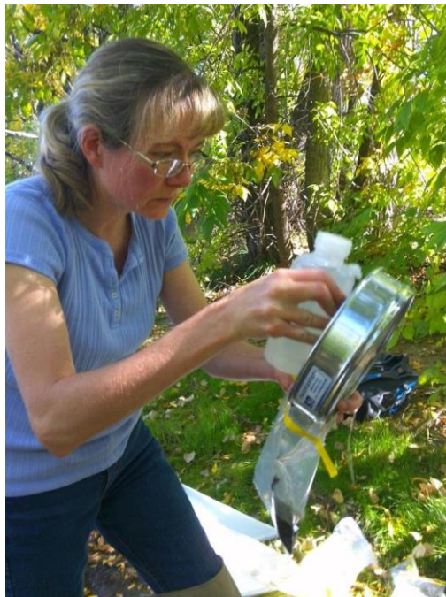
Figure 30. Rinse the sample from the sieve into the open container with the 500 mL wash bottle.
