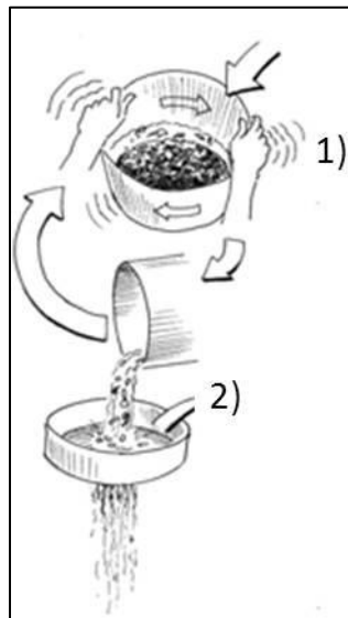
Figure 28. Process of elutriation (Dates and Byrne 1997).
