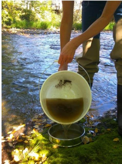
**Figure 35.** Carefully pours water from the 3 gallon bucket into the sieve.
