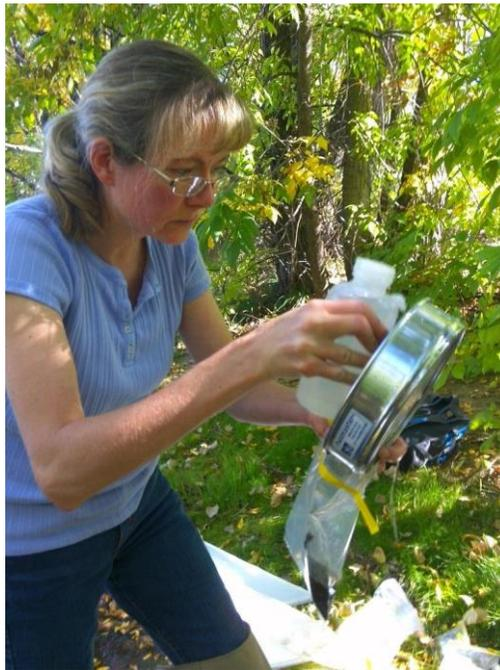
**Figure 36.** Rinse the sample from the sieve into the open container with the 500 mL wash bottle.
