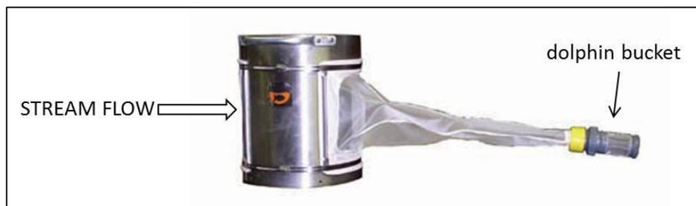
**Figure 27.** Hess sampler with collection net and dolphin bucket.
