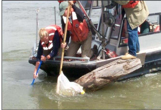
**Figure 30.** From Angradi et al. 2006, example of snag sampling in a large river. While the boat driver holds the boat in position, one person holds the modified kicknet against the snag, while a second scrubs the snag with a long-handled deck brush.
