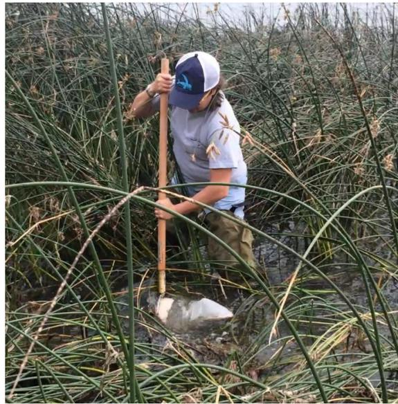
**Figure 33.** D-frame sweep technique in a littoral area; the D-frame net must remain submerged and close to the substrate throughout the entire sweep.
