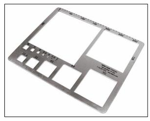
**Figure 12.** Use a gravelometer to determine which size bin/hole the particle fits through.
