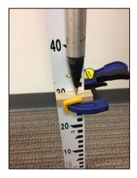
**Figure 8.** Mapping the staff gauge using a small block of wood and a clamp.
