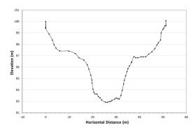
Figure 7. Example discharge cross-section survey data.
