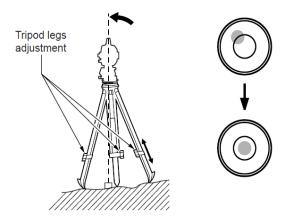
**Figure 5.** Leveling the tripod using the bubble level.
