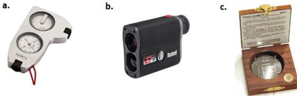
Figure 5. An example of (a) a tandem clinometer used both as a compass and for measuring angles and (b) a laser rangefinder which uses a laser beam to determine the distance to an object and a clinometer for determining height; and (c) a convex spherical densiometer used for determining % canopy cover.
