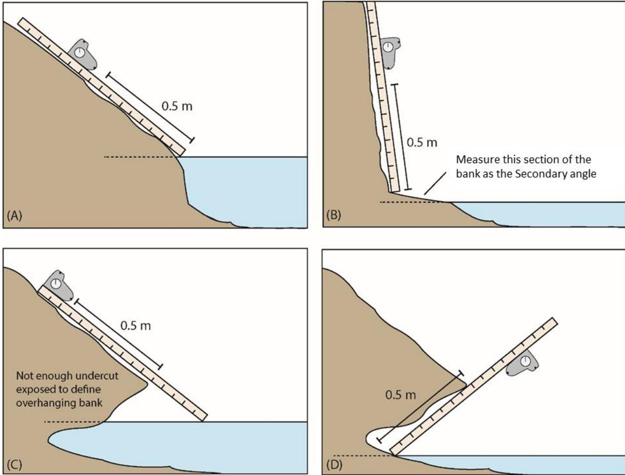
**Figure 5.** Determining shoreline bank angle for different bank types using a meter stick and clinometer. (A) Gradual shoreline (primary angle), (B) vertical bank (primary angle) incised channel (secondary angle), (C) gradual bank (primary angle) with an undercut stream bank (secondary angle), and (D) overhanging stream bank (primary angle).
