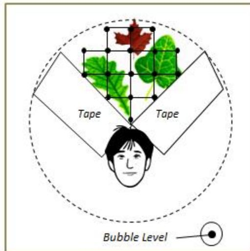
**Figure 7.** Preparing and reading a densiometer
