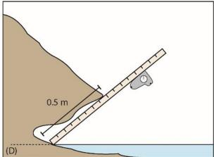
Figure 5. Determining shoreline bank angle for different bank types using a meter stick and clinometer. (A) Gradual shoreline (primary angle), (B) vertical bank (primary angle) incised channel (secondary angle), (C) gradual bank (primary angle) with an undercut stream bank (secondary angle), and (D) overhanging stream bank (primary angle).
