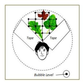
Figure 7. Preparing and reading a densiometer
