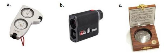
**Figure 6.** An example of (a) a tandem clinometer used both as a compass and for measuring angles and (b) a laser rangefinder which uses a laser beam to determine the distance to an object and a clinometer for determining height; and (c) a convex spherical densiometer used for determining % canopy cover.
