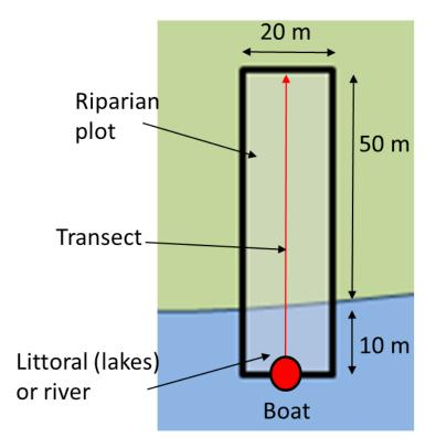
**Figure 4.** Position of the boat for riparian assessment at each lake or non-wadeable stream location. The distance to the shoreline and the approximate location and size of the riparian plot are also shown. Adjacent habitat observations are recorded from up to 15 m on either side of the plot.
