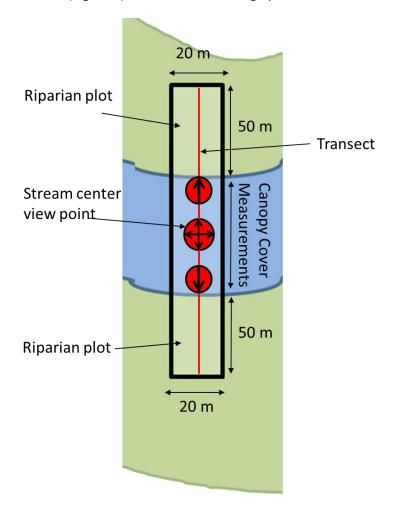
**Figure 8.** Conceptual illustration of transect and plot establishment at wadeable stream sites. Canopy cover measurements are collected at three locations within the stream. Riparian physical habitat assessment is conducted from the stream center (view point). Adjacent observations are made 15 m on either side (upstream and downstream) of the plot. (Modified from Kaufmann, 2001).
