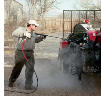
Figure 2 Power washing can be an effective way to clean equipment. Inspect after cleaning.
