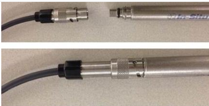
Figure 56. Cable to Sensor Connectors
