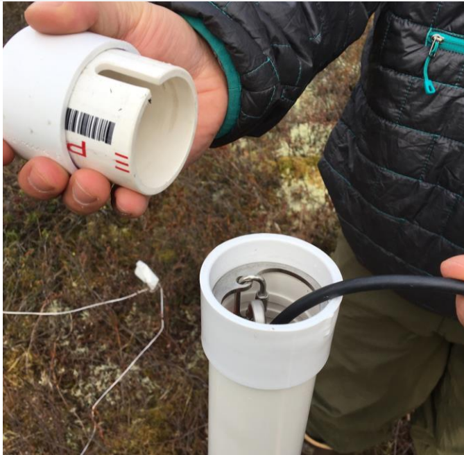
Figure 50. Remove PVC Cap from GWW (D19 CARI)
