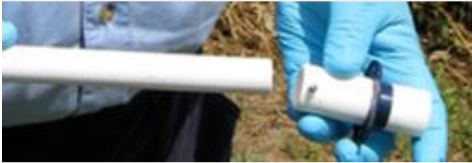
Figure 30. Assemble Surge Block (Source: ER [07])
