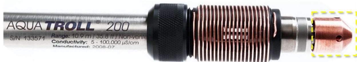
Figure 13. Ports for Pressure Sensor
