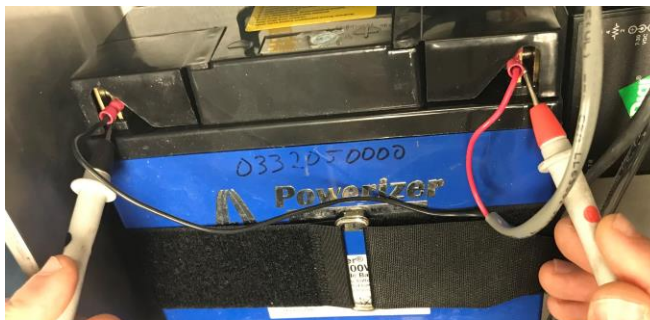
Figure 42. Use a DMM to Verify Battery Voltage
