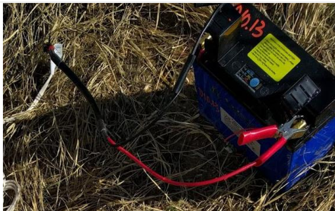
Figure 28. Connect Mini-Typhoon/Monsoon to 12V Battery (D10 ARIK)
