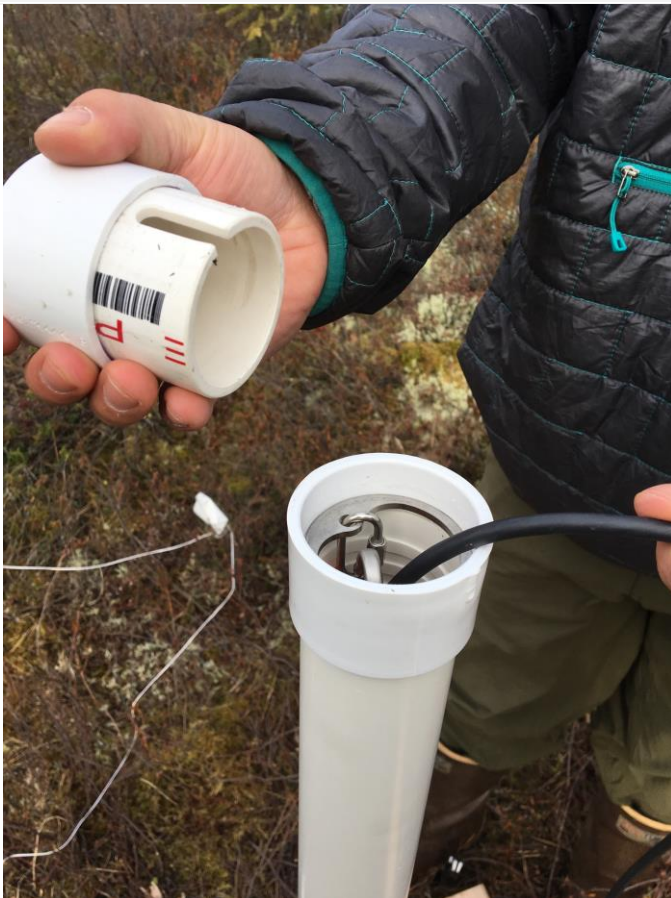
Figure 26. Remove GWW Cap (D19 CARI)
