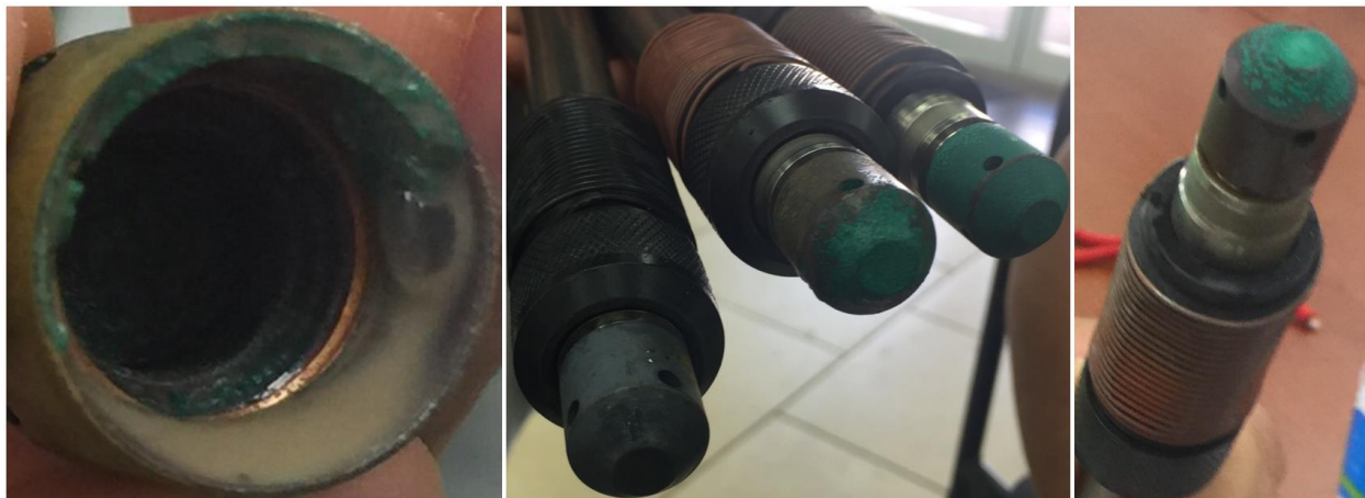
Figure 11. Examples of Biofouling on Aqua TROLL 200
