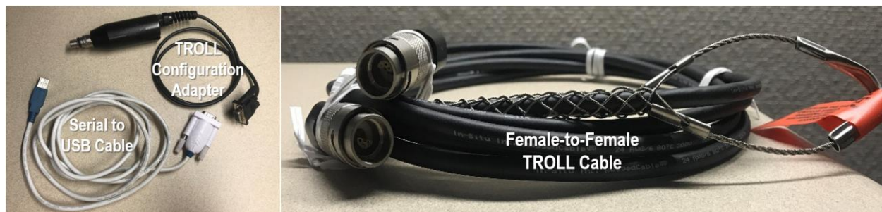
Figure 77. Cables to Configure Aqua TROLLs
