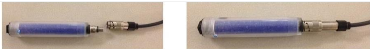
Figure 57. Desiccant Canister to Vented Cable Connectors
