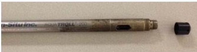
Figure 53. Unthread Black Nose Cone from Sensor
