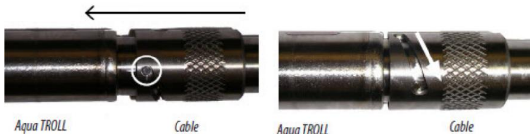
Figure 18. Lock Cable with Pin and Slot
