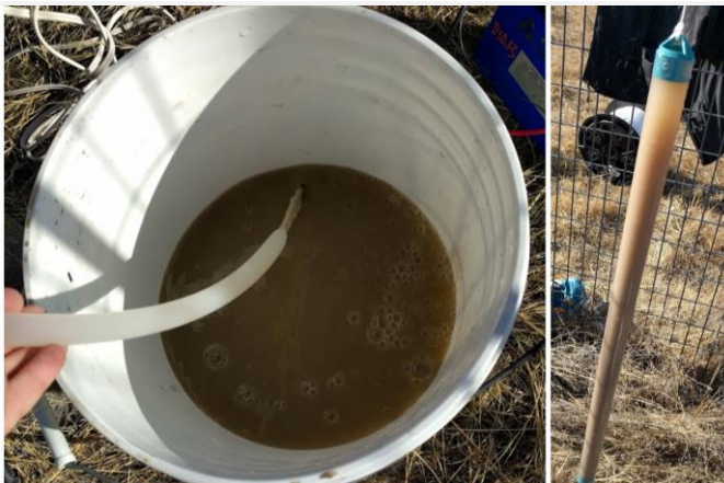
Figure 34. Muddy Water from Aggressive Mixing (D10 ARIK)
