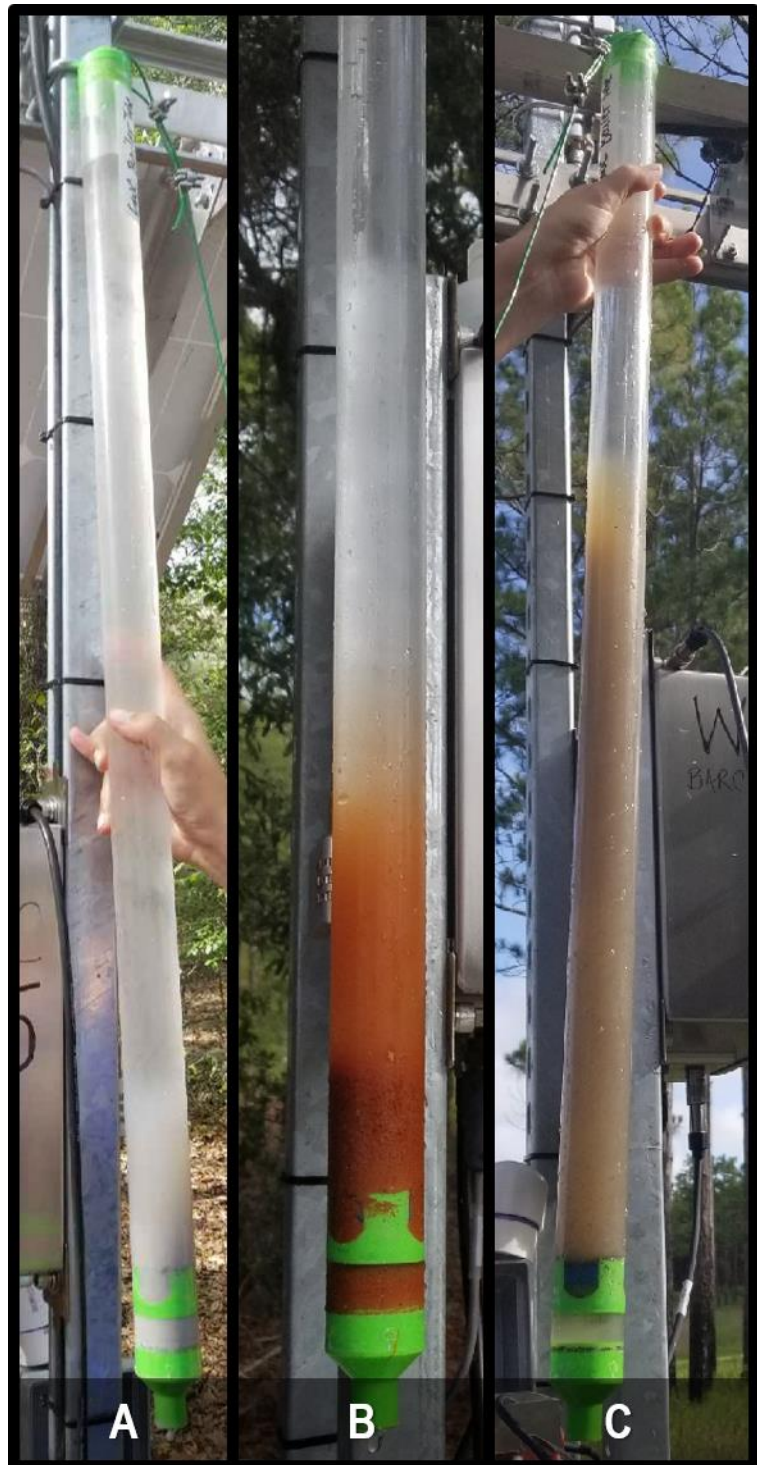
Figure 23. Water Clarity Sample in Bailer Tube Examples (D04)
