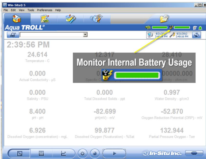
Figure 43. Win-Situ 5 Internal Battery Status Bar Screenshot
