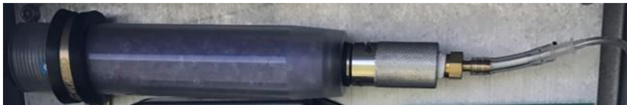
Figure 20. Desiccant in Radio Box with Vent Tube Attachment Close-up
