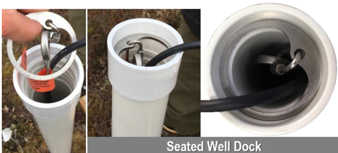
Figure 59. Well Dock in PVC casing
