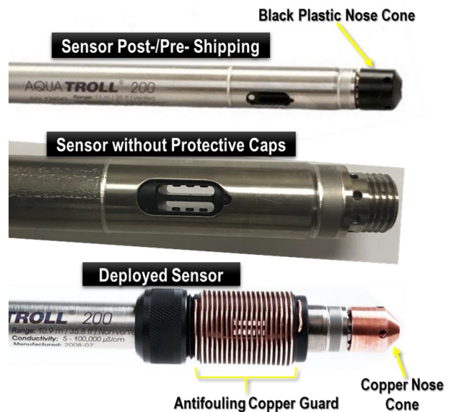
Figure 12. Aqua TROLL 200 Components
