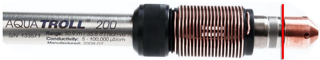
Figure 58. Red Line Identifies the Position to Measure for Sensor Cable Length
