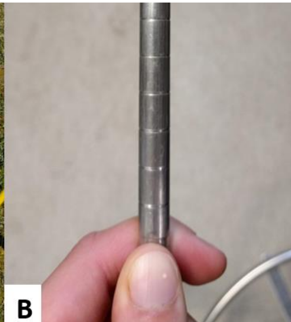
Figure 94. Measure thaw depth by inserting the thaw probe to the frozen interface (A) and reading the corresponding centimeter mark (B).
