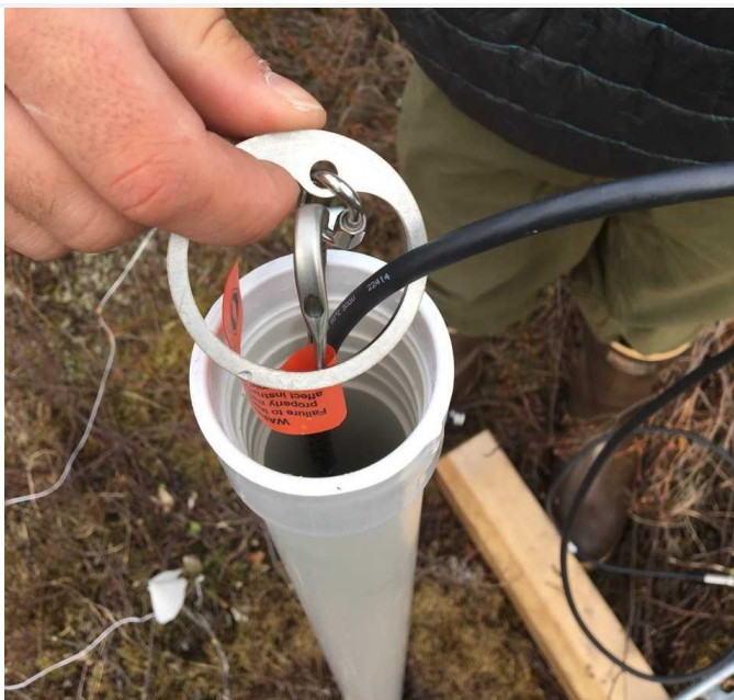
Figure 51. Remove Well Dock from GWW (D19 CARI)
