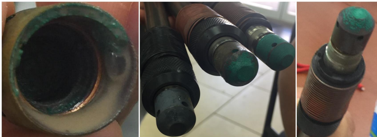
Figure 11. Examples of Biofouling on Aqua TROLL 200
