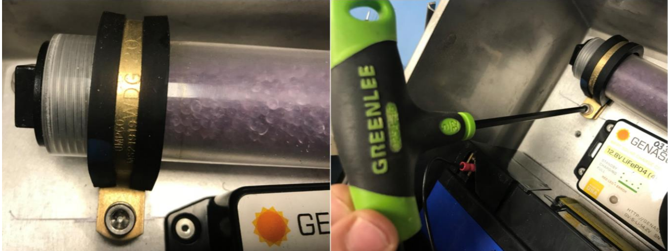
Figure 21. Loosen Clamp Securing Desiccant Canister to Radio/Power Box Back Plate with 5/32 Hex Wrench
