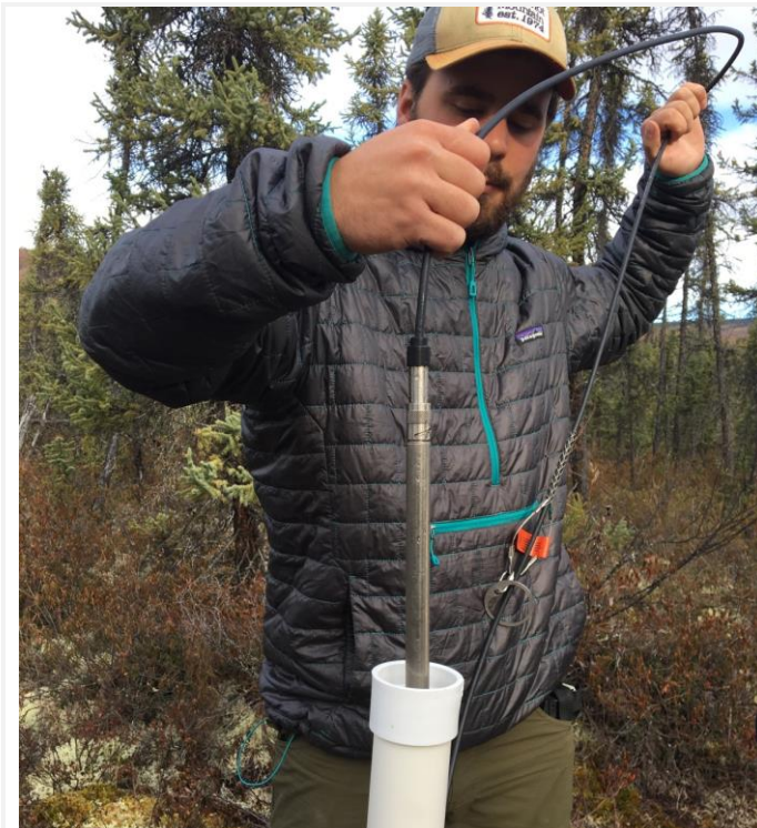
Figure 52. Remove Aqua TROLL 200 from GWW (D19 CARI)
