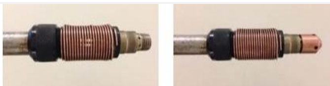
Figure 54. Install Antifouling Parts on Sensor
