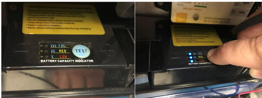
Figure 40. Press 12V Battery Test Button to Check Charge Level
