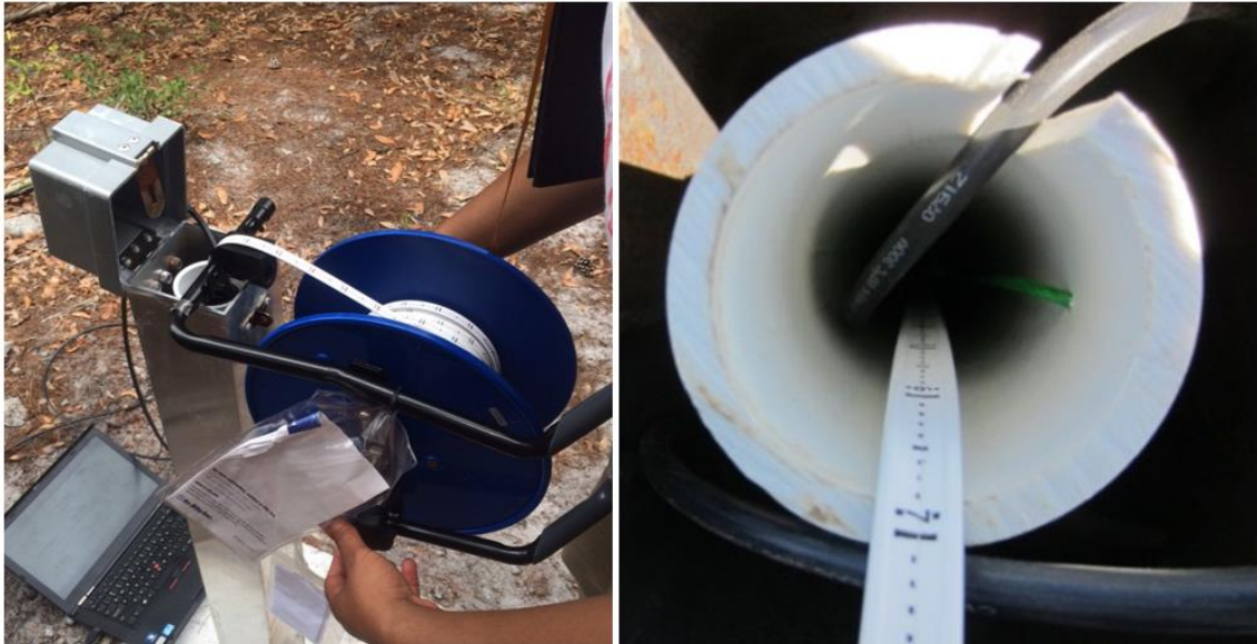
Figure 60. Water Level Tape to Measure Depth to Water
