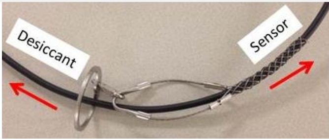
Figure 55. Cable and Wire Basket with Well Dock Orientation
