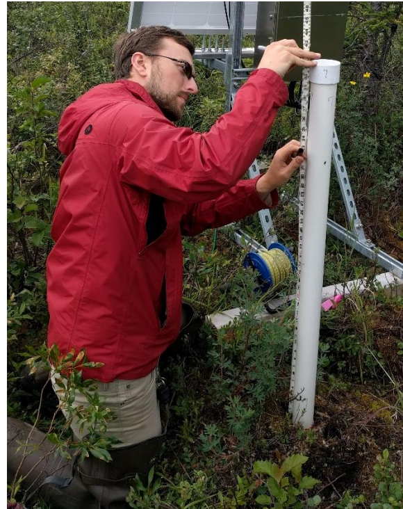
Figure 93. Measure from the Top of the GWW (with the cap removed) to the Ground Surface
