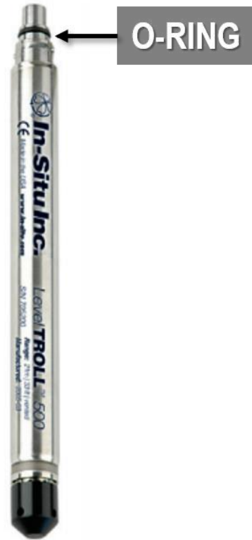
Figure 44. O-Ring Location on Level TROLL Sensor (Same Location for Aqua TROLL sensor)
