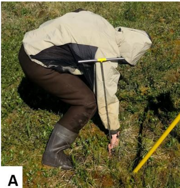
Figure 94. Measure thaw depth by inserting the thaw probe to the frozen interface (A) and reading the corresponding centimeter mark (B).
