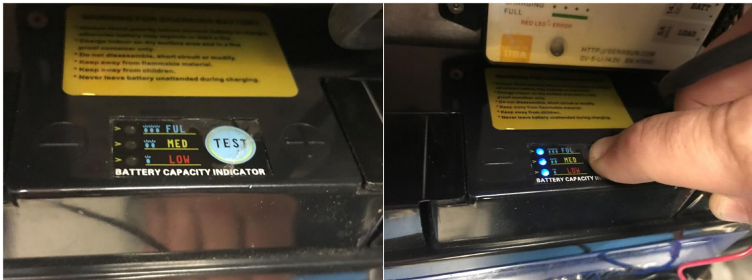
Figure 41. Press 12V Battery Test Button to Check Charge Level
