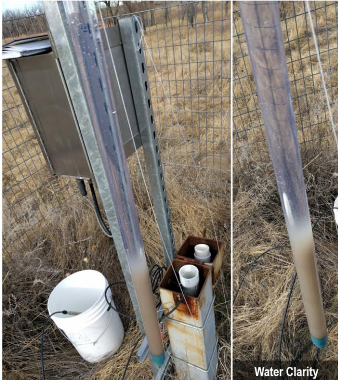
Figure 28. GWW Water Clarity Sample (D10 ARIK)
