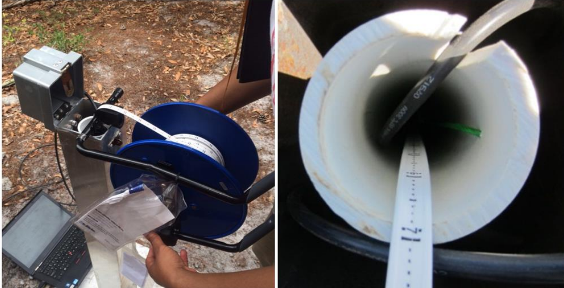
Figure 61. Water Level Tape to Measure Depth to Water
