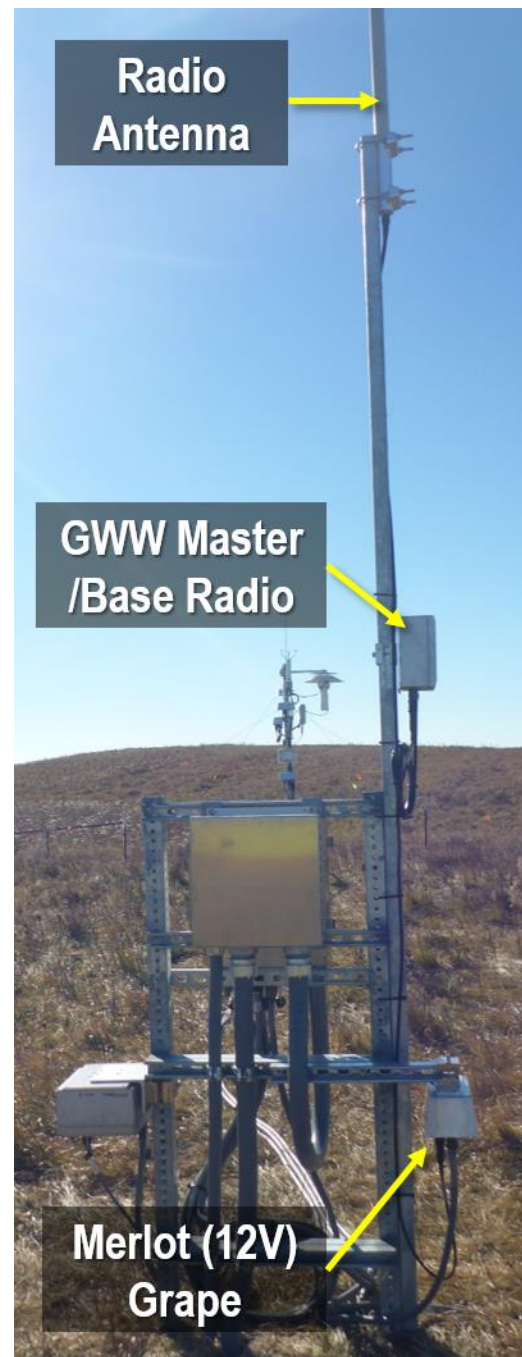
Figure 3. GWW DAS Components on Aquatic Met Station Device Post
