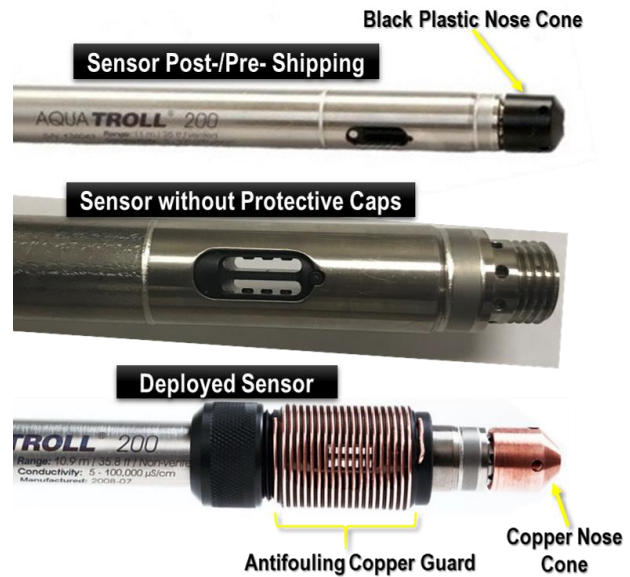
Figure 12. Aqua TROLL 200 Components
