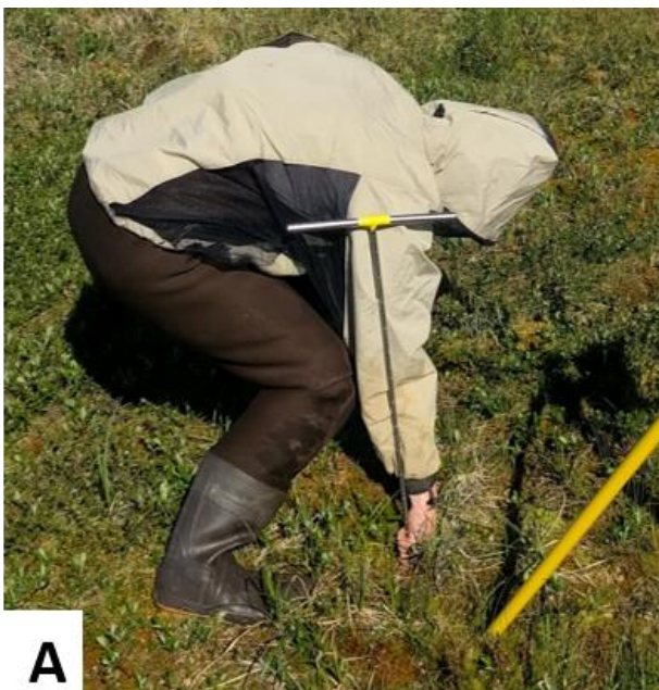
Figure 96. Measure thaw depth by inserting the thaw probe to the frozen interface (A) and reading the corresponding centimeter mark (B).
