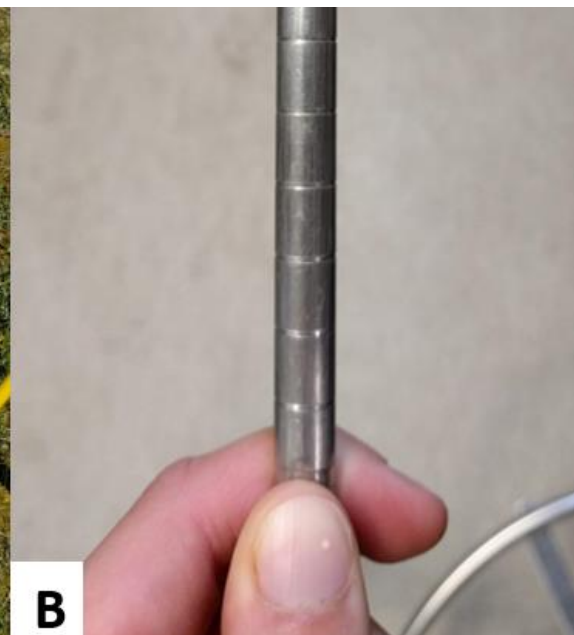
Figure 96. Measure thaw depth by inserting the thaw probe to the frozen interface (A) and reading the corresponding centimeter mark (B).
