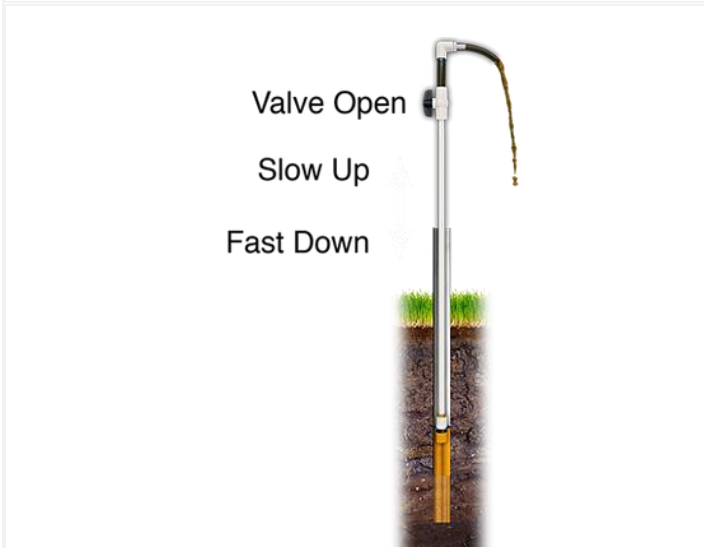
Figure 34. Flush GWW with Surge Block (ER [07])
