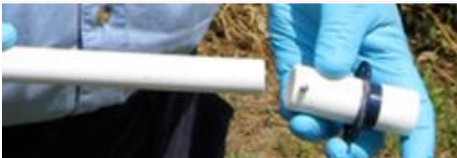
Figure 31. Assemble Surge Block (Source: ER [07])
