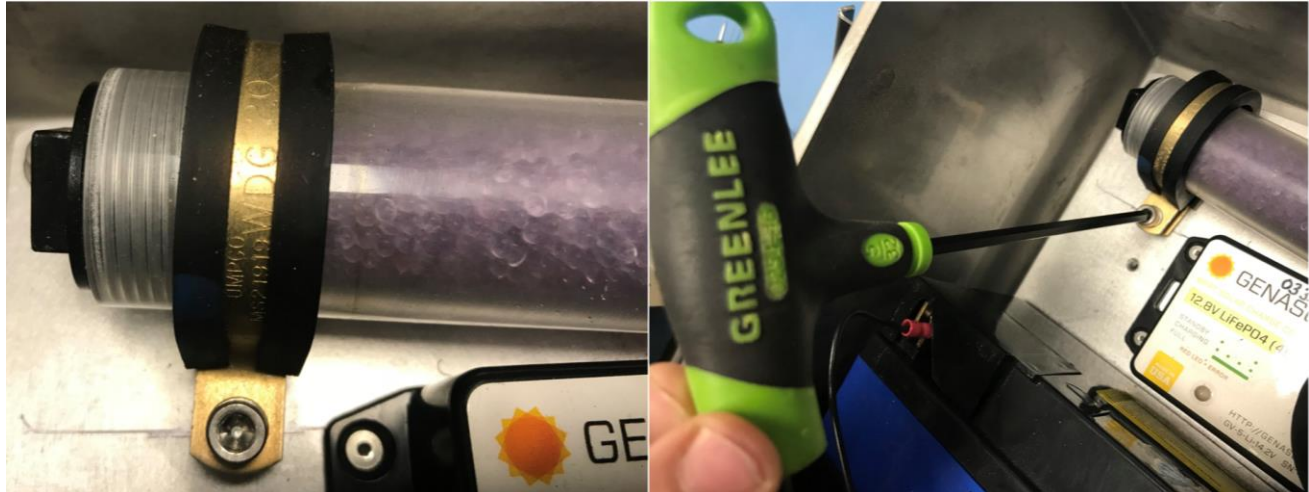
Figure 22. Loosen Clamp Securing Desiccant Canister to Radio/Power Box Back Plate with 5/32 Hex Wrench
