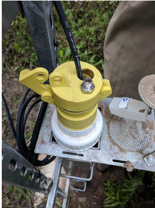
Figure 7. Snorkel cap modification for flood-risk sites.
