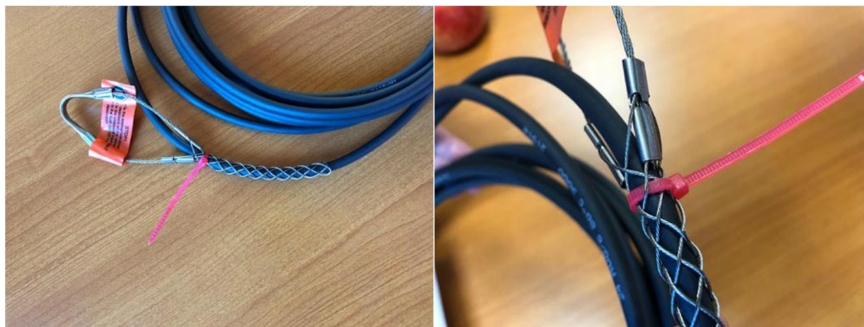
Figure 19. Secure Mesh Wire Basket to Sensor Cable
