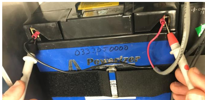
Figure 43. Use a DMM to Verify Battery Voltage
