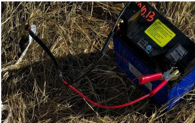
Figure 29. Connect Mini-Typhoon/Monsoon to 12V Battery (D10 ARIK)
