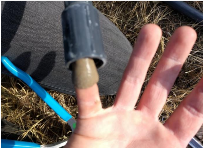
Figure 40. Sediment from Surge Block (D10 ARIK)
