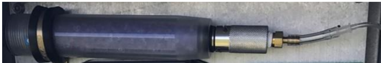
Figure 21. Desiccant in Radio Box with Vent Tube Attachment Close-up
