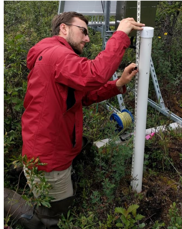
Figure 95. Measure from the Top of the GWW (with the cap removed) to the Ground Surface
