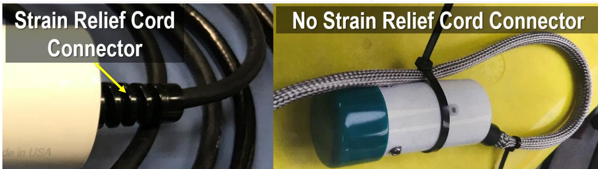
Figure 113. Biological Temperature Sensor Requires Cable Strain Relief – Use Zip Ties to Prevent Straining the Cable if the Sensor has No Connector
