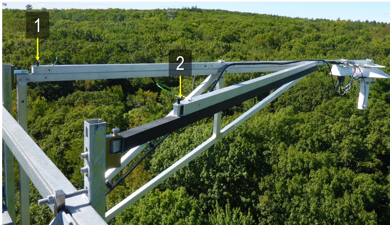
Figure 61. Components in Order of Operation to Retract the Tower Top Boom
