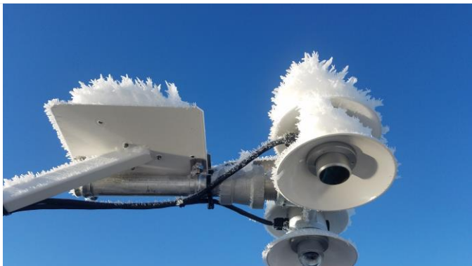
Figure 100. Radiation Sensor Winterization (D18 TOOL)
