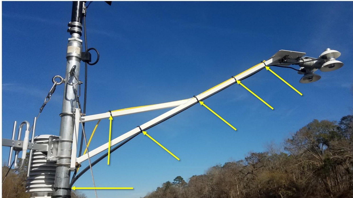
Figure 105. Re-dress Sensor Cables with Zip Ties (D03 FLNT)
