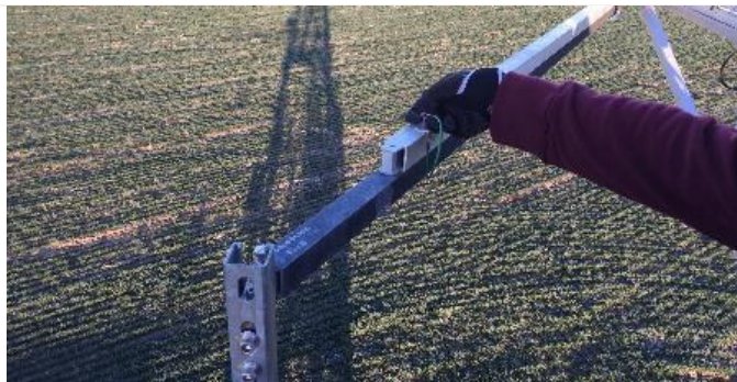
Figure 63. Remove the Second Pin from the Crossbeam (D06)
