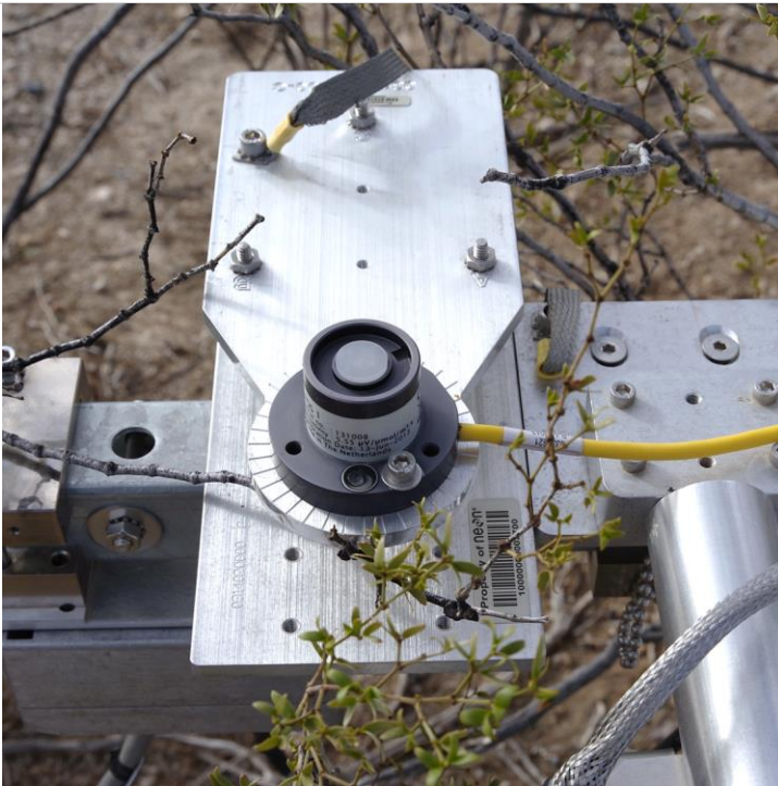
Figure 35. PAR Quantum Sensor mounted on ML1 on the TIS Tower.
