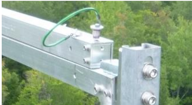
Figure 62. Remove the First Pin from the Longer Boom Arm
