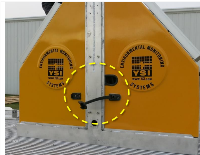
Figure 96. Unlatch to Remove Fiberglass T-Frame Covers (D09 PRPO)
