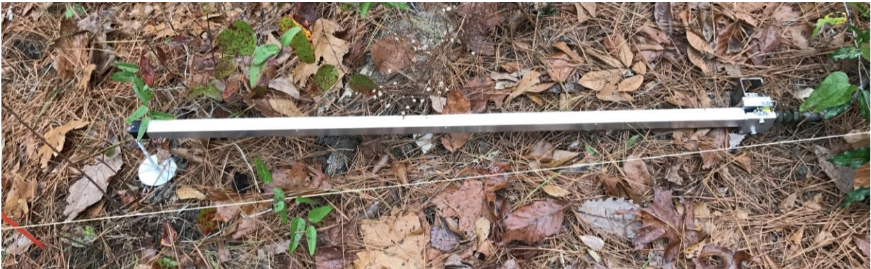
Figure 76. A Quantum Line Sensor (CF05840000) in Soil Plot 3 (D08 TALL)
