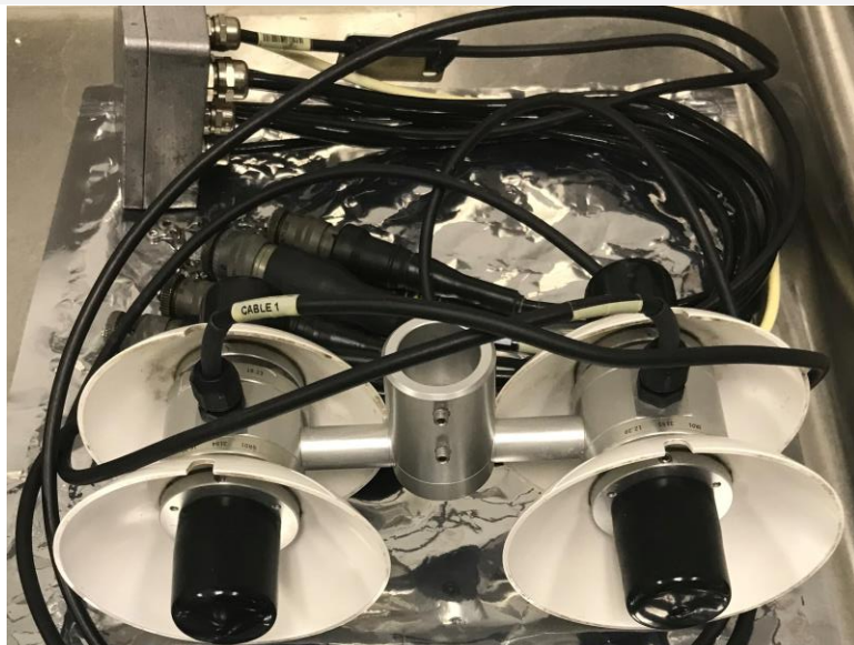
Figure 116. Net Radiometer with Black Caps over the sensors.
