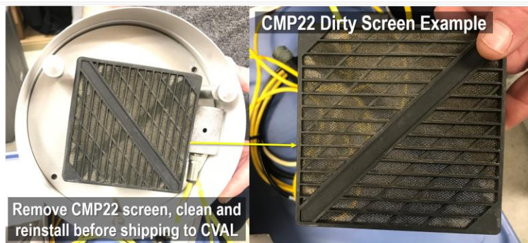
Figure 108. Primary Pyranometer Screen Requires Cleaning
