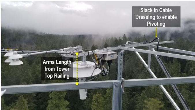
Figure 66. Tower Top Radiation Boom Pivoting Toward Tower Deck
