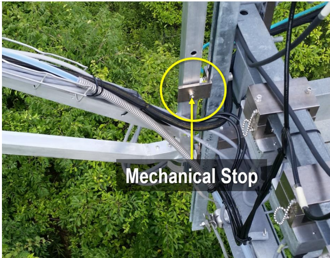
Figure 67. Mechanical Stop for Boom (D02 BLAN)
