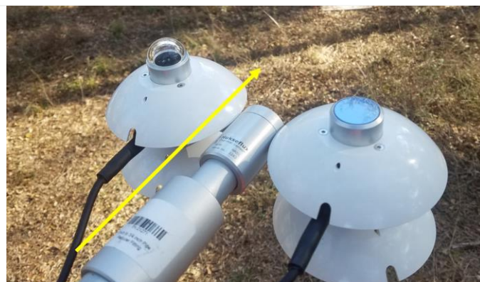
Figure 85. Removing the Net Radiometer
