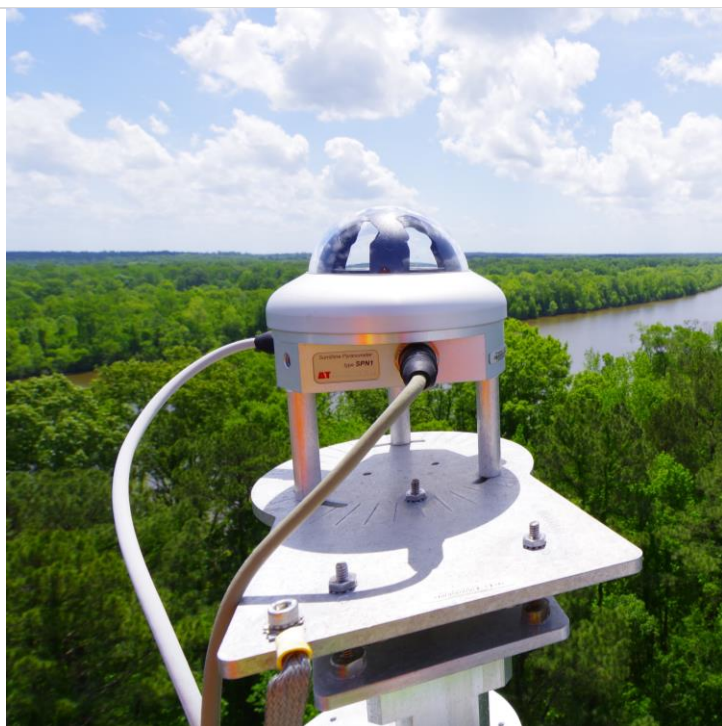
Figure 21. Sunshine Pyranometer mounted atop a TIS Tower.
