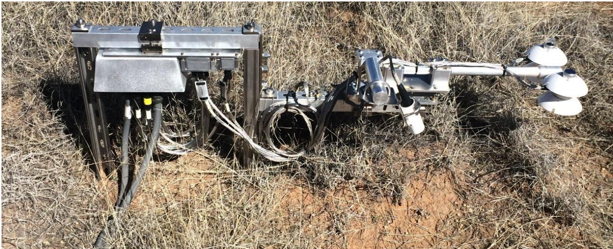
Figure 75. Radiation Arbor with Merlot Grape, Net Radiometer (CF05930000) and Biological Temperature Sensor (CF05940000) in Soil Plot 3 (D14 JORN)
