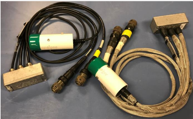
Figure 110. Biological Temperature Sensor Assemblies
