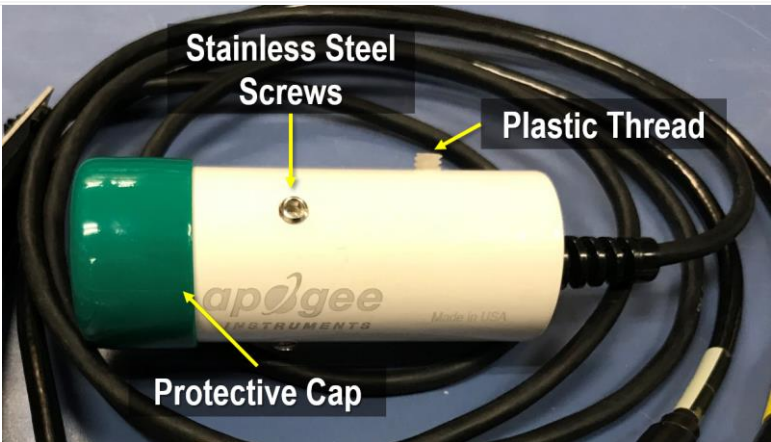
Figure 114. Biological Temperature Sensor must have these Components Post-Decontamination
