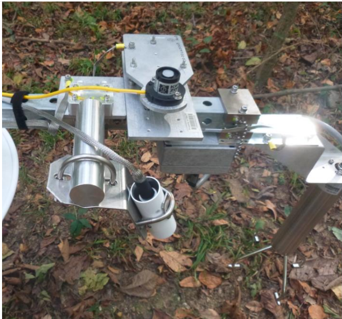
Figure 44. ML1 Profile Radiation and Biological Temperature Sensor Combo
