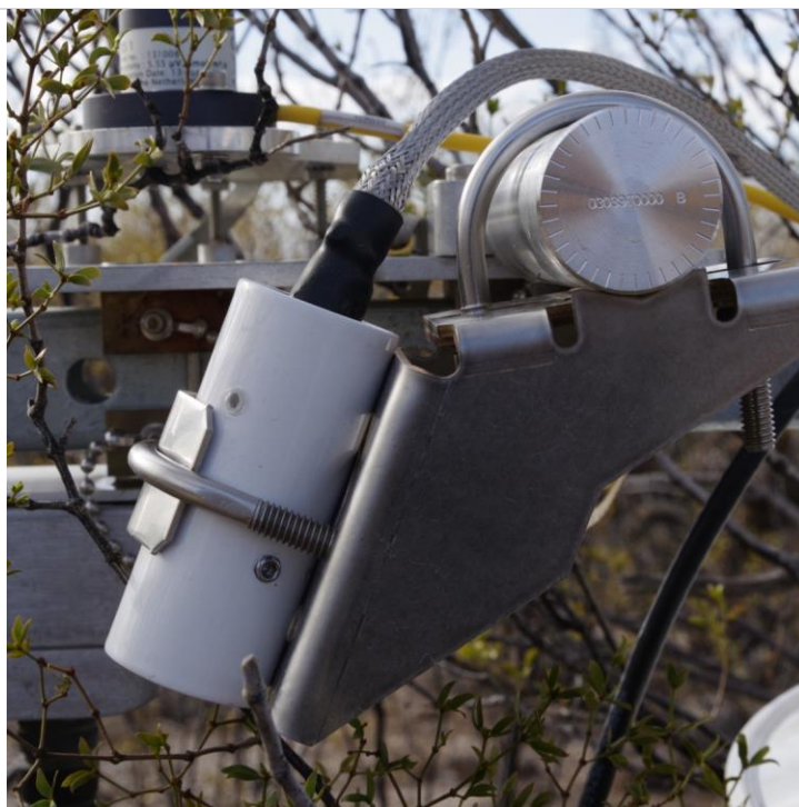
Figure 30. Biological Temperature Sensor mounted 22° from vertical.
