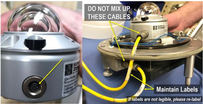
Figure 71. Primary Pyranometer Yellow Cables (CVAL)
