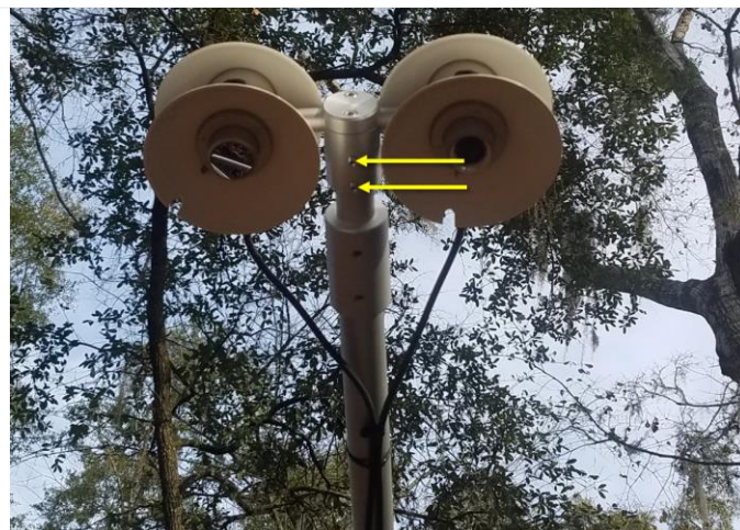
Figure 83. Remove Set Screws to Remove Net Radiometer
