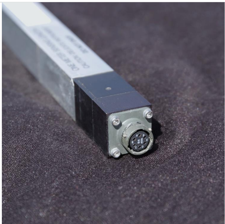
Figure 37. Close-up of the connector end of the Quantum Line Sensor.
