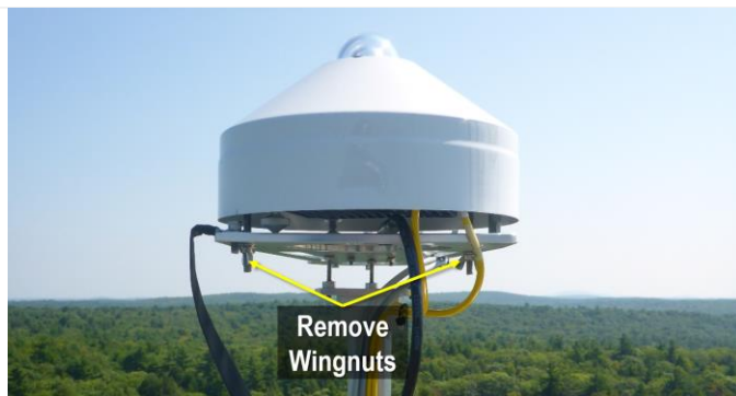
Figure 58. Remove the Primary Pyranometer from Mount Plate
