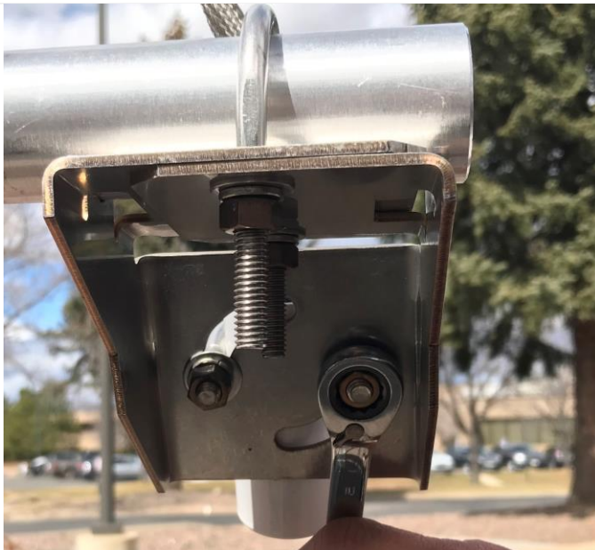
Figure 48. Remove U-Bolts with Speed Wrench
