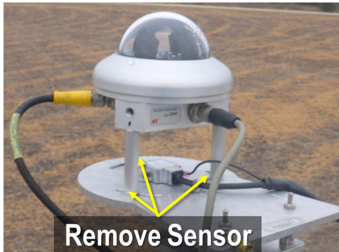
Figure 60. Remove SPN1 Sensor from Mount Plate
