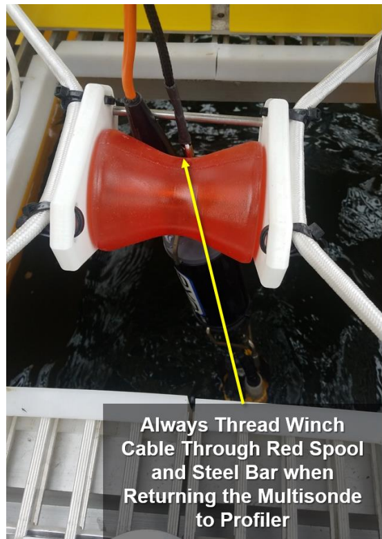
Figure 38. Thread the Winch Cable Properly to Return Multisonde to Water
