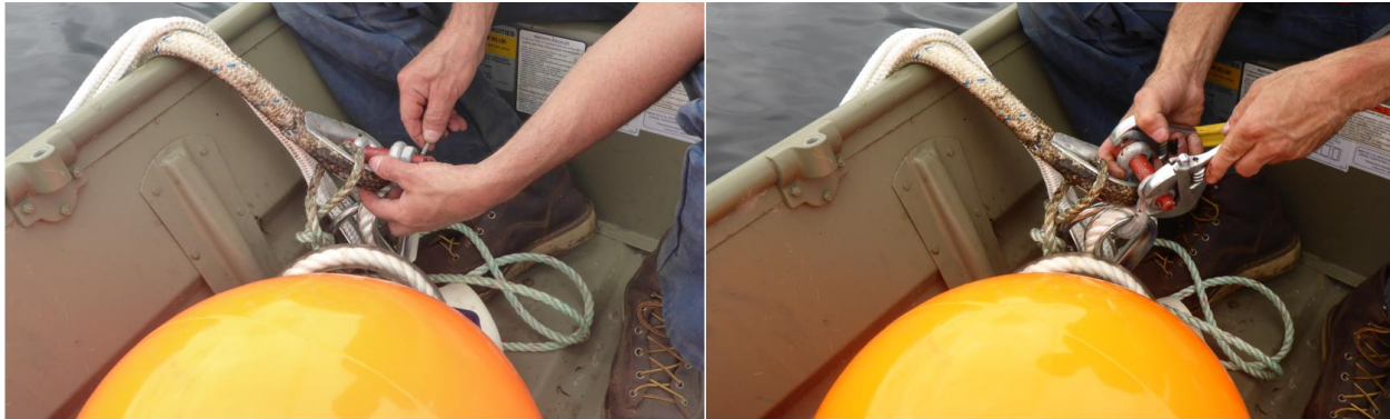
Figure 24. Remove Cotter Pin and Shackle Connecting Bridles to Line Float/Anchor Line
