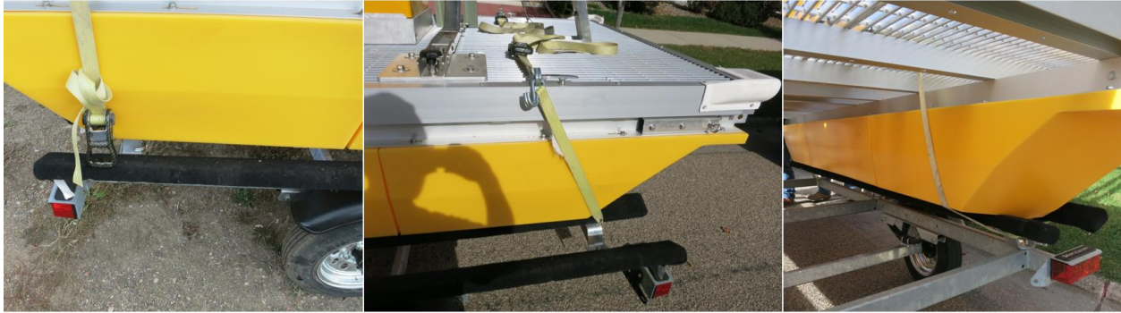
Figure 32. Ratchet Straps secure the AIS Lake Buoy to the Trailer
