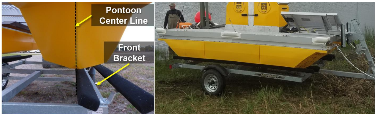
Figure 22. Mounting the AIS Lake Buoy on the Trailer
