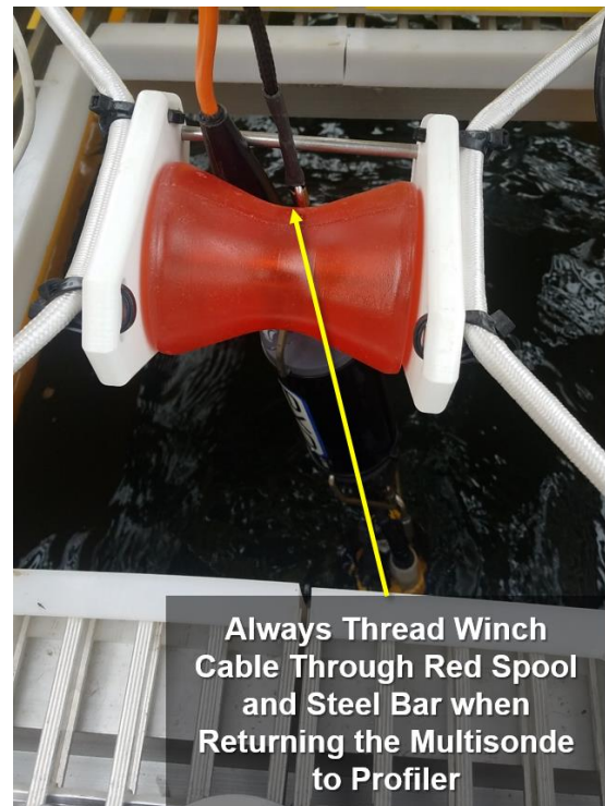
Figure 53. Thread the Winch Cable Properly to Return Multisonde to Water
