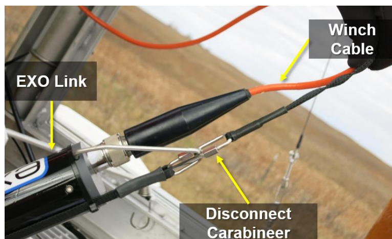
Figure 50. Disconnect Multisonde from the Lake Buoy Winch
