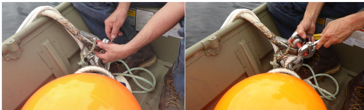
Figure 35. Remove Cotter Pin and Shackle Connecting Bridles to Line Float/Anchor Line
