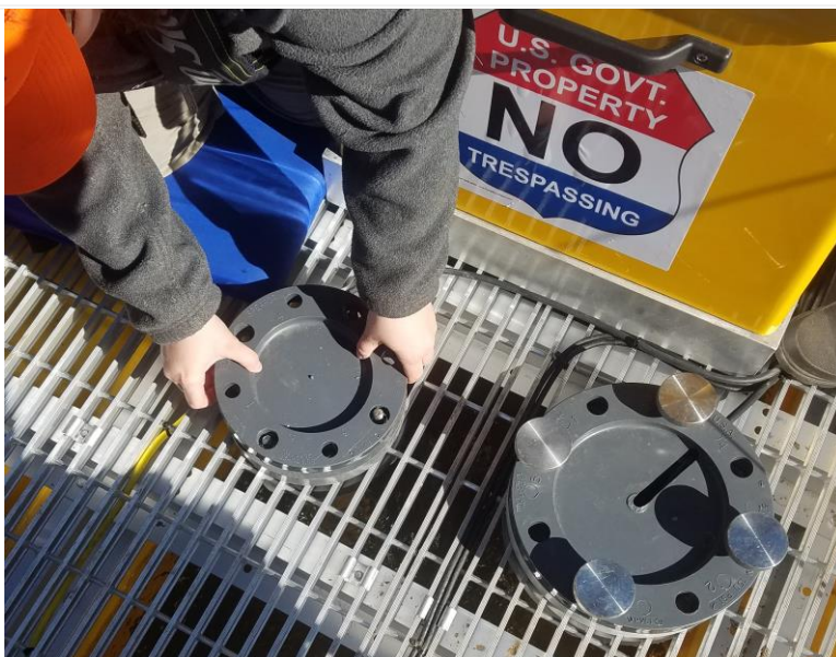
Figure 77. Lift Cap to Access Sensor in Tube
