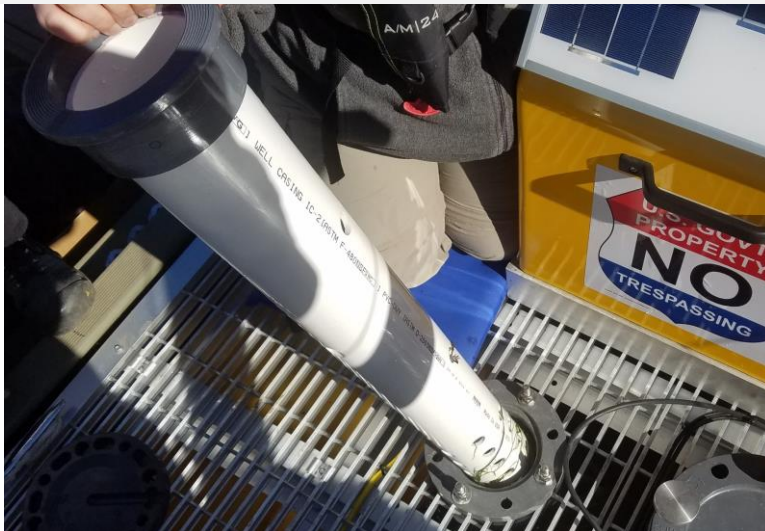
Figure 78. Remove Fixed Sensor Tube from Water
