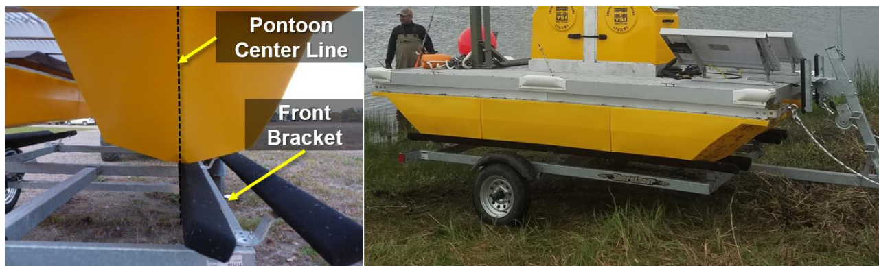
Figure 29. Mounting the AIS Buoy on the Trailer
