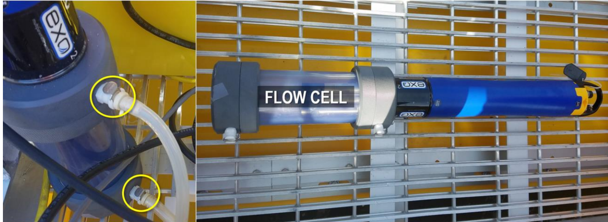
Figure 56. Remove Multisonde from Flow Cell
