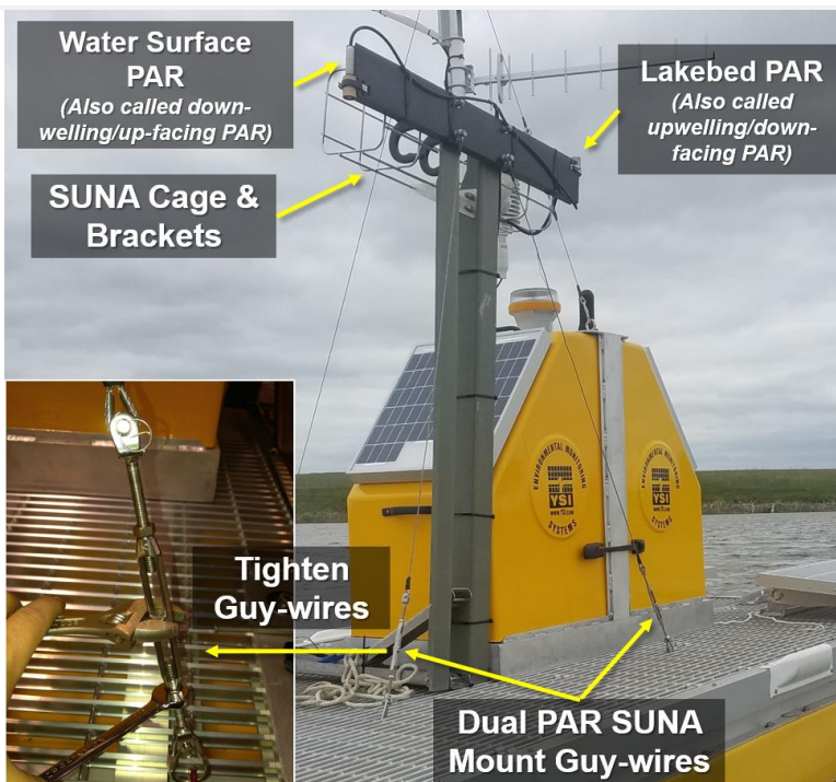
Figure 60. Raise the Dual PAR/SUNA Mount on the AIS Buoy
