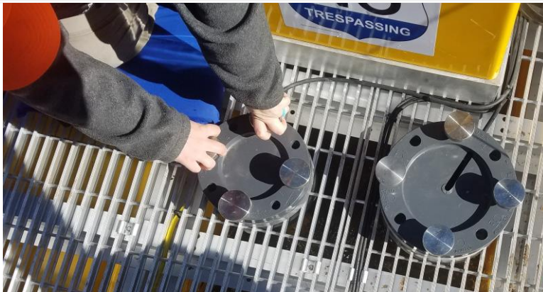
Figure 76. Remove Four Stainless Steel Knobs to Remove Tube
