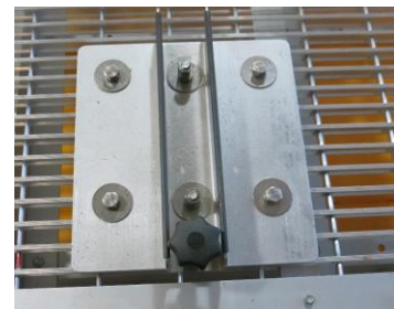
Figure 3. Dual PAR SUNA Mount Bracket - Scissor Risk Safety Note!
