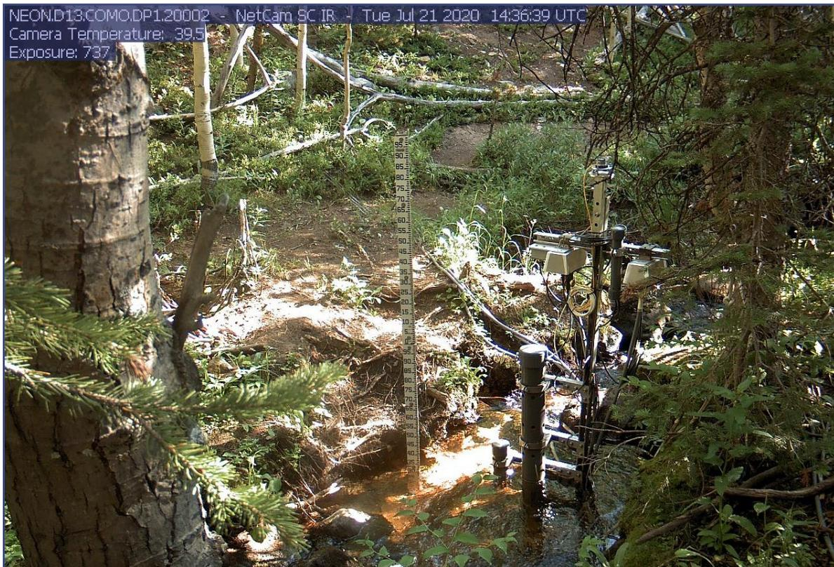
**Figure 1.** Example of a staff gauge installation.
