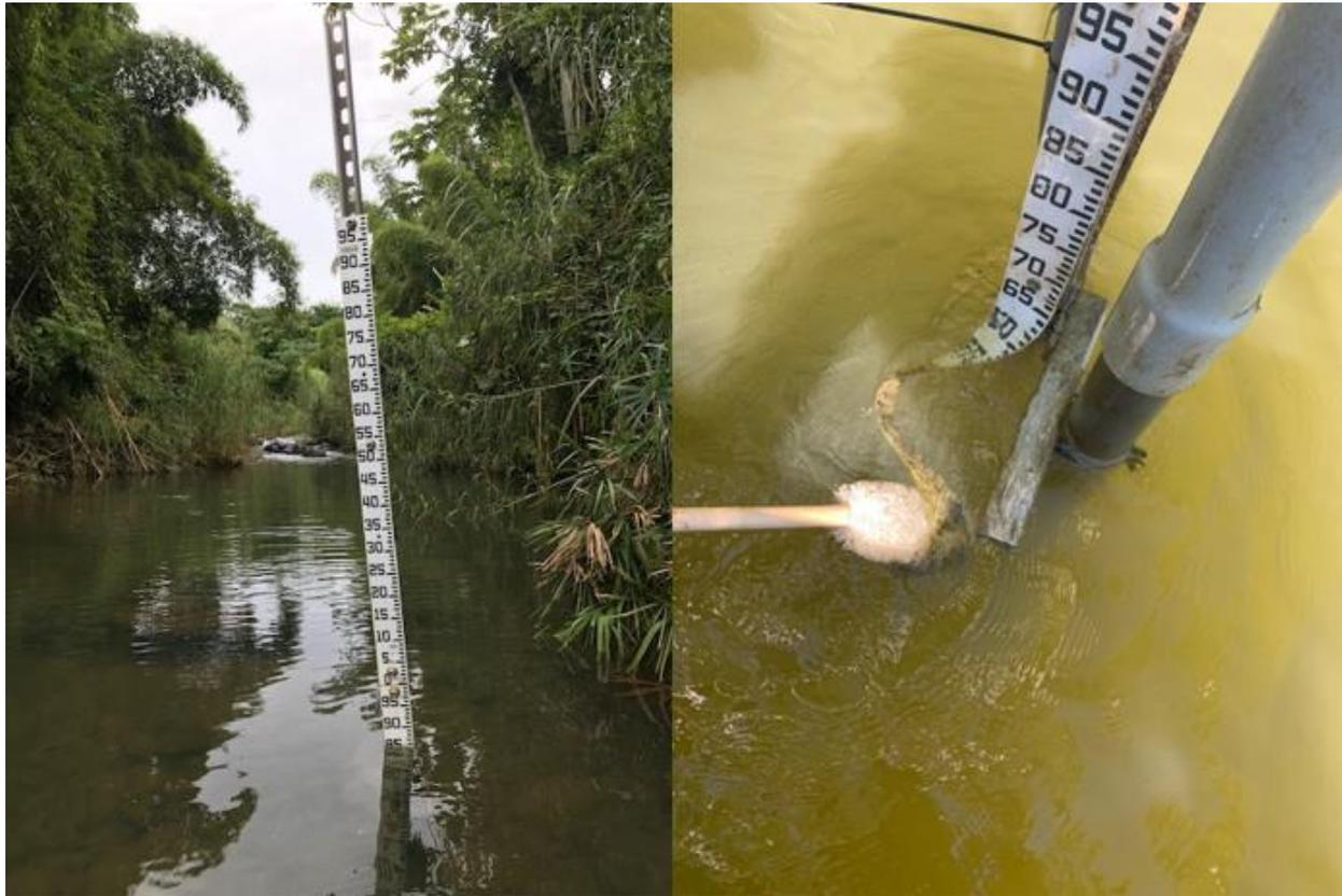
**Figure 2.** Examples of gauges needing repair.
