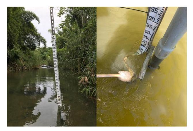
Figure 2. Examples of gauges needing repair.
