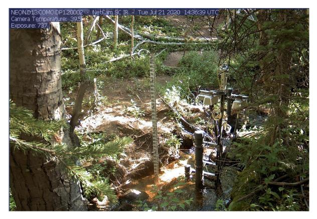
Figure 1. Example of a staff gauge installation.
