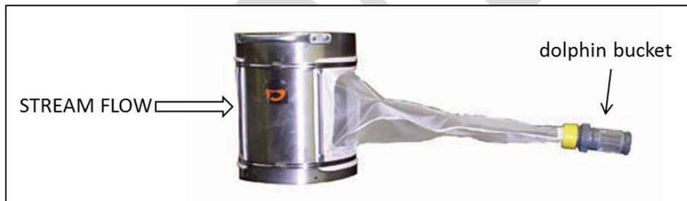
Figure 23. Hess sampler with collection net and dolphin bucket
