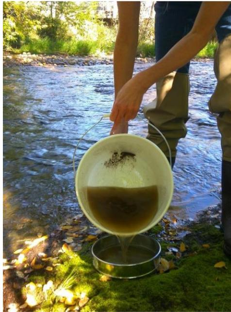
**Figure 25.** A field technician carefully pours water from the 3 gallon bucket into the sieve
