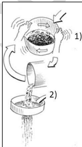
**Figure 24.** Process of elutriation
