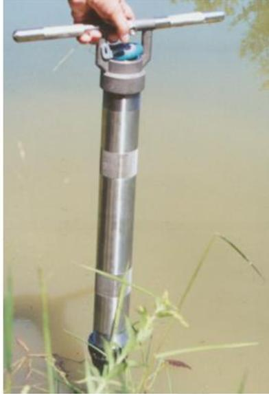
**Figure 21.** Push the hand corer through the water and into the sediments at a 90° angle
