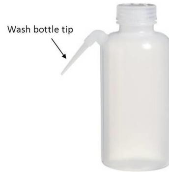
**Figure 10.** Removing the tip of the 500 mL wash bottle helps make rinsing easier and increases water pressure. This tip pulls easily out of the main body of the wash bottle.
