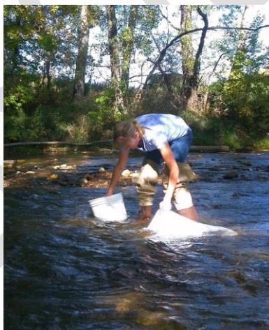
Figure 14. A field technician holds the Surber net on the stream bottom, and keeps the bucket nearby for depositing rocks from the base of the Surber
