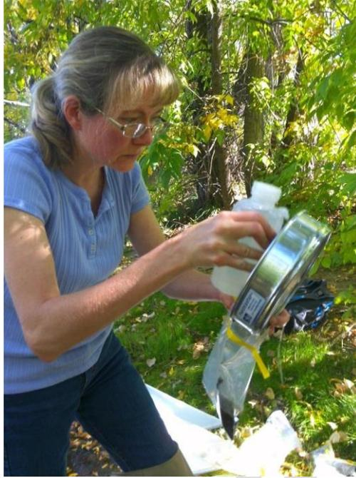
**Figure 26.** A field technician rinses the sample from the sieve into the open container with the 500 mL wash bottle
