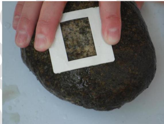
**Figure 17.** Template placement for epilithon protocol.
