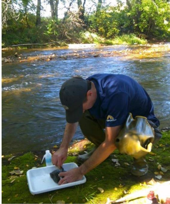
**Figure 16.** A field technician processes an epilithon sample on the stream bank, out of direct sunlight.
