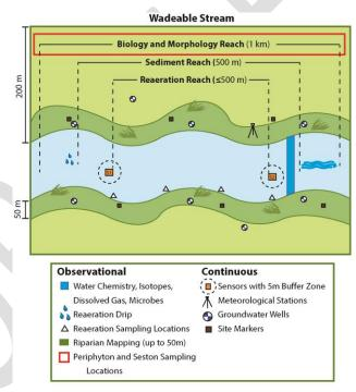
**Figure 12.** A generic site layout for wadeable streams with periphyton and seston sampling locations.
