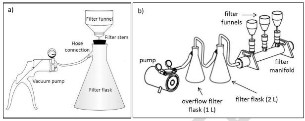
Figure 24. Filter apparatus setup: a) hand pump; b) filter manifold.
