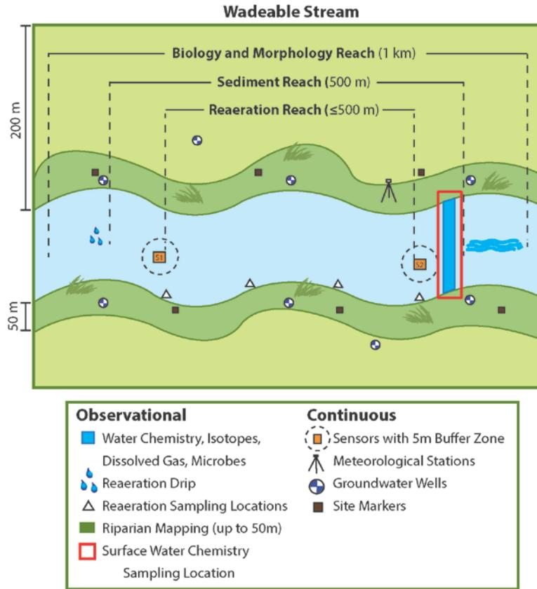
**Figure 1.** A generic wadeable stream site layout with water chemistry sampling locations
