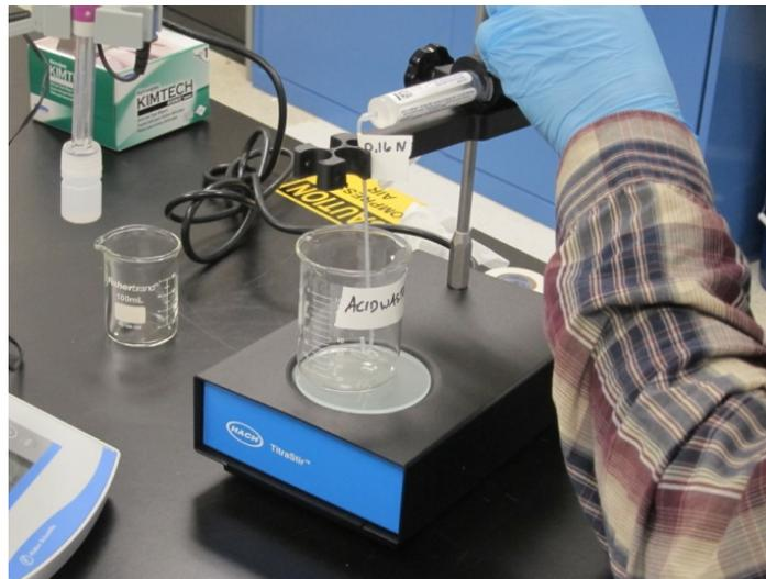
**Figure 10.** Expelling acid from digital titrator set-up into a temporary acid waste container
