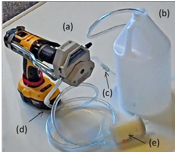
**Figure 6.** Pump and filter setup. Includes (a) a peristaltic sampling pump (modified from Woessner 2007), (b) a 4 L sample bottle, (c and d) tubing connectors to connect peristaltic and C-flex tubing, and (e) a capsule filter.
