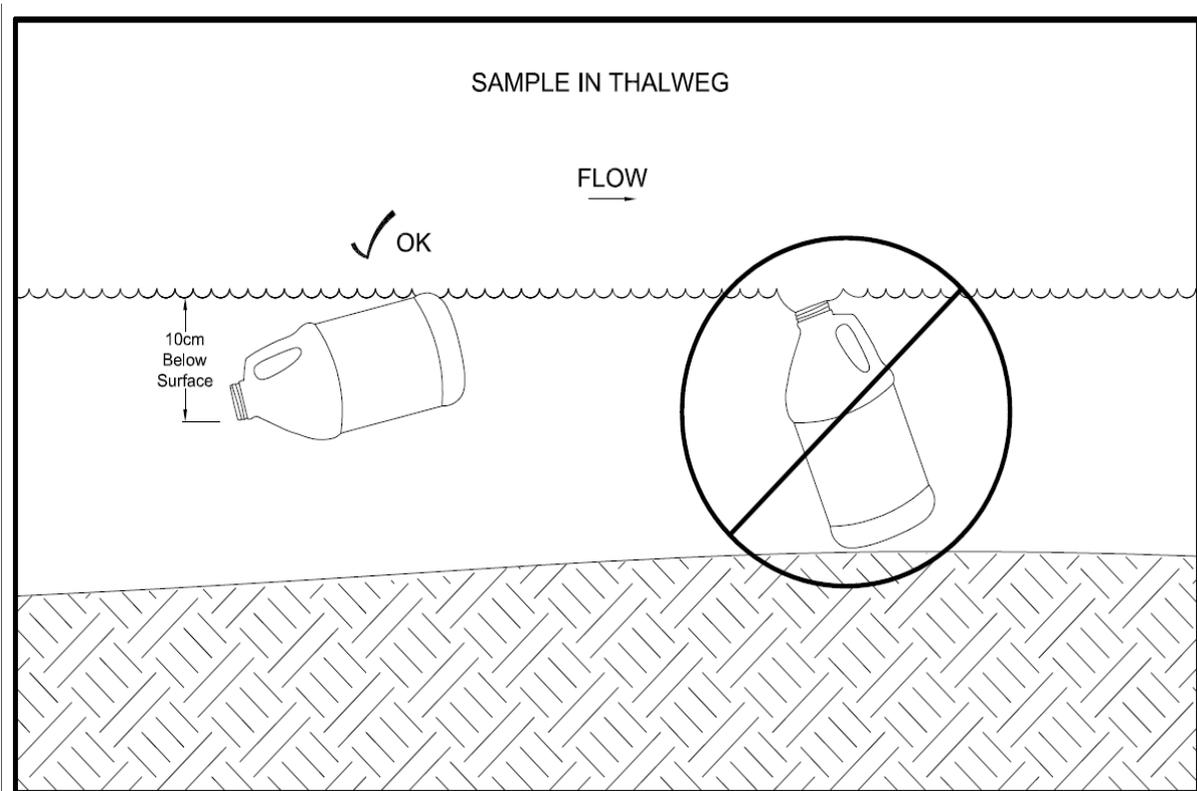
Figure 5. Diagram of proper and poor placement of a water sampling bottle
