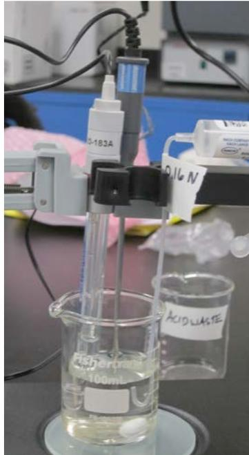
**Figure 11.** Titration setup with digital titrator, stir bar, pH meter, and temperature probe
