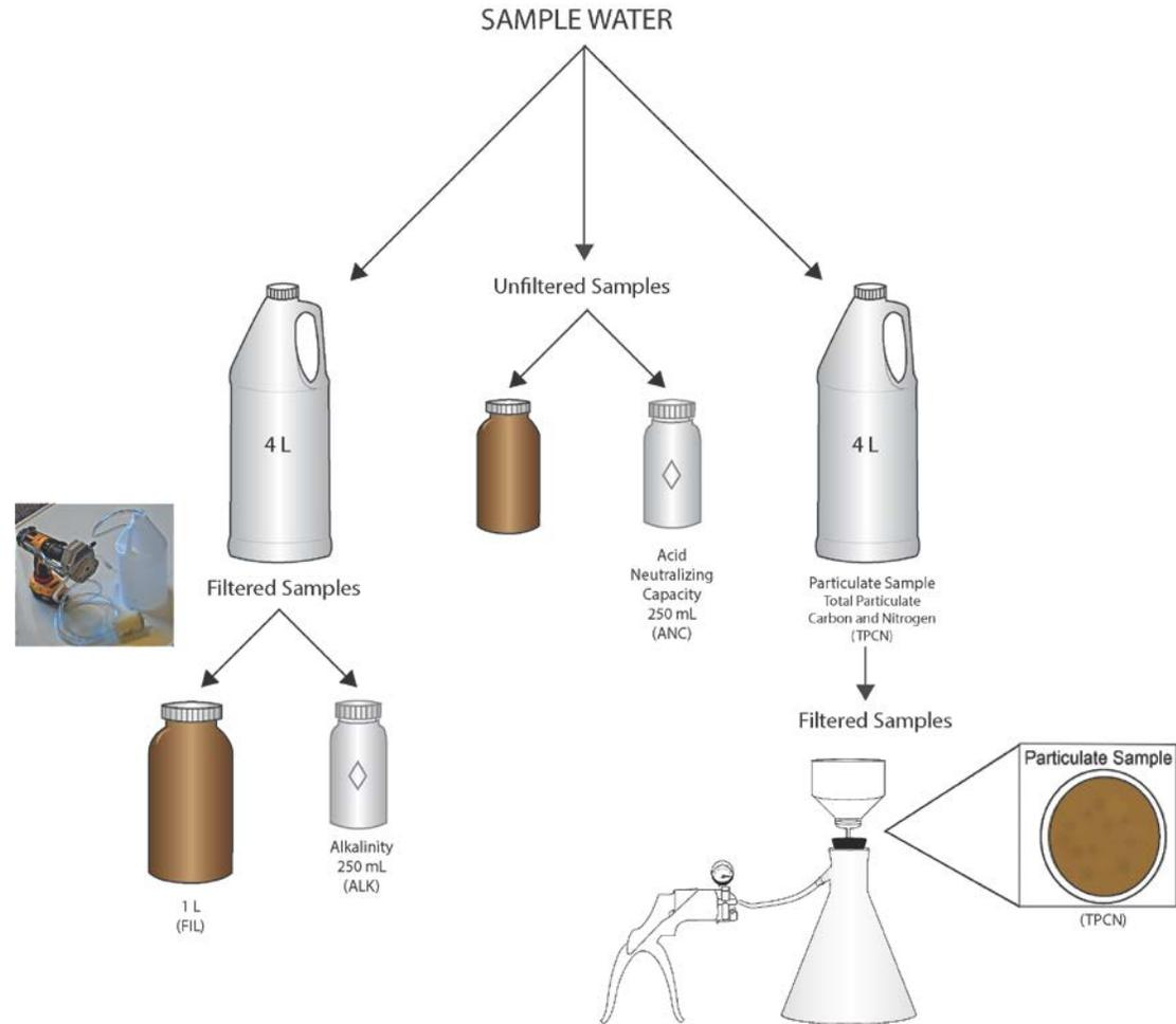
**Figure 3.** Flowchart of Water Chemistry Sample Collection and Filtration. ◊ Indicates 250 mL, wide-mouth sample bottles that remain at the Domain Support Facility for analysis. Letters in parenthesis indicate the codes that correspond to the chemistry labels (see Figure 4 a and b).
