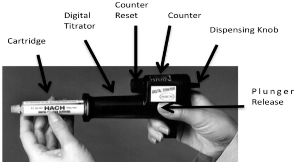
**Figure 8.** Inserting titrant cartridge into digital titrator. Photo from the Hach digital titrator manual.
