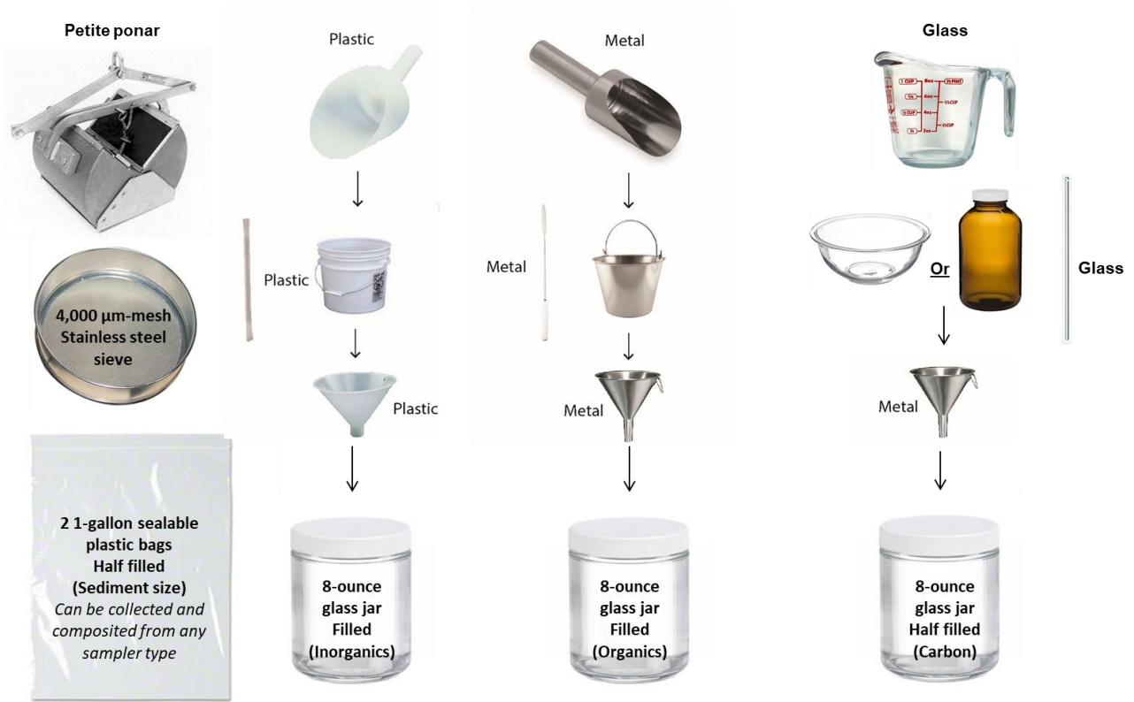
Figure 5. Sampling equipment used to collect sediments for each respective analyte type. Note, the petite Ponar and stainless steel sieve can be used to collect and screen sediments for any analyte Sediment size samples can be collected from any sampler type.
