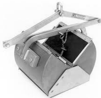
Figure 11. Petite Ponar sampler for use in lakes and non-wadeable streams
