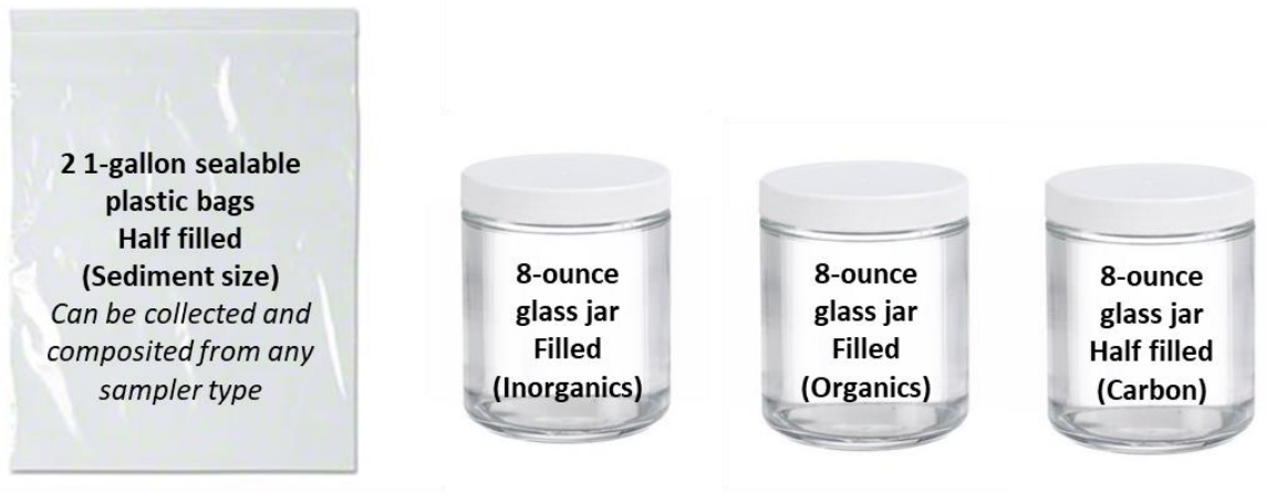
Figure 4. Example of clear Boston round glass jars with PTFE lined lid used for collecting sediment for inorganics, organics (PAH/PCB), and carbon (TOC/TC) analyses. Sediments for grain size samples are collected by filling 2 1-gallon (~3.8L) plastic Ziploc bags about half-full.
