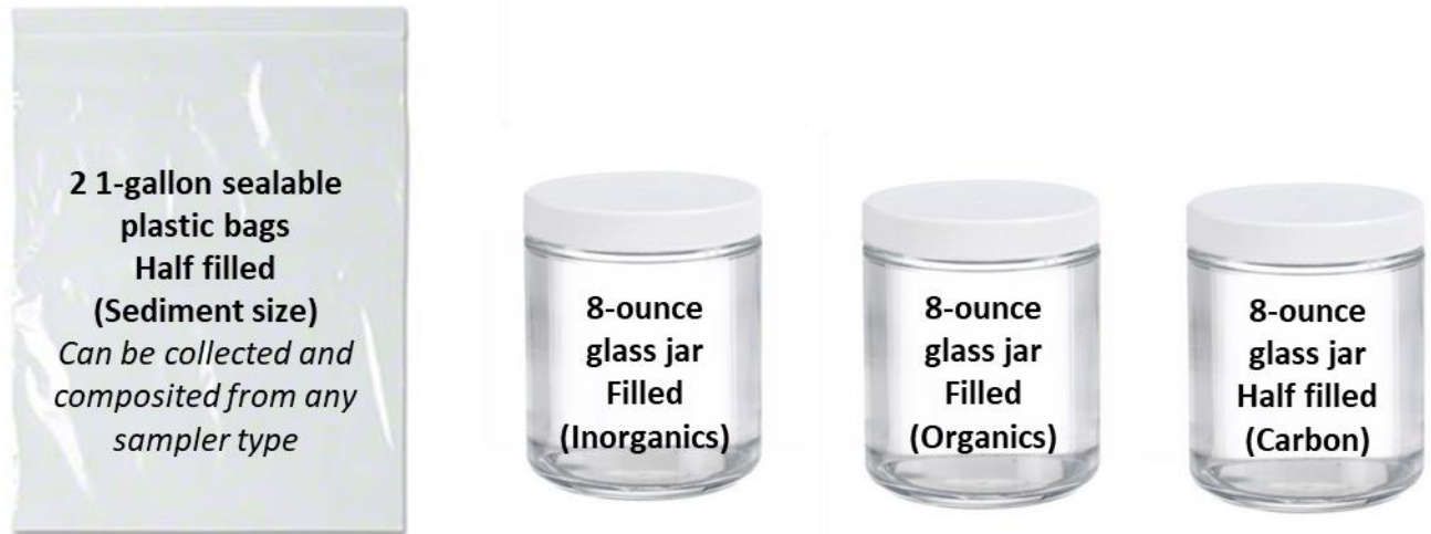
Figure 4. Example of clear Boston round glass jars with PTFE lined lid used for collecting sediment for inorganics, organics (PAH/PCB), and carbon (TOC/TC) analyses. Sediments for grain size samples are collected by filling 2 1-gallon (~3.8L) plastic Ziploc bags about half-full.
