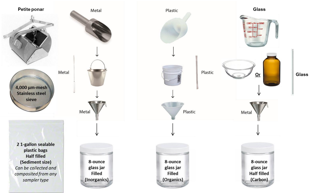
Figure 55 Note, the petite Ponar and stainless steel sieve can be used to collect and screen sediments for any analyte Sediment size samples can be collected from any sampler type.
