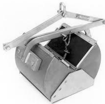
Figure 6. Petite Ponar sampler for use in lakes and non-wadeable streams
