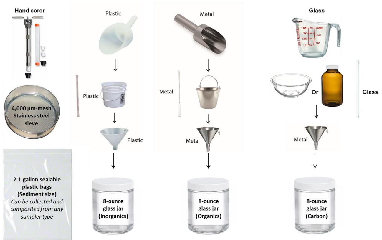
**Figure 6.** Sediment collection instruments by sample analyte type. When collecting sediments for inorganics with the hand corer, insert the plastic nosepiece. Note that the stainless steel sieve can be used for any analyte to remove sediments and other material larger than 2 mm. Sediment size samples can be collected from any sampler type.
