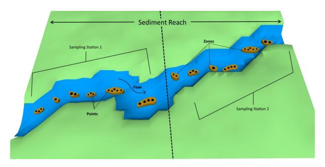
**Figure 3.** Identifying the location for sediment sampling in wadeable streams within the sediment reach. At each station, 5-10 depositional zones (brown blobs) are sampled. Within each depositional zone, up to 5 point samples are collected (black dots).
