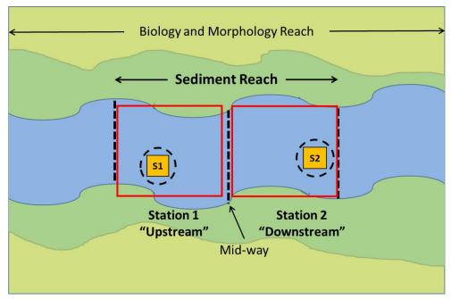
**Figure 2.** Sediment sampling stations at a wadeable stream site. Samples collected from Station 1 "Upstream" represent sediments upstream of the mid-way point of the reach. Station 2 "Downstream" samples are collected downstream of the mid-way point of the reach.
