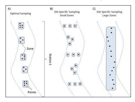
**Figure 10.** Diagram to exemplify determination of sampling zones based on site differences. A) Ideal sampling set up based on availability of different depositional zones (~1 m²); B) in sites with only random small pockets of sediment; and C) in sites where most of the stream bed is characterized by sedimentary or organic substrate.
