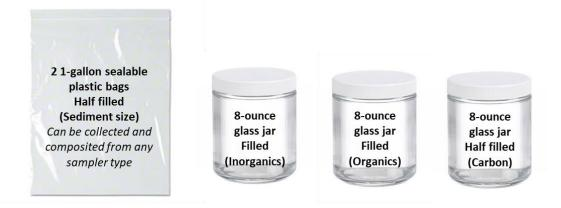
**Figure 5.** Example of clear Boston round glass jars with PTFE lined lid used for collecting sediment for inorganics, organics (PAH/PCB), and carbon (TOC/TC) analyses. Sediments for grain size samples are collected by filling 2 1-gallon (~3.8L) plastic Ziploc bags about half-full.
