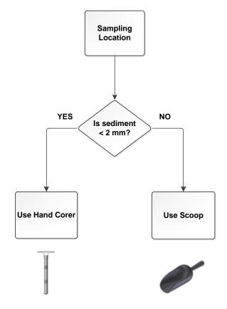
**Figure 4**. Decision flow chart for determining appropriate sampler to use in the field. **Note:** if the sediments depth is shallow (< 3 cm) the scoop is the more appropriate collection tool.
