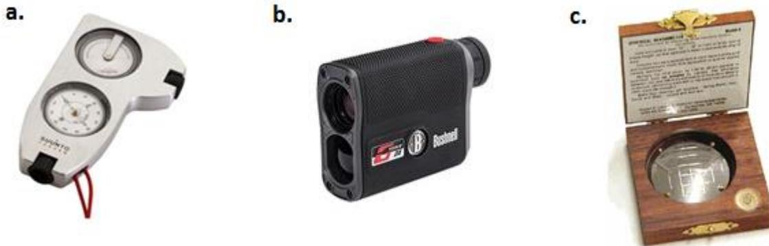
Figure 4. An example of a) a tandem clinometer used both as a compass and for measuring angles and b) a laser rangefinder which uses a laser beam to determine the distance to an object and a clinometer for determining height ; and c) a spherical densiometer used for determining % canopy cover.
