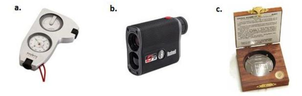
**Figure 4.** An example of a) a tandem clinometer used both as a compass and for measuring angles and b) a laser rangefinder which uses a laser beam to determine the distance to an object and a clinometer for determining height; and c) a spherical densioneter used for determining % canopy cover.
