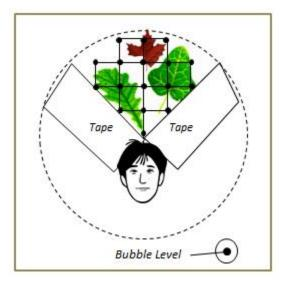
Figure 6. Preparing and reading a densiometer
