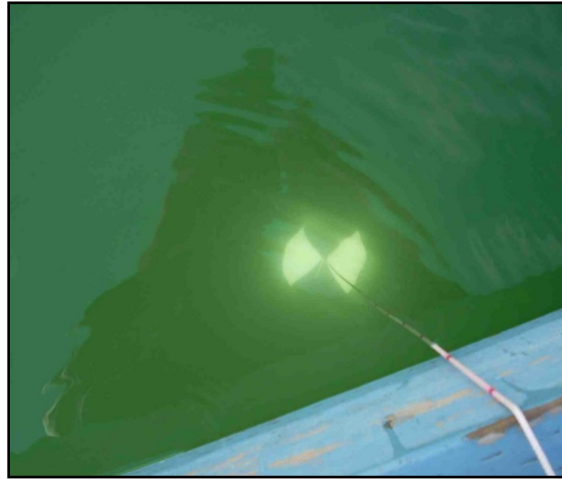
Figure 4. Illustration of Secchi disk lowered into water with shading
