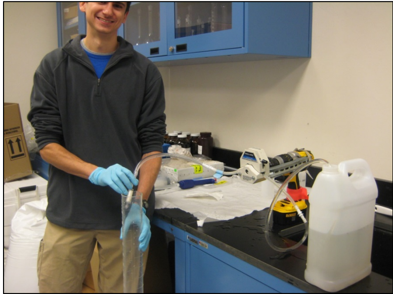
Figure 7. A field technician demonstrates pumping sample water out of the 4 gallon HDPE jug, through the peristaltic pump, through the Sterivex® filter, and into a graduated cylinder to measure the volume filtered.
