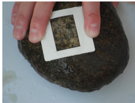
Figure 16. Template placement for epilithon protocol. (Note: Samples should not be processed in direct sunlight.)
