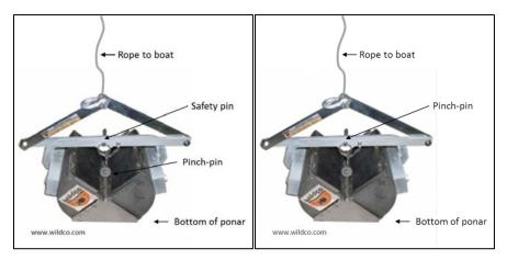
Figure 12. Example of petite ponar setup
