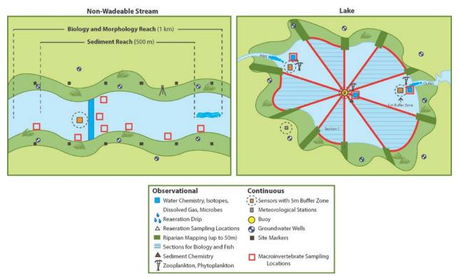
Figure 9. Generic site layouts for lakes and non-wadeable streams with macroinvertebrate sampling locations
