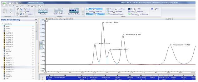
Verify that all appropriate standards are used to make the curves for each component in the Calib. & PM view setting on the Calibration tab.
