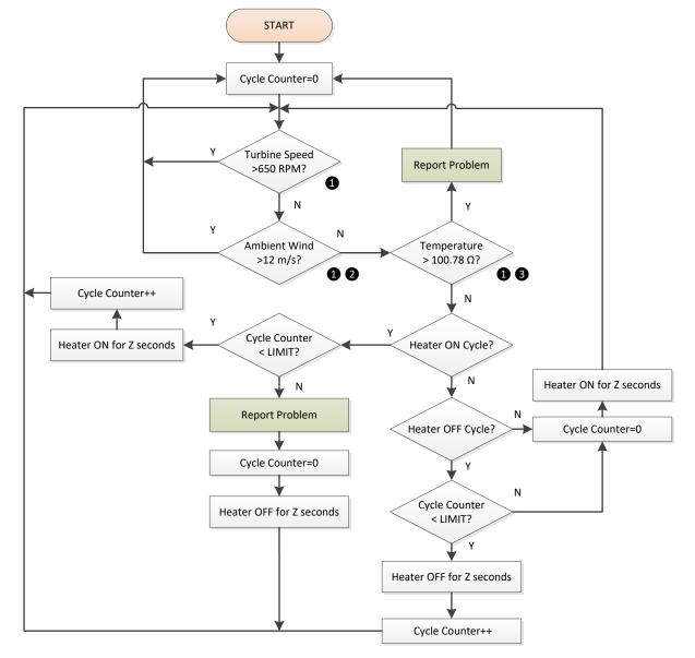
1 30 Seconds Average for Turbine Speed, Ambient Wind and Temperature
