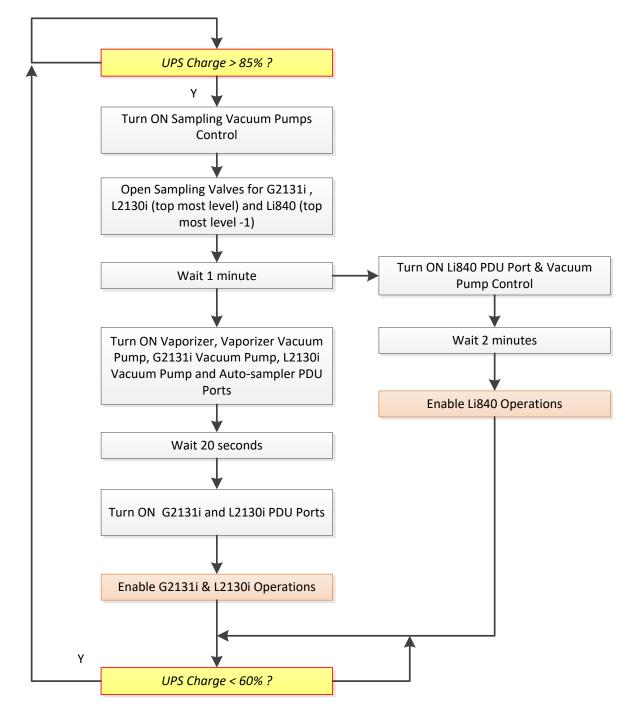
Figure 3. Flow chart for G2131-I and L2130-I power start up sequence.
