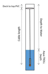
Cable length + Dock to top PVC = Depth to water + Aqua Troll Depth
