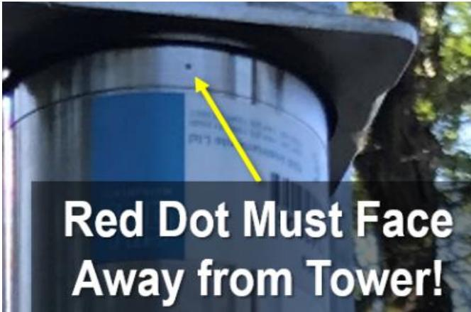
Figure 22. Orient Red Dot or Red Line Away from Tower (D06 KING).
