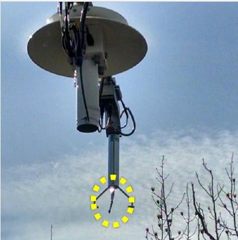
**Step 6.** Do a closer inspection of each spar of each 2D Sonic Anemometer for any more subtle misalignments of the spars.
