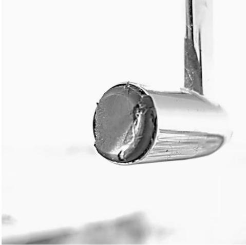
**Step 1.** Visually inspect each face of the transducers for any damage to the black transducer caps.
