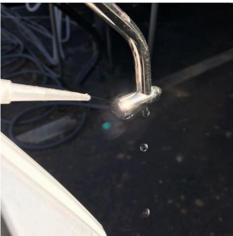
**Step 6.** Rinse once more with distilled or DI water and allow to air dry
