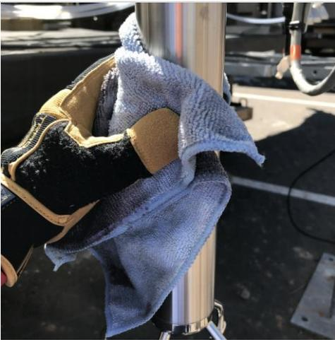
**Step 2.** Wipe down and clean the cylindrical sensor body.
