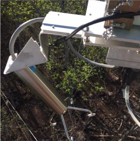
**Step 1.** Visually inspect each 2D Sonic Anemometer for any obvious misalignments or sensor mount damages.
