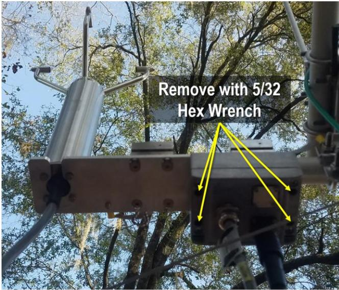
Figure 28. Remove Junction Box (D03 FLNT).
