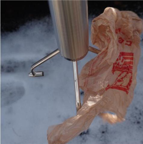
**Step 1.** Visually inspect the spars and transducers and remove any debris blocking the sonic paths.
