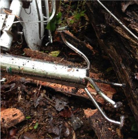
**Step 5.** Visually inspect each 2D Sonic Anemometer for any obvious damages to the spars (i.e. obvious misalignments).
