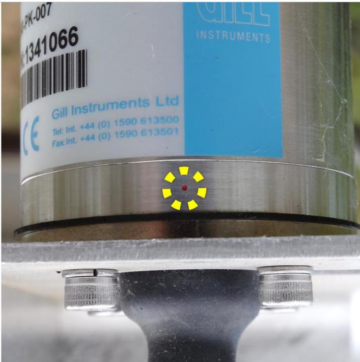
**Figure 3.** Close-up view of the Red Alignment Dot on Non-Heated and Heated 2D Sonic Anemometers.
