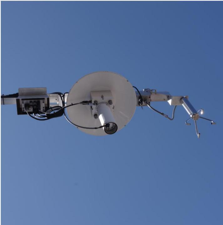
**Figure 11.** The 2D Sonic Anemometer mounted with other instruments on a TIS Tower mid-level boom.
