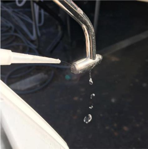
**Step 4.** If there is accumulated dirt on the transducer cap, gently spray some distilled or DI water on to the transducer cap and let it drain off.
