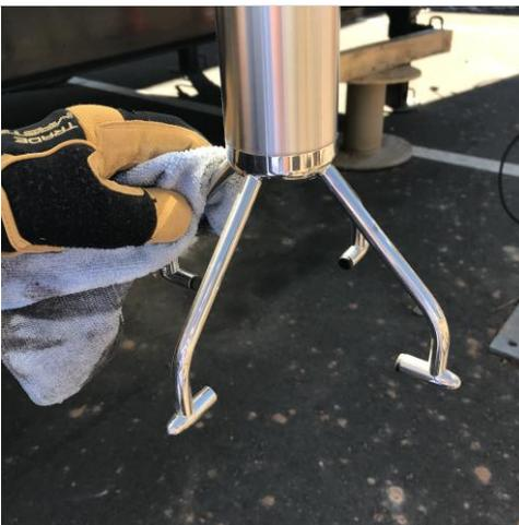
**Step 3.** Gently wipe down and clean the stainless steel portions of the spars and transducers. Avoid applying pressure to the spars that may cause a misalignment.
