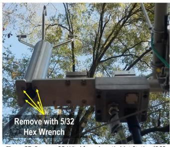
**Figure 27.** Remove 2D Wind from Aquatic Met Station (D03 FLNT).
