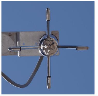
**Figure 2.** Picture of the 2D Anemometer showing the configuration of the opposing pairs of transducers.
