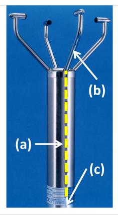
**Figure 4.** Identifying the "North" or Reference spar on Non-Heated and Heated 2D Sonic Anemometers.
