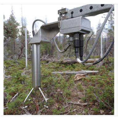
**Figure 9.** TIS Tower mounted 2D Sonic Anemometer with associated Junction Box on ML1.
