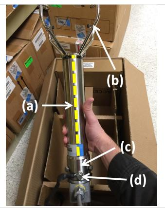
**Figure 6.** Identifying the "North" or Reference spar on Extreme-Heated 2D Sonic Anemometers.
