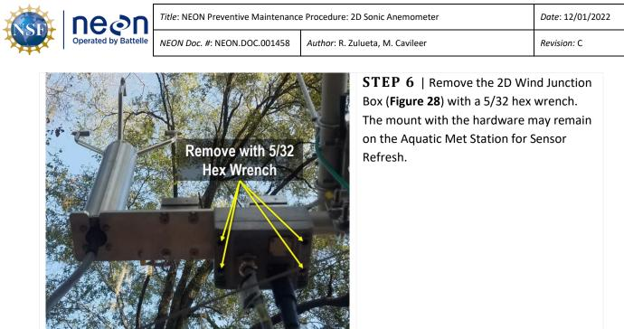
Figure 28. Remove Junction Box (D03 FLNT).
