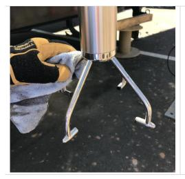
**Step 3.** Gently wipe down and clean the stainless steel portions of the spars and transducers. Avoid applying pressure to the spars that may cause a misalignment.
