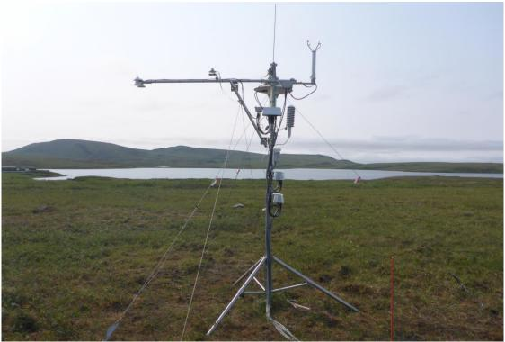
Figure 23. AIS Aquatic Met Station Radiation Boom Arm - Short End with the 2D Sonic Anemometer (D18 TOOK).
