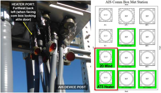
Figure 35. AIS Device Post: Comm Box Heater Ports for Aspirated Temperature Shield (ATS) and 2D Wind (Source: AD [10]).
