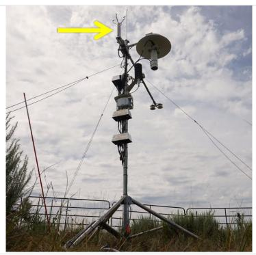
**Figure 14.** AIS Met Station Mounted 2D Sonic Anemometer.
