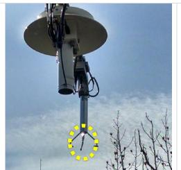
**Step 6.** Do a closer inspection of each spar of each 2D Sonic Anemometer for any more subtle misalignments of the spars.
