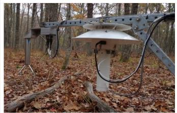
Figure 17. ML1 Profile Temperature Sensor Boom (D07 MLBS).
