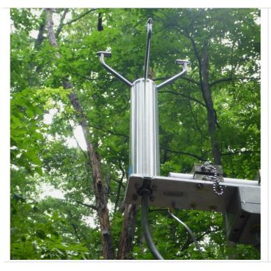
**Figure 13.** Close-up picture of an AIS Met Station mounted 2D Sonic Anemometer.
