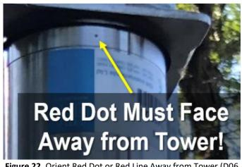
**STEP 7.1** | Orient the 2D Wind sensor where the red dot (or red line) on the sensor body faces away from the tower (**Figure 22**).
