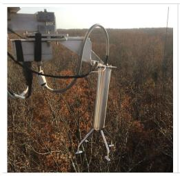
**Step 2.** Do a closer inspection of each 2D Sonic Anemometer mount for more subtle misalignments, bent mounts, or damage.
