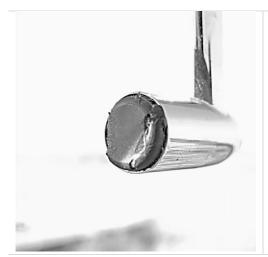
**Step 1.** Visually inspect each face of the transducers for any damage to the black transducer caps.
