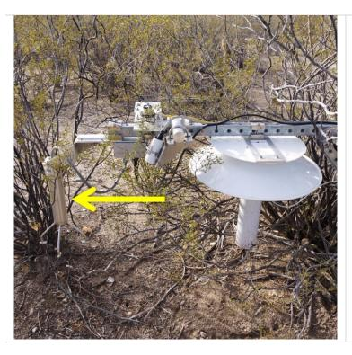
**Figure 12.** The 2D Sonic Anemometer shield mounted along with other instruments on TIS Tower Measurement Level (ML) 1.
