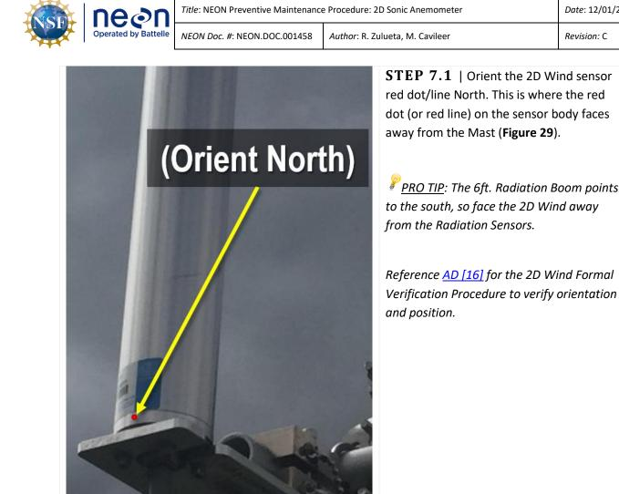
Figure 29. Orient Red Dot or Line North (D09 PRPO).
