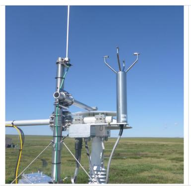
**Figure 10.** AIS Met Station mounted 2D Sonic Anemometer.
