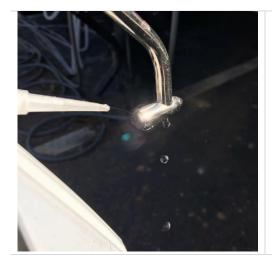
**Step 6.** Rinse once more with distilled or DI water and allow to air dry
