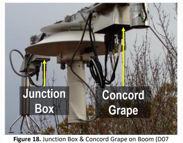
**STEP 3** | The 2D wind sensor shares a Concord Grape (24V) with the AATs sensor (**Figure 18**). Disconnect Eth-to-Comm (RJF) and sensor connections from the Concord Grape (24V) per AD [09].
