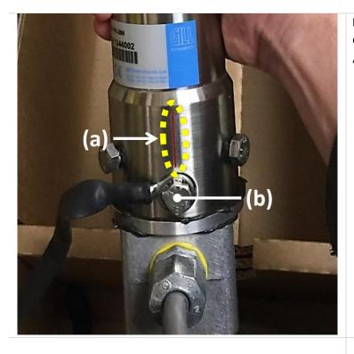
**Figure 5.** Close-up view of the Red Alignment Line and M8 Grounding Bolt on Extreme-Heated 2D Sonic Anemometers.
