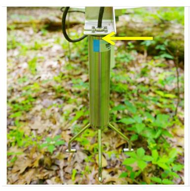
**Figure 8.** TIS Tower mounted 2D Sonic Anemometer indicating the position of the Red Alignment Dot (arrow).
