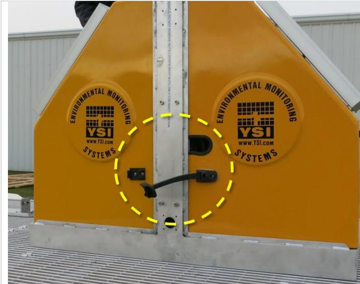
Figure 19. Unlatch to Remove Fiberglass T-Frame Covers (D09 PRPO).
