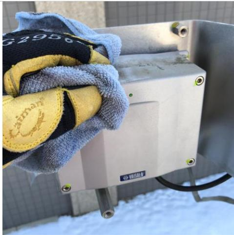
**Step 5.** Using a multi-surface cleaner and a lint-free cloth or microfiber towel, clean the outside of the Barometric Pressure Sensor.
