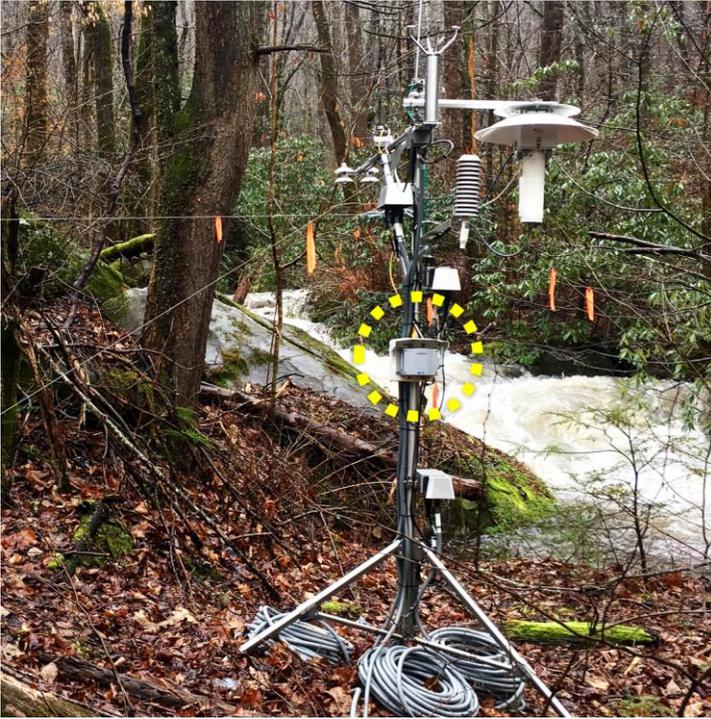
**Figure 7.** Barometric Pressure Sensor with rain shield, which mounts to the tripod mast on the Aquatic Met Station. Grape subsystem mounts to the mast as well under a sun/rain shield.
