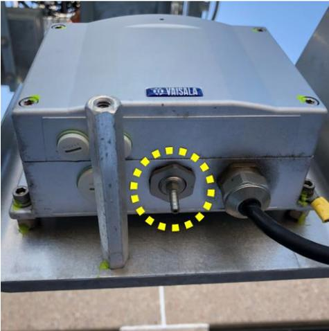
**Step 1.** Visually inspect the  $\frac{1}{8}$ " Pressure Inlet Port for any debris or blockage.
