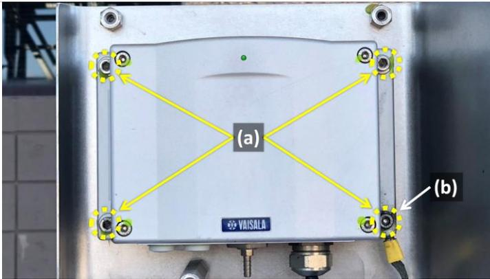
Figure 11. Remove Sensor (D13 NIWO).
