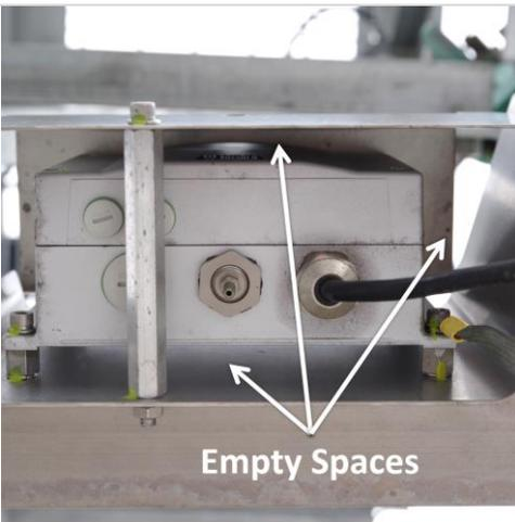
**Step 3.** (TIS Only) Visually inspect the space between the sun shields and the sensor enclosure for any debris or insect nests.
