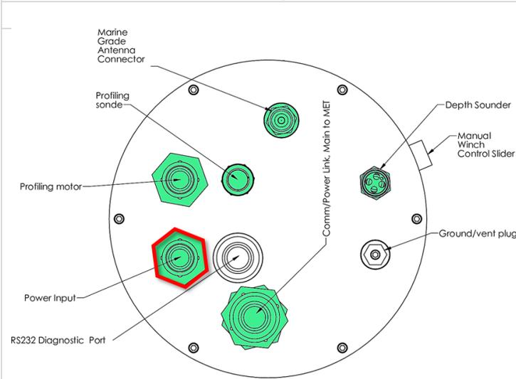
Figure 20. Profile Canister Port Mapping (Source: AD [10]).
