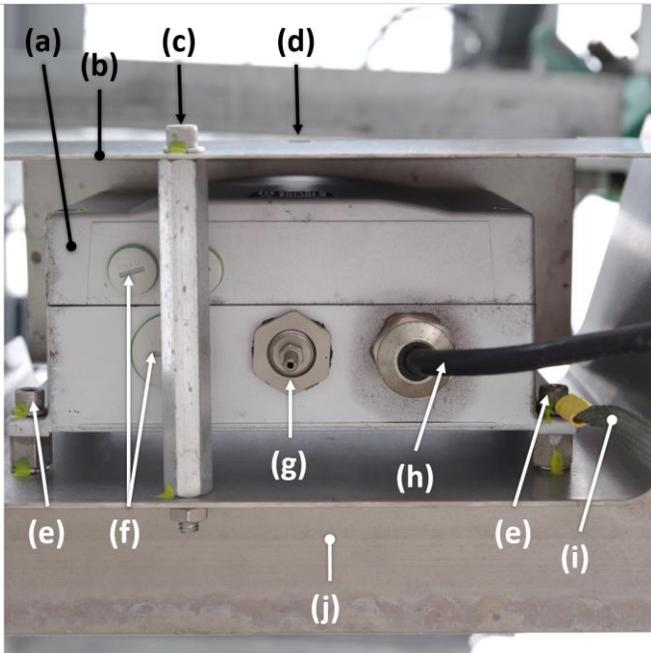
**Figure 4.** Underside view of a TIS tower mounted Barometric Pressure Sensor.
