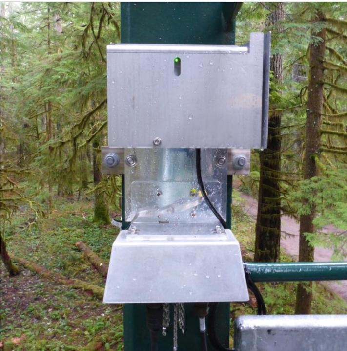
**Figure 6.** Barometric Pressure Sensor with both sun shields and subsystem mount for its Grape, which mount together to the Wind River Tower leg.
