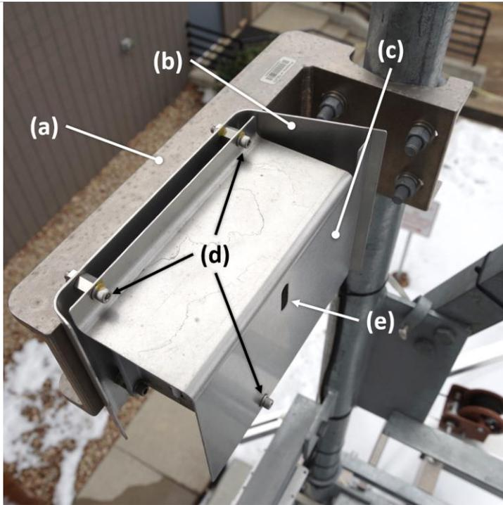
**Figure 3.** The Barometric Pressure Sensor with sun shields mounted on the TIS tower.
