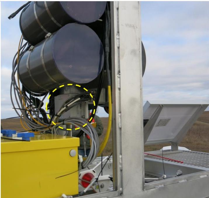
**Figure 8.** For AIS Buoy lake/river sites, the Barometric Pressure sensor mounts on the T-Frame under the Met and Profile PVC Canisters. (Yellow fiberglass covers protect these components when the AIS Buoy is on the lake/river.)
