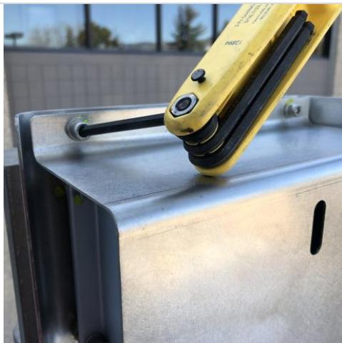
**Step 6.** (TIS Only) Replace the sun shield and tighten the screws.
