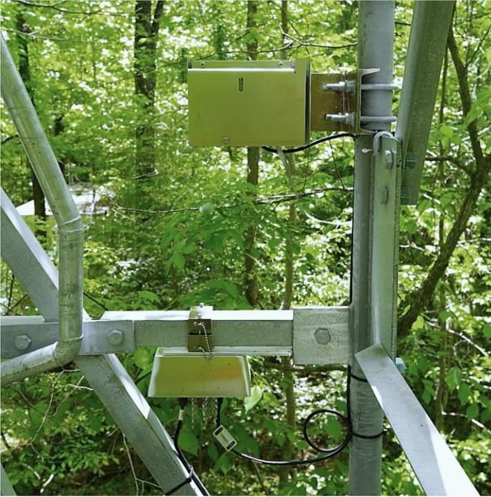
**Figure 5.** TIS Tower mounted Barometric Pressure Sensor with both Sun Shields and tower leg U-bolt mount, and Concord Grape subsystem with railing mount.
