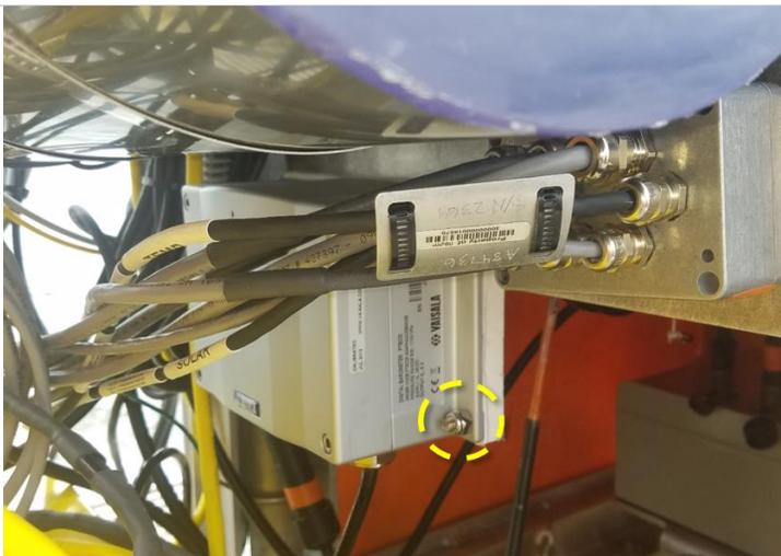
Figure 22. Remove Sensor via Mounting Hardware.
