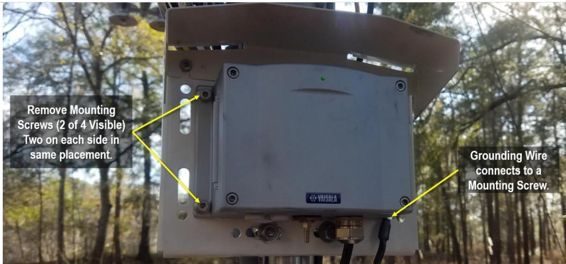
**Figure 14.** Remove the 4 Screws Securing the Sensor to the Mounting Plate on the Aquatic Met Station (D03 FLNT).
