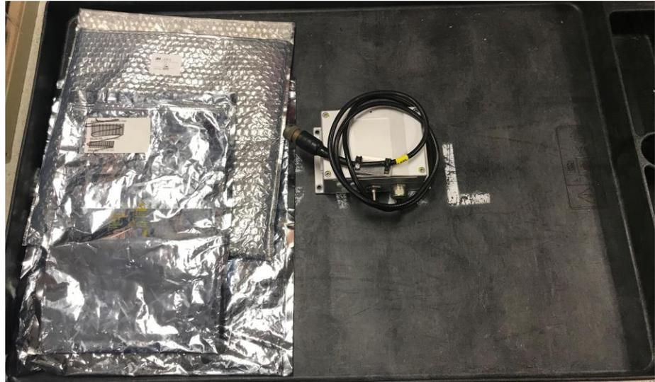
**Figure 25.** Use ESD Packaging to Return Sensor to CVAL Post-Decontamination.
