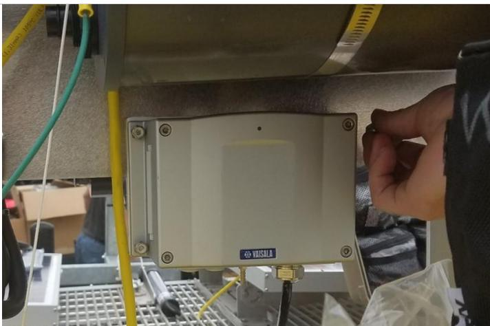
**Figure 24.** Reinstall Sensor on AIS Buoy (D09 PRLA).
