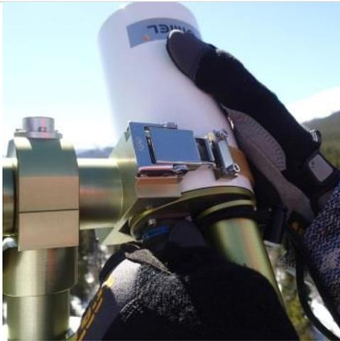
**Step 19.** Remove or slide the tool lanyard down the collimator and reconnect the sensor head cable to the sensor head. The MIL Spec connector should ‘click’ in place when fully secured.
