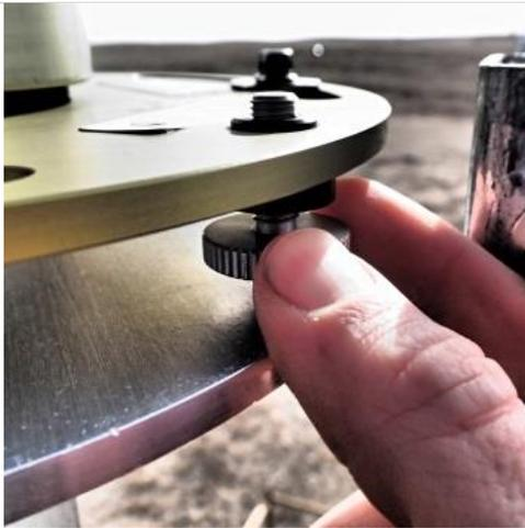
**Step 3.** Adjust the two thumbscrews up or down on the base until level.
