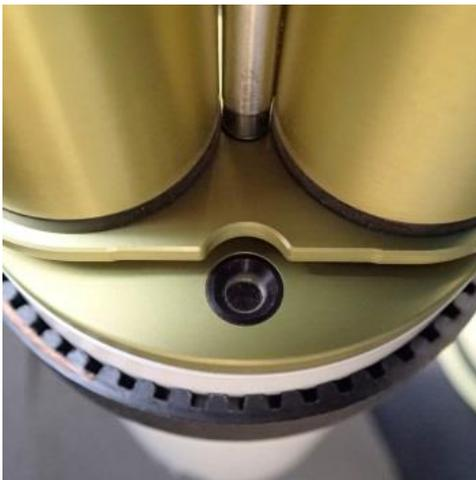
**Step 2.** When attaching the collimator, the other side of the collimator should also align along the outside of the four quadrant light sensor. See also **Table 2** for additional alignment information.
