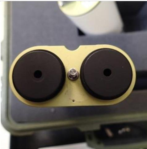
**Step 2.** Hold collimator so the end that attaches to the sensor body is facing you. Inspect the rubber gaskets for cracks or tears, particularly around the two center apertures. Cracks and tears will cause additional stray light to leak through to the detectors.
