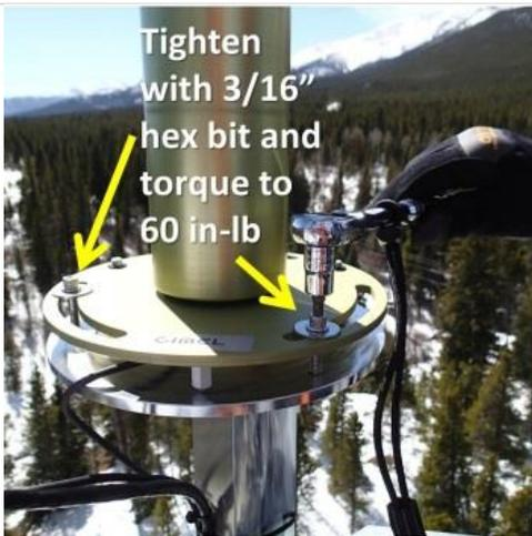
**Step 4.** Once level, tighten down the three socket head screws with a 3/16" hex bit, and torque to 60 in-lb.
