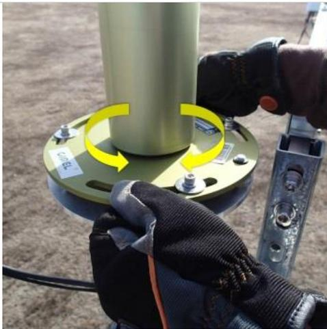
**Step 2.** Rotate the base and observe the direction the sun spot moves when rotated.
