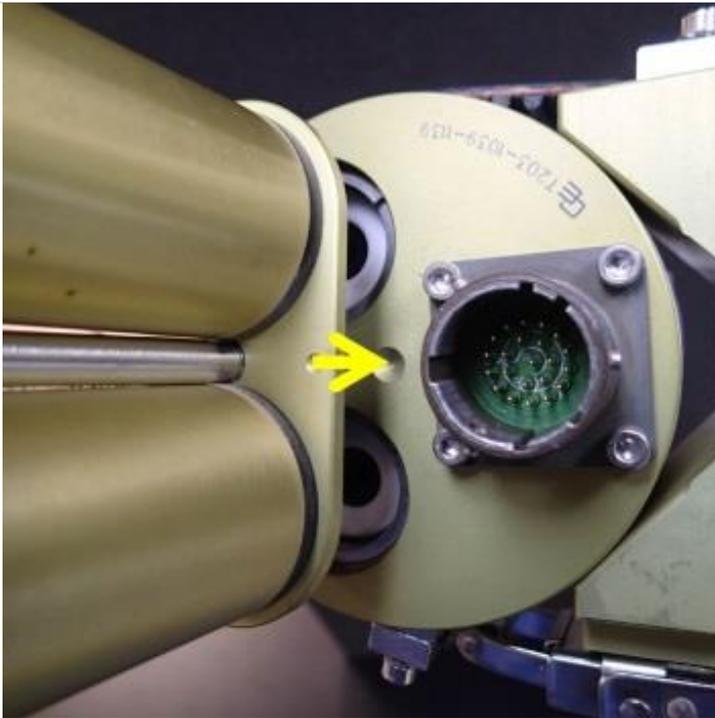
**Figure 15.** When attaching the collimator to the sensor body, match the alignment hole on the collimator to the hole in the sensor body (yellow arrow).
