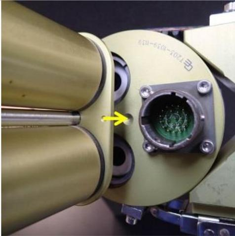
**Step 1.** Gently grab hold of the sensor body and carefully match the alignment hole with that on the sensor body. When attaching the collimator, orient it properly by aligning the notch on the collimator base and the sensor body.
