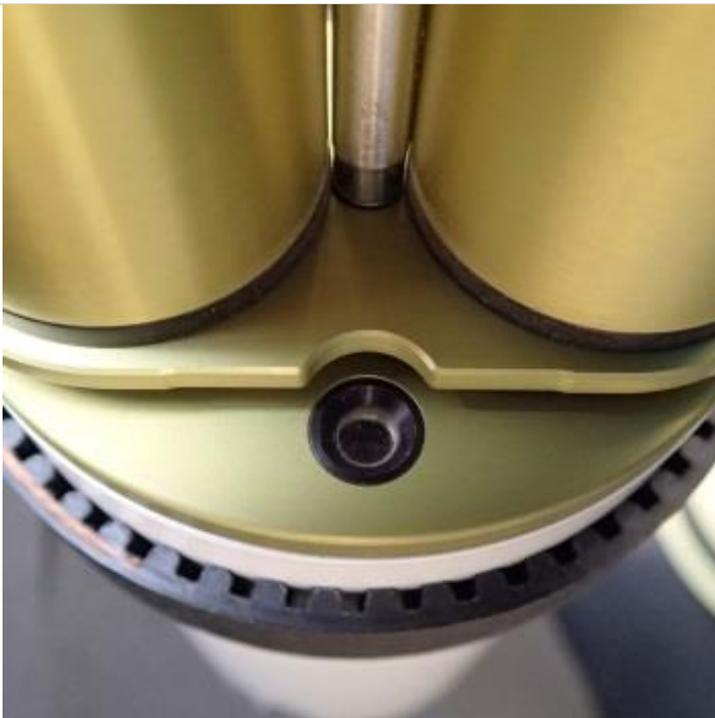
**Figure 16.** The half-circular notch on the collimator should align along the edge of the four quadrant detector, if properly aligned and installed.
