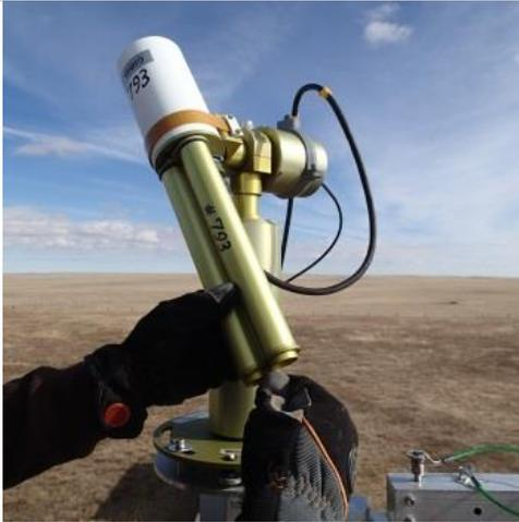
**Step 4.** While holding the collimator, loosen the screw knob the remaining way with your fingers.
