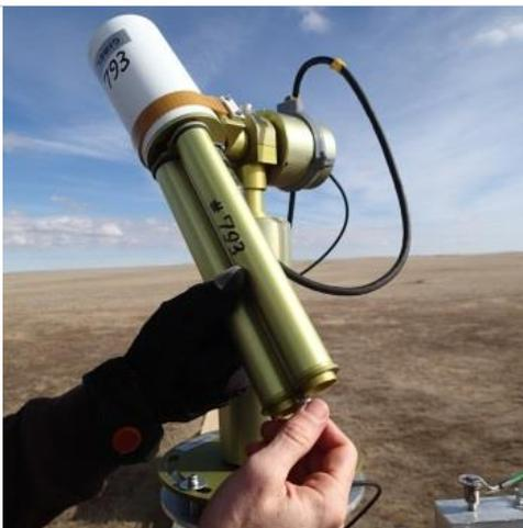
**Step 3.** Hold the collimator in place and finger tighten
