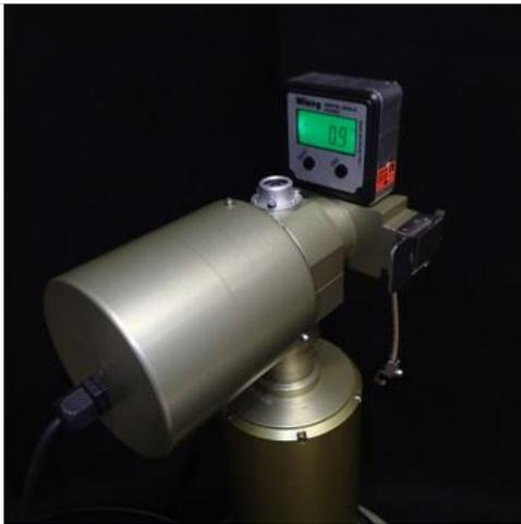
**Step 11.** Place an electronic level on the claw and check if it is level.
