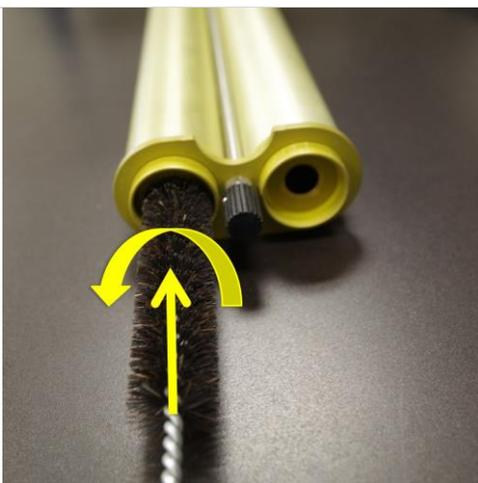
**Step 6.** Insert the specified brush into the open end of the collimator and slowly move it through the column with a counter-clockwise twisting motion until the end of the brush hits the end of the collimator.
