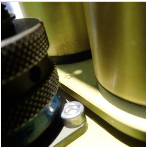
**Step 3.** Rotate the base as needed until the sun spot is horizontally aligned with the alignment target.
