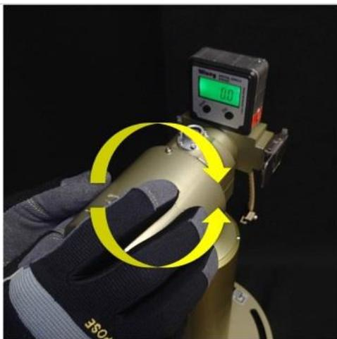
**Step 12.** To level the claw, hold the zenith motor and rotate along the motor's axis until the claw is level.
