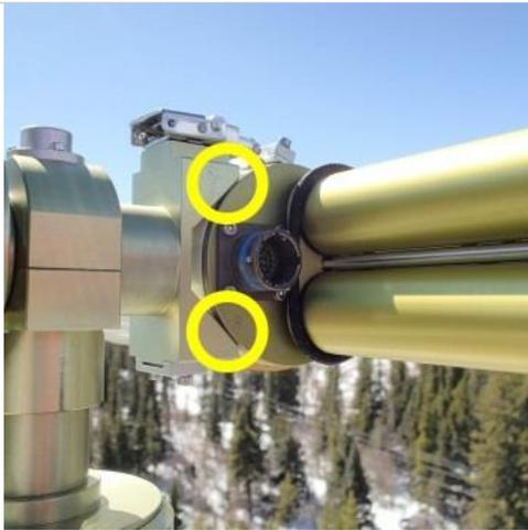
**Step 16.** Re-install the sensor head, and secure the strap. Remember the sensor head will be pointing downward.
