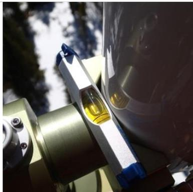
**Step 4.** Place a small 3" precision spirit level at the top part of the claw and check level.
