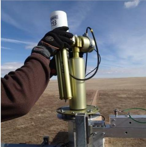
**Step 1.** Gently grab hold of the sensor body and slowly rotate the body so the collimator is approximately 45° from vertical.
