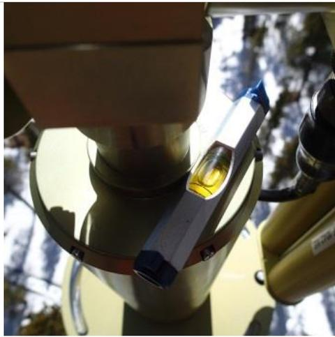
**Step 2.** Place a small precision spirit level at the top of the vertical motor cylinder.
