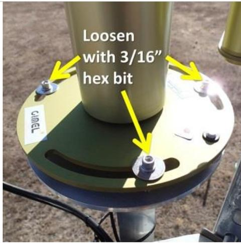
**Step 1.** Loosen the three socket head screws with a 3/16" hex bit.
