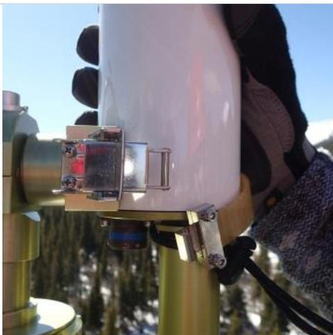
**Step 7.** Gently remove the sensor head and place in a secure location away from the elements, and in an area where it will not get damaged.
