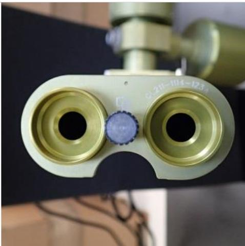
**Step 5.** Turn the collimator over so the open end is facing you.
