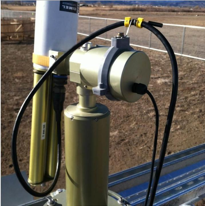
**Figure 6.** Example of the cable routing for the sensor head cable. This routing should allow for full range motion of the robot.
