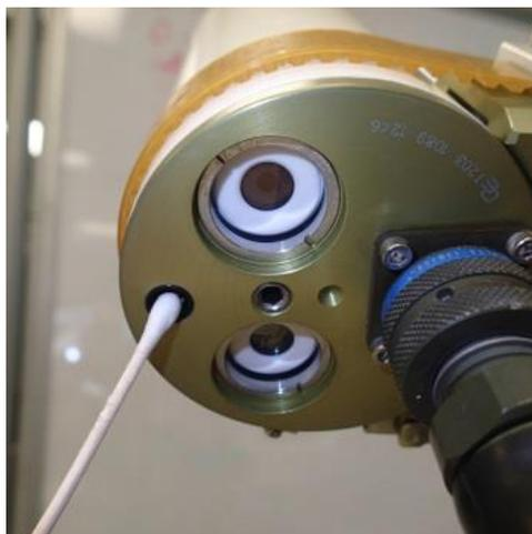
**Step 2.** Dampen a clean cotton swab with distilled or DI water and gently wipe clean the four quadrant detector window. Dry the detector with a dry cotton swab, lint free cloth, or Kimwipe.
