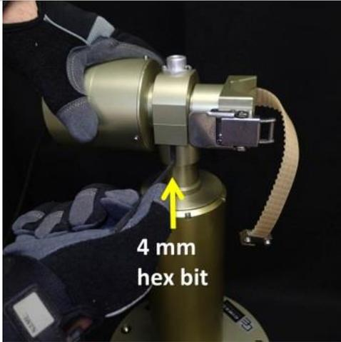
**Step 8.** Hold the zenith motor and with a 4 mm hex bit, loosen the screw  $\frac{1}{4}$  turn.
