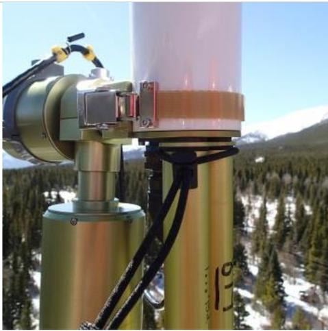
**Step 2.** Attach a large tool lanyard to the collimator as shown to secure it from falling to the ground.
