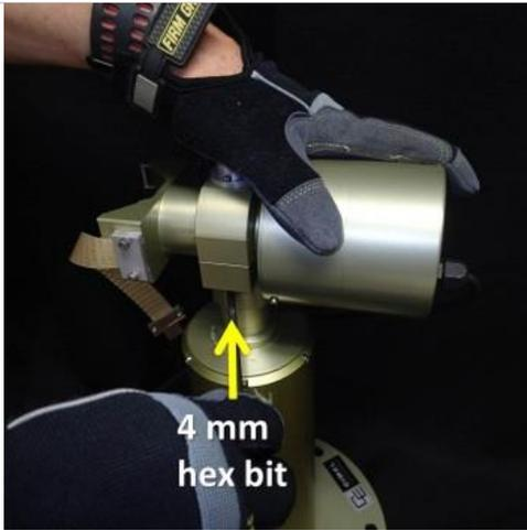
**Step 10.** Hold the zenith motor and with a 4 mm hex bit, loosen the screw  $\frac{1}{4}$  turn.
