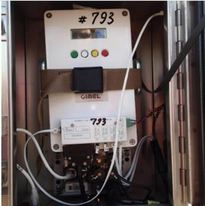
**Figure 18.** The Cimel control box within the enclosure.
