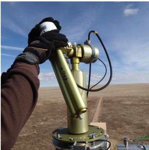
**Step 2.** The sensor body and collimator should be rotated so it is about a 45° angle from vertical, or enough to clear the mounting base or other tower support.
