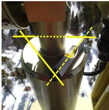
**Step 3.** Place a small precision spirit level at the top of the vertical motor cylinder. Check the level along three horizontal planes as shown to the left.
