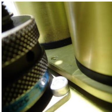
**Step 6.** A sun image will shine through the pinhole at the top end of the collimator and onto the base of the collimator (by the sensor head cable connector).
