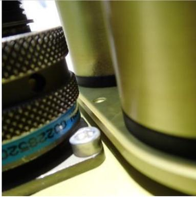
**Step 7.** If perfectly aligned, the sun image should overlap with the alignment hole at the base of the collimator (left).
