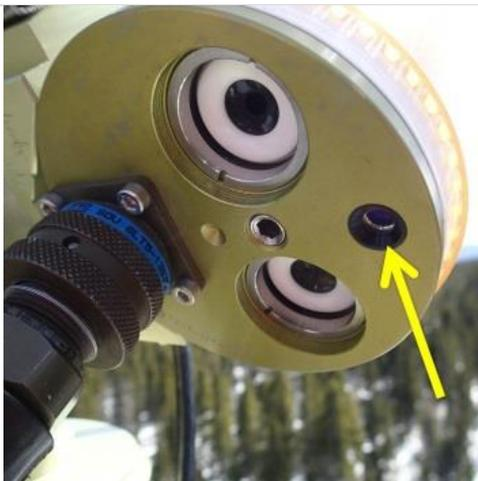
**Step 1.** Visually inspect the four quadrant detector for dust, dirt, or spider webs.
