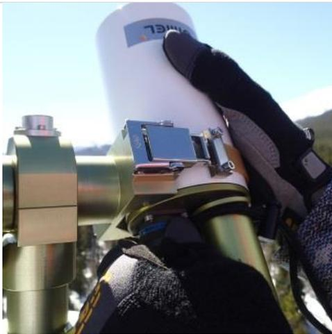
**Step 3.** Hold the sensor body and disconnect the sensor head cable from the sensor body. You may have to slightly rotate the sensor head to allow for easier removal of the connector. Once removed, you can let the sensor head cable dangle out of the way as it should still be attached to the cable holder on the robot. The sensor head cable connector is a MIL Spec twist connector.
