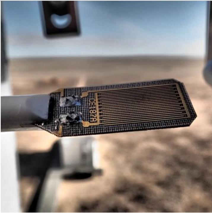
**Figure 4.** Close up view of the wet sensor.
