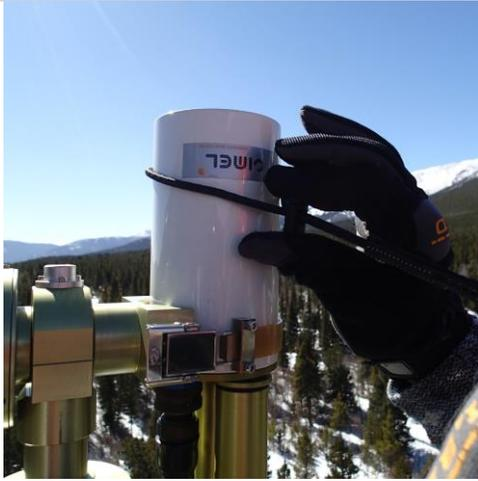
**Step 2.** Attach a large tool lanyard to the sensor body as shown to secure it from falling to the ground.
