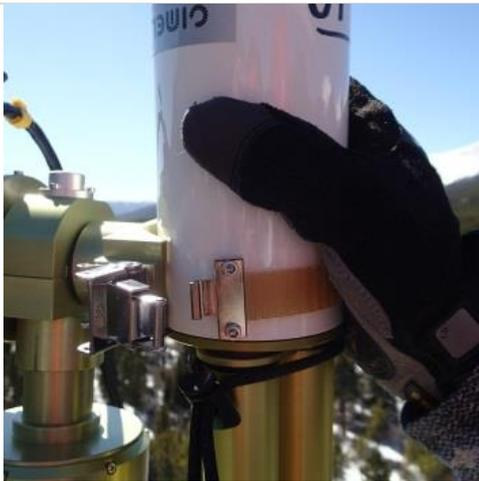
**Step 6.** While holding the sensor body, release the clasp that attaches the strap to the buckle.
