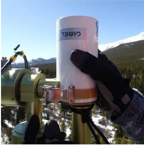
**Step 4.** Hold the sensor body and unbuckle the strap that holds the sensor body to the claw.
