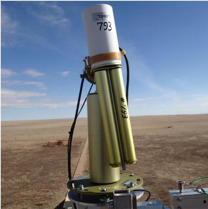
**Figure 9.** The sensor head when it is in Automatic Mode and parked. Notice that it is pointed downward, but slightly off center from vertical by a few degrees.
