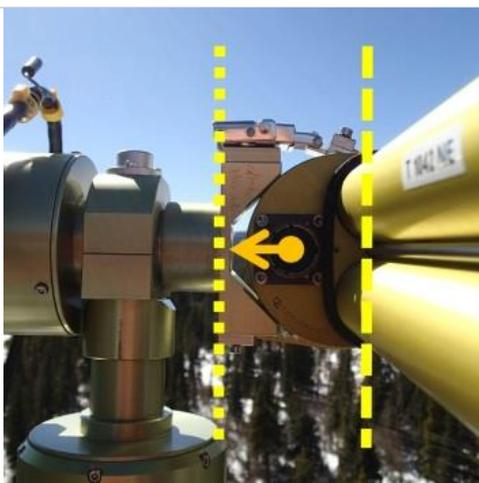
**Step 18.** Align the sensor with respect to the back edge of the claw. The collimator should be parallel with the back edge of the claw.
