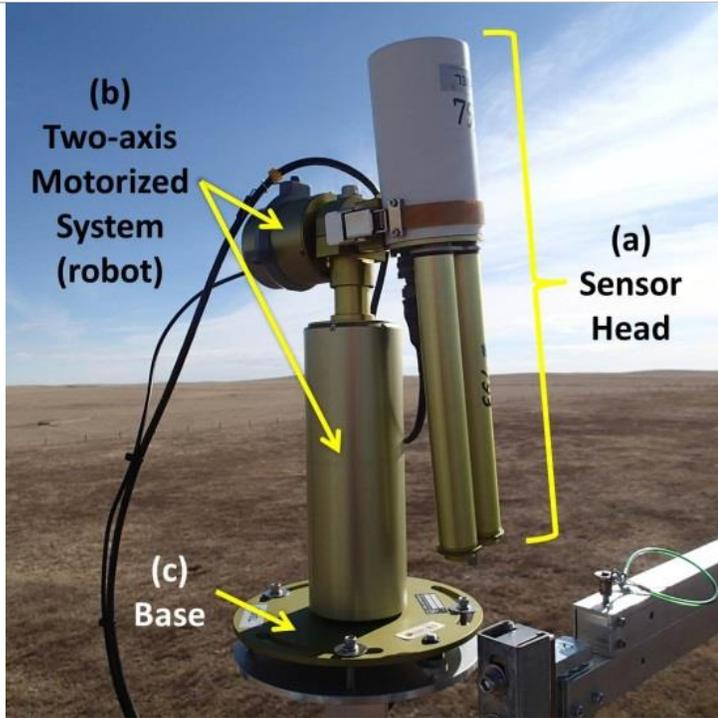
**Figure 1.** The main components of the Cimel CE318N includes the following:
