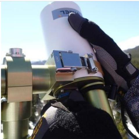
**Step 3.** Hold the sensor body and disconnect the sensor head cable from the sensor body.
