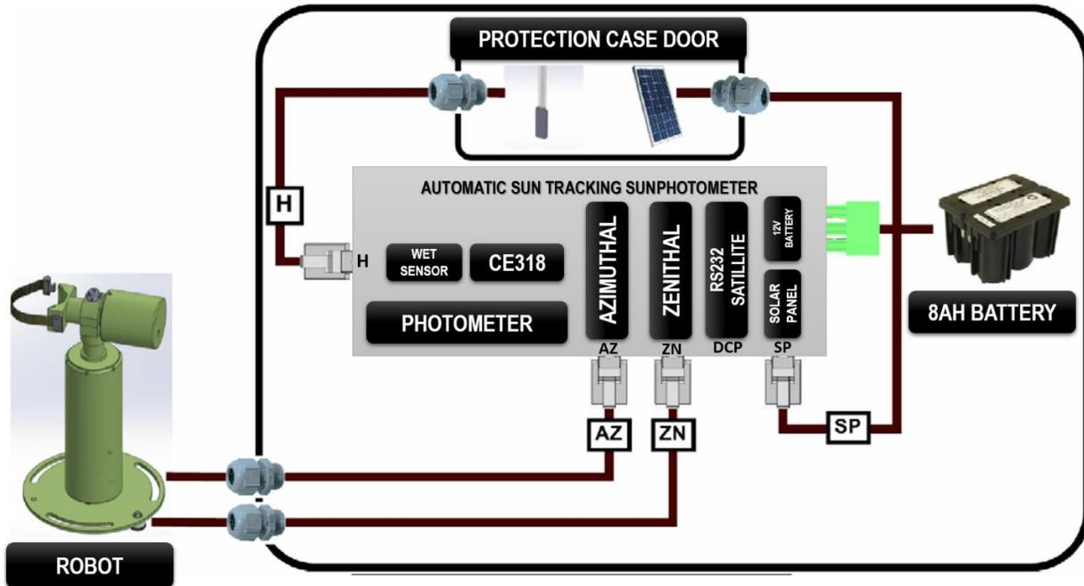
**Figure 26.** Disconnect all the wires connected to the Control Box when removing the robot from the tower top.
