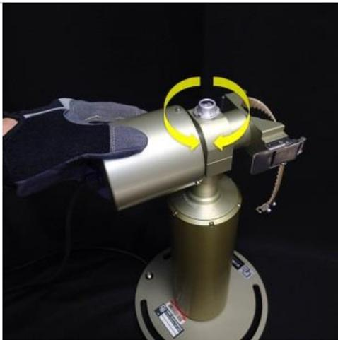
**Step 9.** Holding the zenith motor, rotate the motor and claw  $180^\circ$  to access other side.
