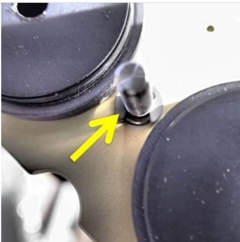
**Step 3.** Check to see that there is a metal clip still attached to the end of the threaded screw end.
