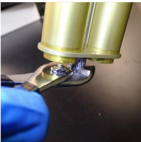
**Step 3.** Hold steady the collimator, and use a pair of pliers to initially loosen the screw knob at the end of the collimator if cannot be loosened by hand.
