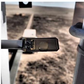
**Step 8.** Wet the sensor with water and observe whether the HH status changes to ‘1’ within a minute.
