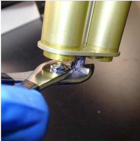
**Step 4.** Once the screw knob is finger tight, hold the collimator while using a pair of pliers and tighten an additional ¼ turn.
