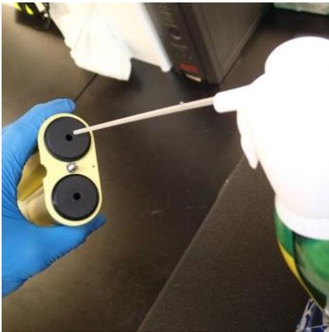
**Step 9.** Follow with two more short blasts of air through each collimator side.
