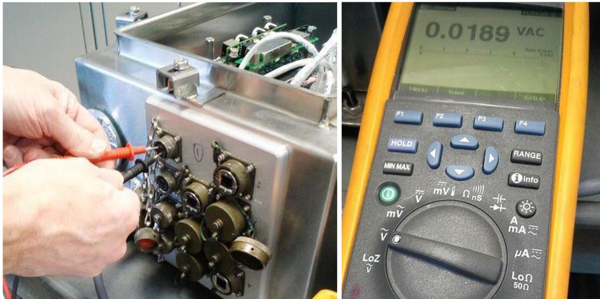
Figure 23. Verifying shut down procedures via the communications box heater port.
