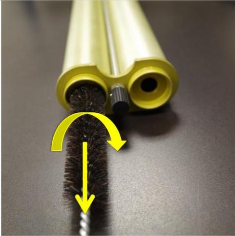
**Step 7.** Once the brush hits the end of the collimator, slowly remove the brush by pulling it through the column with a clockwise twisting motion until completely removed.
