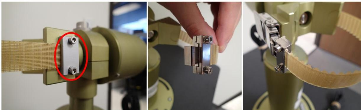
**Figure 27.** Photos for strap replacement and removal.
