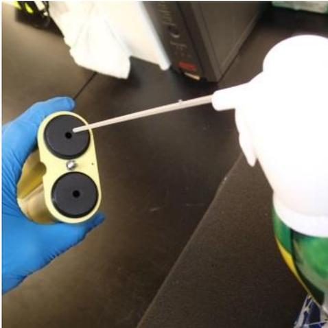
**Step 4.** Insert the tube from a compressed air canister and apply two short blasts of air. This will help quickly loosen any dust or spider webs.
