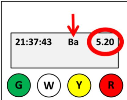
**Step 5.** The **Ba** indicates that you are monitoring the internal battery. In the example, the battery voltage is 5.20 V.
