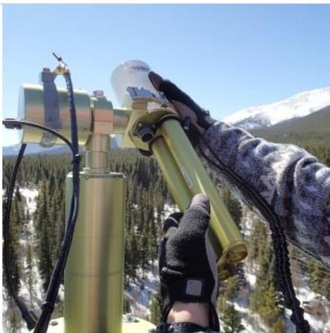
**Step 17.** Gently rotate the sensor head so it is horizontal and the collimator is facing towards you.
