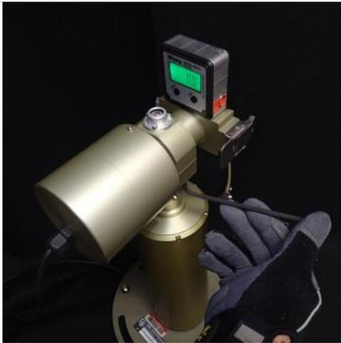
**Step 13.** Re-tighten box hex screws with a 4 mm hex bit.
