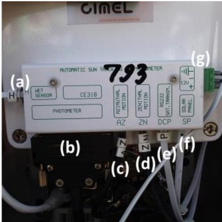
**Figure 21.** Connector panel on the control box. Inputs includes connectors for the:
