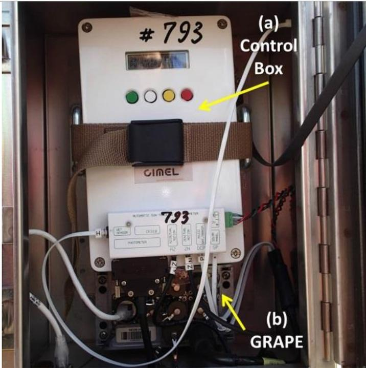
**Figure 2.** The (a) Cimel control box as mounted within the enclosure. It is mounted above its associated (b) GRAPE.
