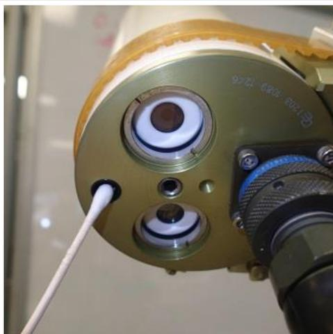
**Step 3.** Dampen a clean cotton swab with 95% ethanol and gently wipe clean the four quadrant detector window. Dry the detector with a dry cotton swab, lint free cloth, or Kimwipe.
