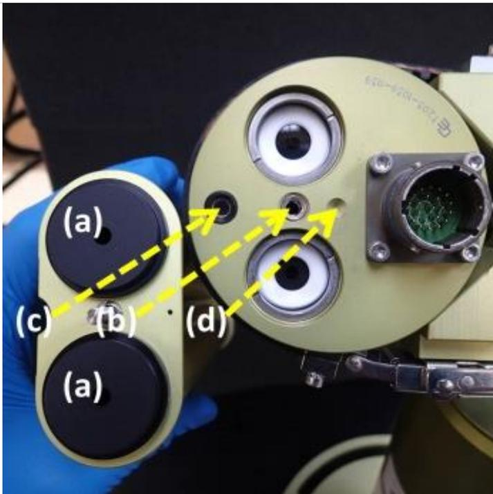
**Figure 14.** Alignment of the collimator is a matter of matching the (b) threaded screw to the sensor body, the (c) half-circular notch around the four quadrant sensor, and the (d) sun spot alignment hole. The collimator will only properly align in one orientation.
