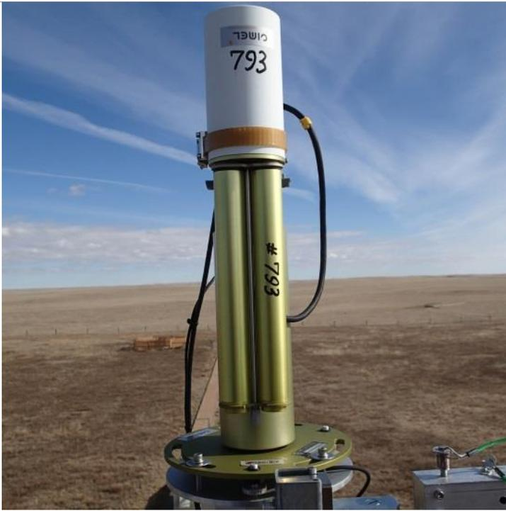
**Figure 10.** The sensor head when it is in Manual Mode, and manually parked. Notice that it is pointed downward and vertical.
