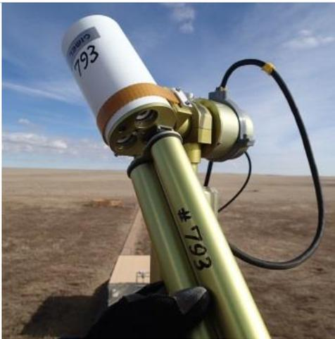
**Step 5.** Once the collimator is loose, pull the collimator free along the same angle that the sensor body is already positioned.
