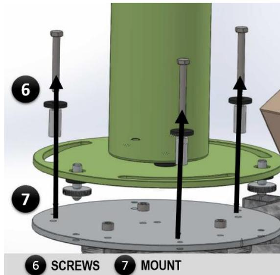
**Figure 25.** Screws to remove for removing the robot from the tower top.
