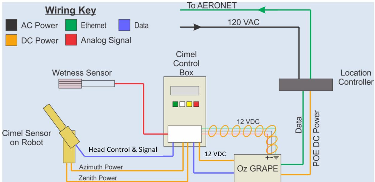
Figure 22. Electrical schematic for the Cimel.
