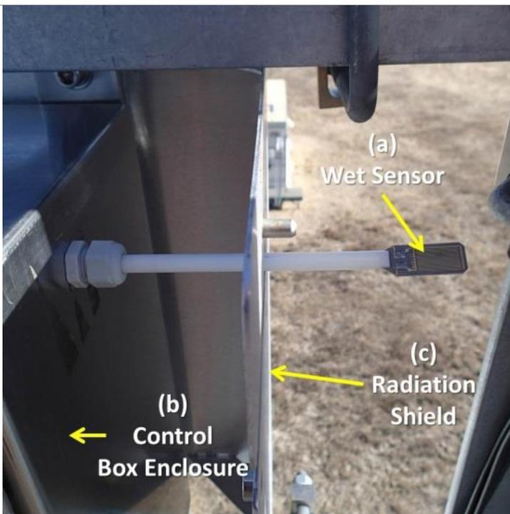
**Figure 3.** The Cimel (a) wet sensor is typically attached to the side of the Cimel (b) control box environmental enclosure, and through the (c) enclosure radiation shield.
